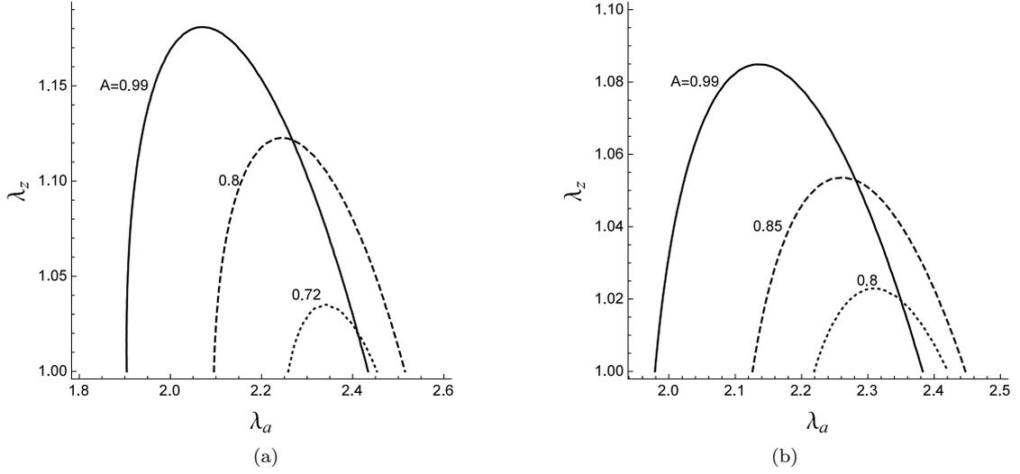
**Fig. 4** Effects of finite thickness/bending stiffness for two different values of  $k_1$  while  $J_s$  and  $\phi$  are fixed to be 30 and  $30^\circ$ , respectively. (a):  $k_1 = 1/15$ ; (b):  $k_1 = 1/10$ . It is seen that the stronger the fibre-reinforcement, the earlier the bifurcation curve disappears as  $A$  is decreased.
