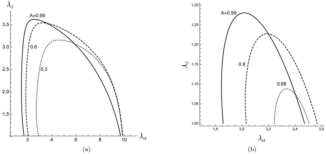
**Fig. 3** Plot of  $\Omega(\lambda_a, \lambda_z) = 0$  for three representative values of  $A$ . (a): Without fibre-reinforcement; (b): with fibre-reinforcement ( $k_1 = 1/20$ ,  $J_f = 30$ ,  $\phi = 30^\circ$ ). It shows the fact that with fibre-reinforcement the bifurcation curve moves down quickly as  $A$  is decreased and the curve disappears completely at a threshold value of  $A$ .
