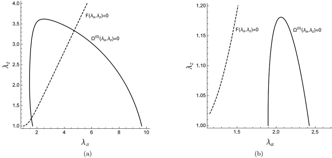
**Fig. 2** The contour plots of  $\Omega^{(0)}(\lambda_a, \lambda_z) = 0$  and  $F(\lambda_a, \lambda_z) = 0$  under the membrane assumption. (a):  $k_1 = 0$ ; (b):  $k_1 = 1/15$ ,  $J_f = 30$ ,  $\phi = 30^\circ$ . They show the fact that without fibre-reinforcement localized bulging is possible if either the axial stretch or the axial force is fixed, but with fibre-reinforcement localized bulging is only possible if the axial stretch is fixed to be less than 1.18.
