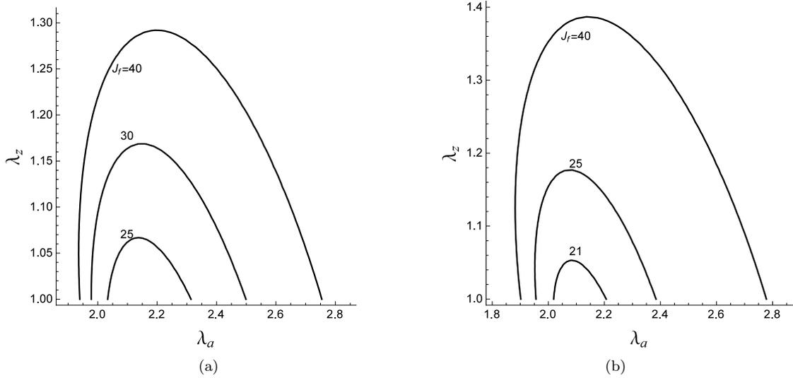
**Fig. 5** Effects of fibre extensibility (characterized by  $J_f$ ) with  $A = 0.9$  and  $\phi = 30^\circ$  fixed. (a): Solution of  $\Omega(\lambda_a, \lambda_z) = 0$  with  $k_1 = 1/15$ ; (b): solution of  $\Omega(\lambda_a, \lambda_z) = 0$  with  $k_1 = 1/20$ .
