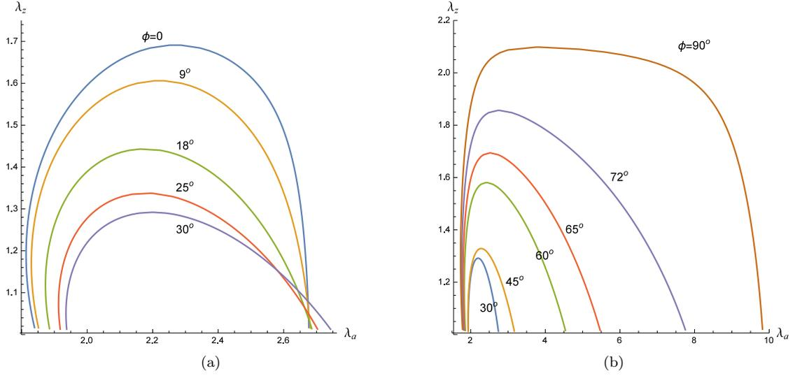
**Fig. 6** Effects of fibre orientation  $\phi$  with  $A = 0.9$ ,  $k_1 = 1/15$  and  $J_f = 40$  fixed. All the curves are the solutions of  $\Omega(\lambda_a, \lambda_z) = 0$  for the values of  $\phi$  indicated.
