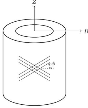
**Fig. 1** Geometry of a helically fibre-reinforced cylindrical tube
