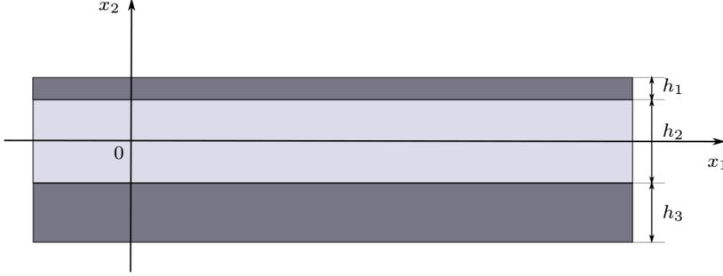
Fig. 1: A three-layered asymmetric plate
