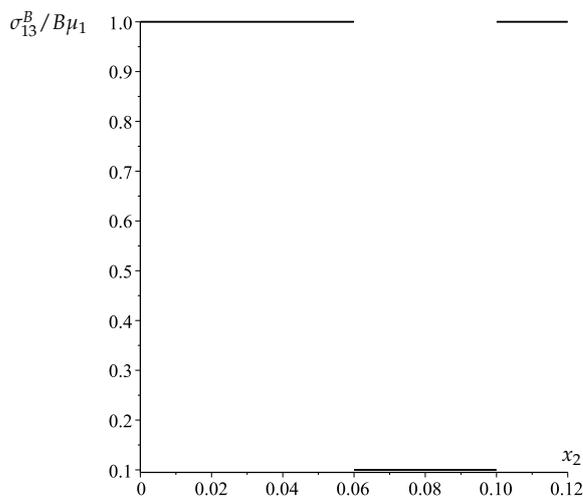
Figure 5. Scaled stress variation (33) across the width of a semi-strip.
