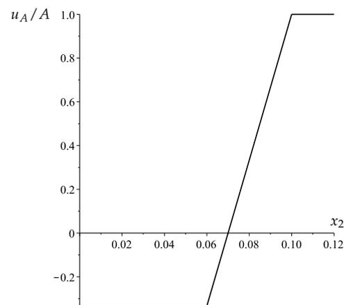
**Figure 2.** Dimensionless displacement variation (30) across the width of a semi-strip.
