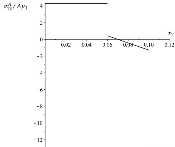
Figure 4. Scaled stress variation (32) across the width of a semi-strip.
