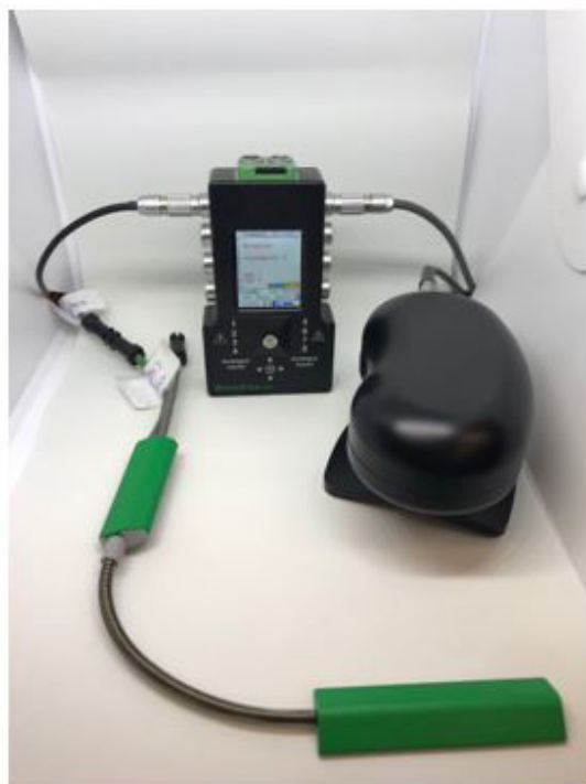
Figure 1a: Twin Axis Electronic Goniometer (front left). Electronic Myometer (front right). DataLOG (back centre) used to gather data
