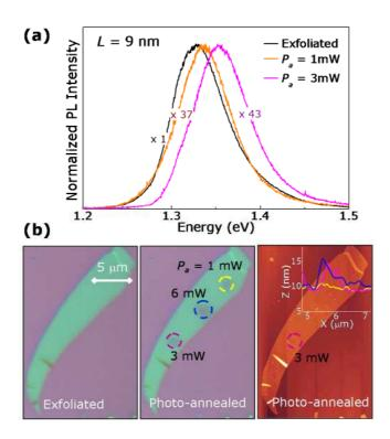
**Figure 2** (a) Room temperature PL spectra of an InSe flake before and after laser exposure at different powers,  $P_a$ . (b) Optical image of the flake before (left) and after (right) laser exposure at powers  $P_a = 1$  mW, 3 mW and 6 mW ( $\lambda_a = 532$  nm,  $t_a = 30$  mins). The circles indicate the laser-exposed areas of the flake. The image on the right is an AFM image of the flake after the laser exposure. The inset shows the AFM z-profiles of a laser-exposed areas.
