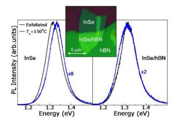
**Figure 6.** (a) Room temperature normalized PL spectra of p-InSe flakes with and without encapsulation by hBN (P = 0.1 mW and  $\lambda = 633$  nm). Spectra were measured before (black line) and following (blue line) thermal annealing steps at increasing temperatures  $T_a$  up to 150 °C. The inset is an optical image showing the regions of the flake with and without the hBN film.
