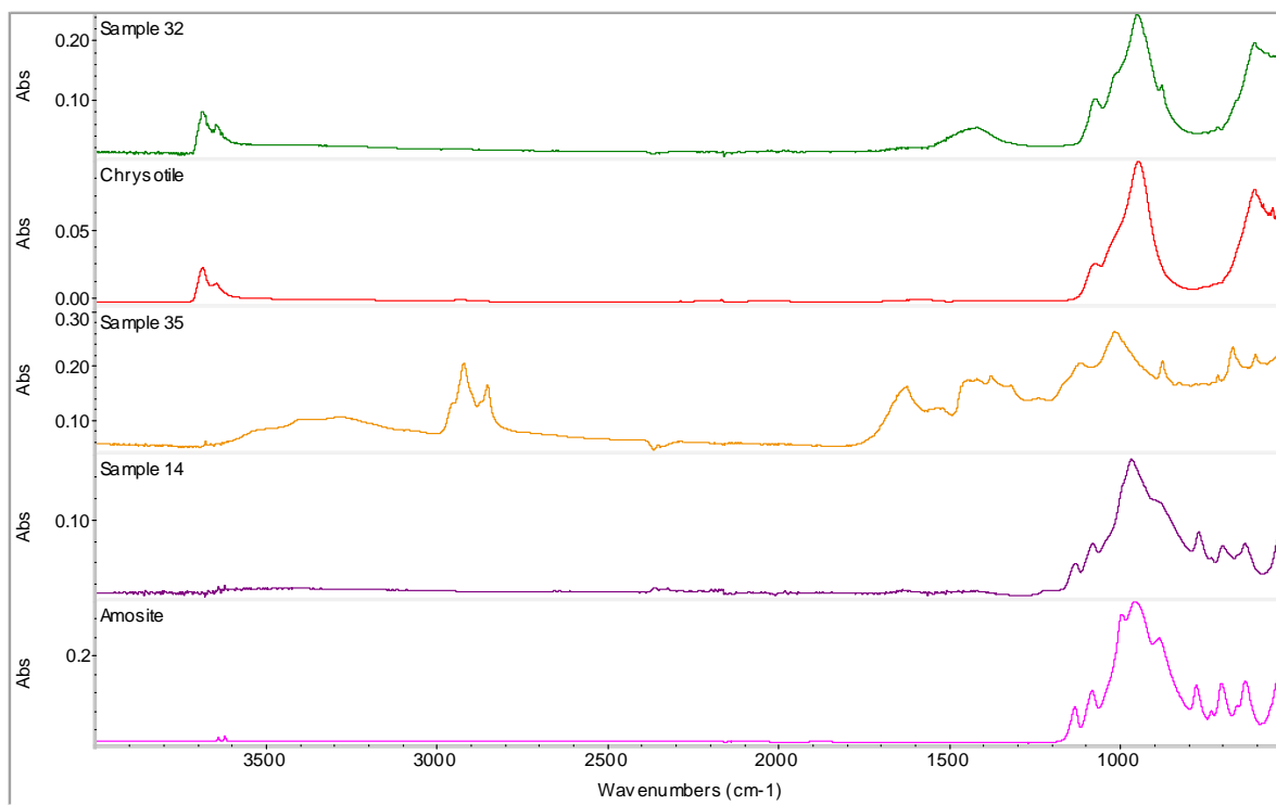
Figure S4. FTIR spectra of samples 32, 35 and 14, along with reference chrysotile and amosite.
