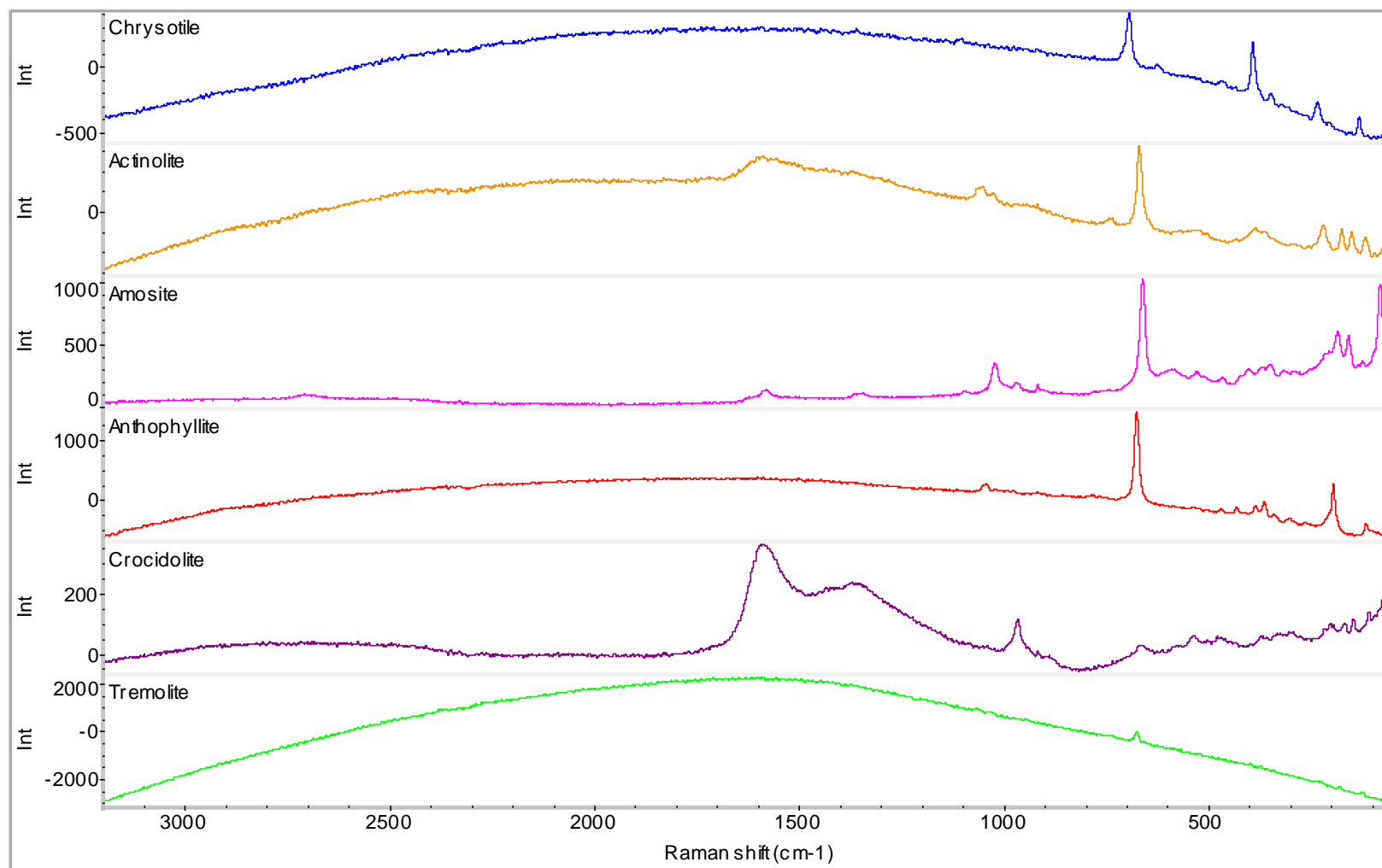
Figure S7a. Raman spectra of asbestos reference samples collected using 532 nm excitation wavelength.
