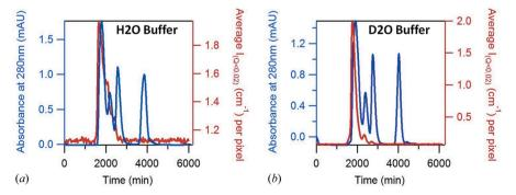
Figure 2 SEC-SANS measurements of SEC calibration standards eluted with 0% (a) and 100% (b) D<sub>2</sub>O buffer. The absorbance of the sample at 280 nm is plotted in blue, and the averaged SANS intensity between  $Q = 0.007 \text{ Å}^{-1}$  and  $Q = 0.02 \text{ Å}^{-1}$  is in red. The column (Superdex 75) efficiently separates proteins of molecular weight (MW) from 3000 to 70000 Da.
