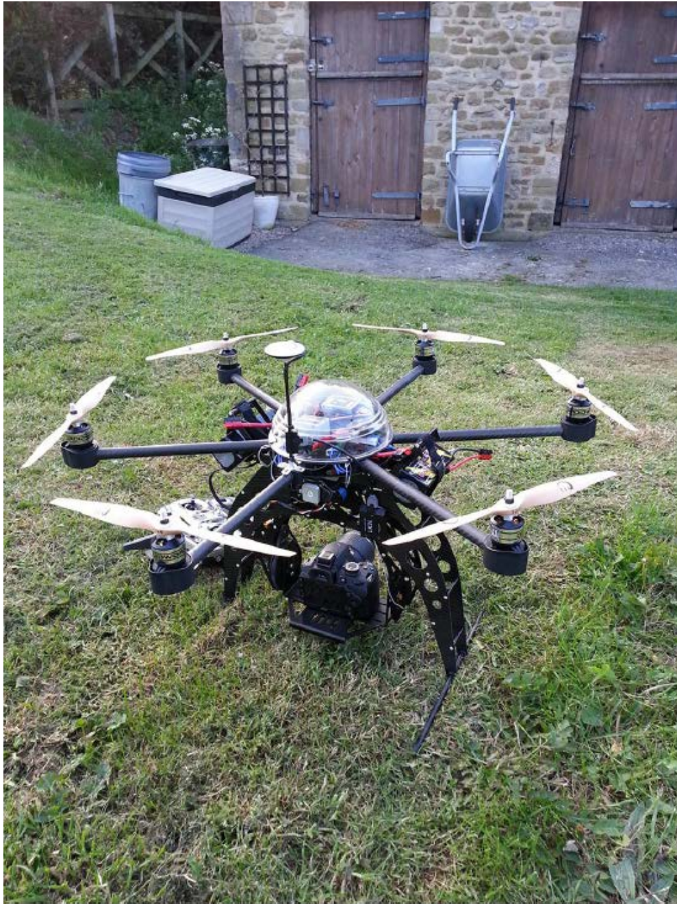
Fig. 3. A camera-mounted hexacopter for orthogonal to vertical, oblique and orthogonal to ground imagery. A standard 16 megapixel digital camera is shown but any payload up to 1 kilogram can be deployed (see text for discussion).
