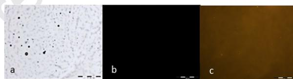
Figure 4. Bright field (a) and fluorescence images (b) and (c) of nano-particles fabricated from the copolymer dissolved in THF and diethyl glycol. Fluorescence photographs were obtained using 510 nm emission and 470 - 495 nm excitation filters with 1000 ms (b) and 15000 ms (c) exposure time. All images were captured under 40 x magnification.
