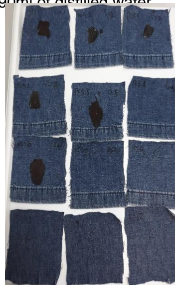
Figure 4 - Blood stained and control preliminary cotton samples before they were washed (own image).
