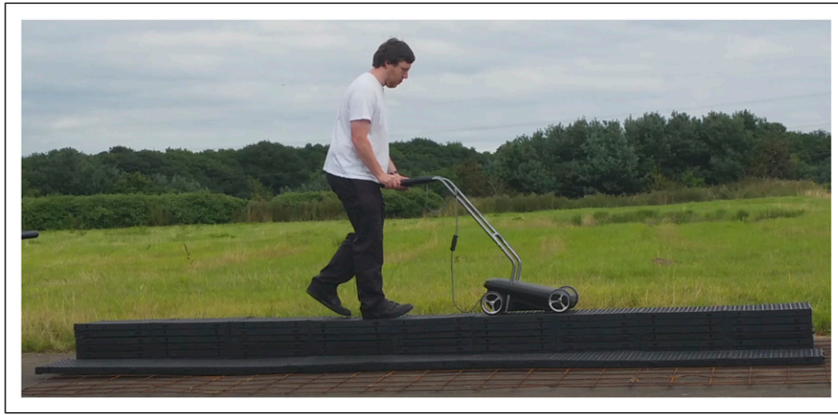
Figure 4. An EMAD scan being carried out with a simulated cover depth of 251 mm.
