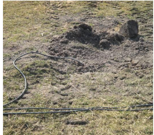
Figure 8 Left: Shallow burial of CMG-5U accelerometer in horizontal position. Bedded level with sand. Right: CMG-5U in place in the ground covered with soil.
