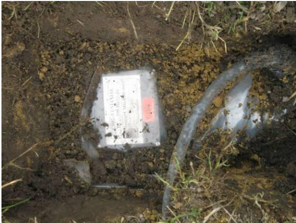
Figure 8 Left: Shallow burial of CMG-5U accelerometer in horizontal position. Bedded level with sand. Right: CMG-5U in place in the ground covered with soil.
