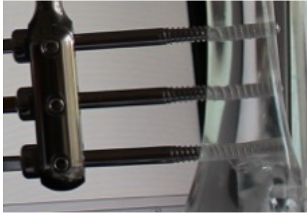
Fig 2 – An Illustration of the Half-Pin Providing Mono-Lateral Location
