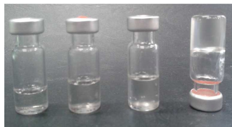
Figure 3. Concentrated aqueous solutions of 9:Na ; from left to right: 1, 2, 2.5 and 3 g/mL.
