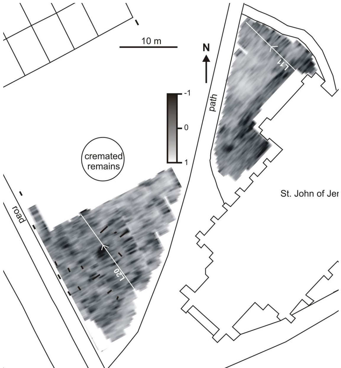
Fig. 18. Mapview of combined 225/450 MHz GPR absolute amplitude 9-35 ns time-depth slices with background map.
