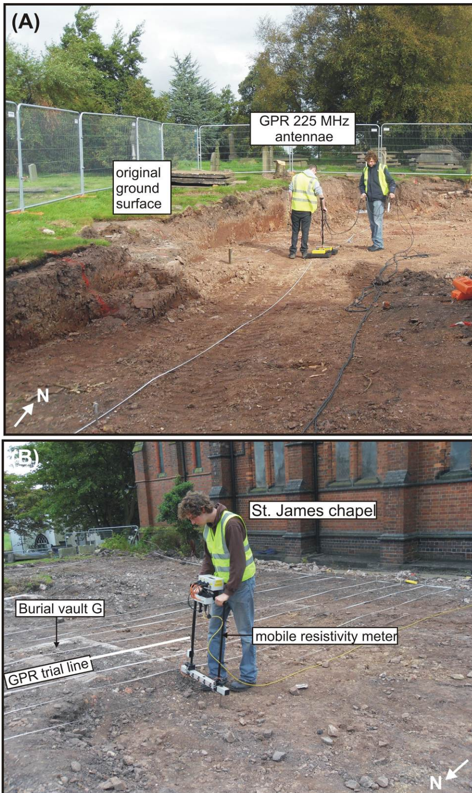
Fig. 2. Photographs of case study 1 site, also showing (A) 225 MHz dominant frequency GPR and (B) bulk ground resistivity (0.5 m fixed-offset) data being collected. Note trial 2D GPR L1043 profile position over burial vault (Fig. 3b) marked in (B).
