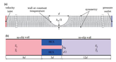
**Figure 45.** Geometry of the HEX used for CDF simulations. (a) Circular HEX tube. (from Figure 3 in Surendran et al.<sup>90</sup>) and (b) Rectangular HEX tube (after Figure 2 in Strobio Chen et al.<sup>91</sup>).
