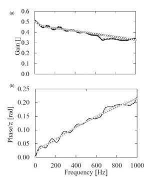
**Figure 52.** HEX transfer functions with average velocities taken at 2 mm ( $\cdots$ ), 25 mm(- - - -), and 42 mm (-) from the flame tip. The no-burner case is shown by markers (°). (a) Gain and (b) Phase (from Figure 11 in Hosseini et al. <sup>94</sup>).
