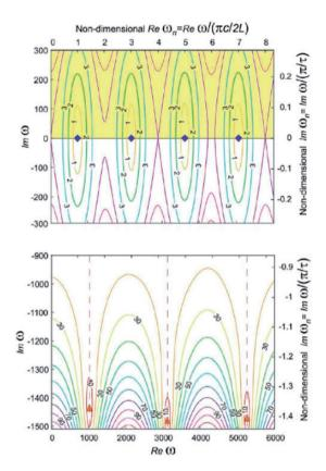
**Figure 23.** Contour plot of  $|f(\omega)|$  in the complex frequency plane for  $\tilde{n}=0.025$ ,  $\tau=3$  ms. The two sections are parts of the same plot. Yellow shading indicates instability (from Figure 3 in Mukherjee and Shrira<sup>45</sup>).
