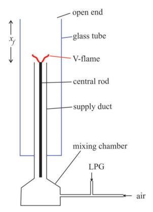
**Figure 1.** Schematic illustration of the laminar premixed ducted V-flame (after Figure I (a) in Mukherjee et al.<sup>8</sup>).
