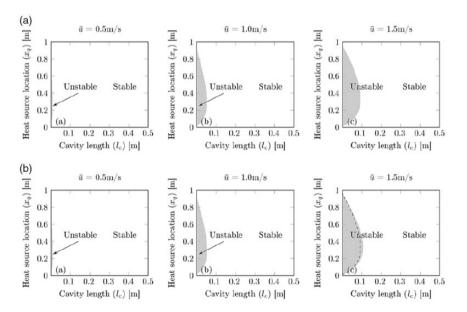
**Figure 57.** Stability maps in the  $I_c - x_q$  parameter plane for three different inlet velocities  $\bar{u}$ . (a) HEX modelled as oscillating heat sink and as acoustic scatterer (from Figure 14 in Surendran et al.<sup>93</sup>). (b) HEX modelled as oscillating heat sink only (from Figure 15 in Surendran et al.<sup>93</sup>). The dashed line in the right sub-figure of (b) marks the stability boundary of the sub-figure above it.
