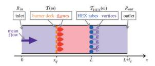
**Figure 38.** Schematic of idealised quasi-ID configuration for modelling purposes.
