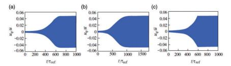
**Figure 16.** Time evolution of the acoustic velocity for nonlinear heat release laws. (a) Van der Pol polynomial with  $n_0=1$ ,  $n_1=-10$ ,  $n_2=-3\times 10^8$ . (b) Levine-Baum heat release law with  $n_0=1$ ,  $n_1=-17.3$  and (c) Capped linear heat release rate with  $q_{max}=0.007\bar{Q}/(S\bar{\rho}\bar{u})$  (after Figures 3, 5, 7 in Crespo Anadón et al. 38).
