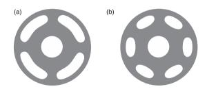
**Figure 5.** Flow restrictors acting as turbulence generators. (a) 75% blockage ratio and (b) 85% blockade ratio (after Figure I (c,d) in George et al. <sup>14</sup>).
