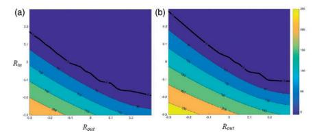
**Figure 55.** Stability map obtained from network model in the  $R_{out} - R_{in}$  parameter plane. (a) Single row of HEX tubes (from Figure 5.3 in Strobio Chen<sup>63</sup>) and (b) Double row of HEX tubes (from Figure 5.4 in Strobio Chen<sup>63</sup>). Positive growth rates indicate instability.
