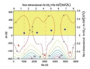
**Figure 24.** Contour plot of  $|f(\omega)|$  in the complex frequency plane for  $\tilde{n}=$  I,  $\tau=$  3 ms. Yellow shading indicates instability (from Figure 4 in Mukherjee and Shrira<sup>45</sup>).
