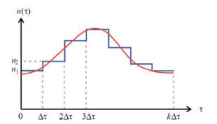
**Figure 10.** Coupling coefficient as a function of time-lag (red curve) and its piecewise approximation (blue curve; after Figure 2 in Gopinathan et al.<sup>25</sup>).
