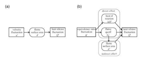
Figure 29. Processes generating fluctuations in heat release rate caused by (a) velocity fluctuations u', and (b) equivalence ratio fluctuations  $\phi'$  (after Figure 3 in Cho and Lieuwen<sup>52</sup>).
