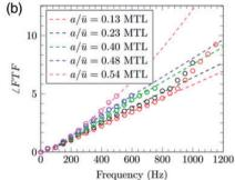
**Figure 11.** FDF of Noiray's matrix flame vs. frequency. Markers: measured values (after Figure 6 in Noiray et al.<sup>28</sup>). Dashed curves: Gopinathan's approximation based on (11) with linear fitting functions for  $n_1(a), \ldots n_k(a), \sigma_1(a), \ldots \sigma_k(a)$ , and quadratic fitting functions for  $\tau_1(a), \ldots \tau_k(a)$ . (a) Gain and (b) Phase (after Figure 3 in Gopinathan et al.<sup>27</sup>).
