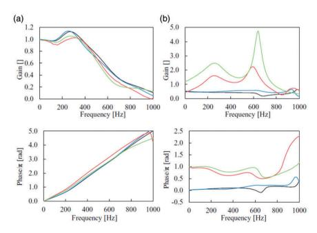
Figure 54. Gain and phase of the transfer functions for four burner-HEX distances: Y = 10 mm (—), Y = 8 mm (—), Y = 7 mm (—) and Y = 6 mm (—). (a) Transfer function of the burner and (b) Transfer function of the HEX (from Figures 13 and 14 in Hosseini et al. <sup>94</sup>).
