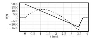
**Figure 34.** Overall impulse response. Solid line: uniform profile. Dashed line: parabolic profile (from Figure 4 in Albayrak and Polifke<sup>54</sup>).
