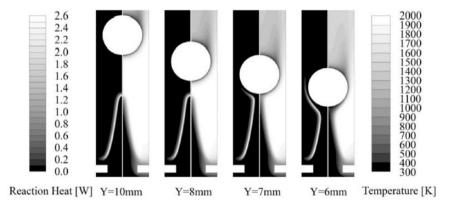
**Figure 53.** Thermodynamic fields for four burner-HEX distances: Y = 10, 8, 7 and 6 mm. Left side of each image: field of reaction heat. Right side of each image: temperature field (from Figure 12 in Hosseini et al.<sup>94</sup>).
