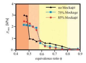
**Figure 6.** Bifurcation diagram showing the effect of equivalence ratio  $\phi$  on the rms pressure for three flow restrictors: no blockage (black curve), 75% blockage ratio (blue curve), and 85% blockage ratio (red curve; after Figure 3 in George et al. <sup>14</sup>).
