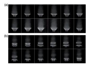
**Figure 2.** Flame dynamics over one period. (a) Low-amplitude limit cycle;  $x_f = 34 \, \text{cm}$  (from Figure 7 in Mukherjee et al.<sup>8</sup>) and (b) High-amplitude limit cycle;  $x_f = 45 \, \text{cm}$  (from Figure 9 in Mukherjee et al.<sup>8</sup>).
