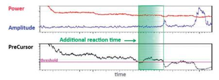
Figure 9. Performance of the IfTA precursor as early warning of an impending instability (after slide 28 in Rouwenhorst et al. 19).
