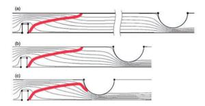
**Figure 49.** Flow streamlines (thin black curves) and flame shapes (thick red curves) for three successively decreasing burner-HEX distances. (a) Flow distorted by the burner/flame regains its ID profile upstream of the HEX; flame does not impinge. (b) Flow upstream of the HEX does not regain its ID profile; flame does not impinge and (c) Flow upstream of the HEX does not regain its ID profile; flame impinges on the HEX (after Figure 2 in Hosseini et al. 94).
