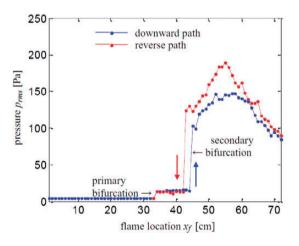
Figure 3. Bifurcation diagram showing the effect of flame location on the rms pressure (from slide 13 in Mukherjee<sup>11</sup>).
