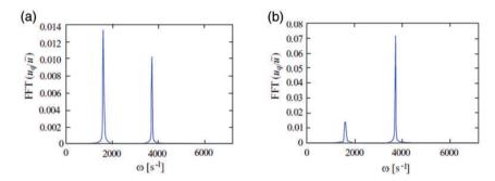
**Figure 20.** Fourier transform of the time history  $u_q(t)$  shown in Figure 5.5. (a) Time-window [0,1 s] and (b) Time-window [9 s, 10 s] (after Figure 6 in Bigongiari and Heckl<sup>41</sup>).
