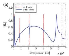
**Figure 42.** Reflection and transmission coefficient of a tube row with d = 0.017 m, h = 0.001 m,  $\eta = 0.0225$  m (from Figure 2.8 in Surendran<sup>82</sup>).
