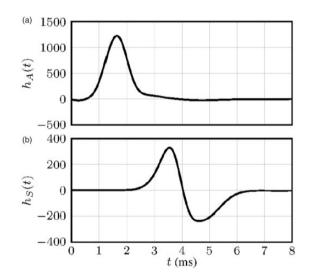
**Figure 32.** Impulse responses of the flame. (a) Response to the acoustic impulse (55) and (b) Response to the swirl impulse (56) (from Figure 7(c) in Albayrak et al.<sup>55</sup>).
