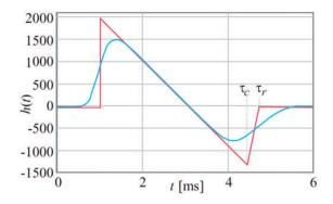
**Figure 33.** Impulse response combining the perturbations in  $\Delta H$ ,  $S_L$  and A. Red curve: without diffusion. Blue curve: with diffusion (after Figure 7 in Albayrak et al. <sup>56</sup>).
