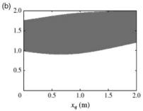
**Figure 17.** Stability maps depicting the dependence on the heat source position  $x_q$  of the amplitude  $a/\bar{u}$ . Stable regions are white; unstable regions are grey. (a) Rijke tube and (b) Quarter-wave resonator (from Figure 4 in Bigongiari and Heckl<sup>39</sup>).
