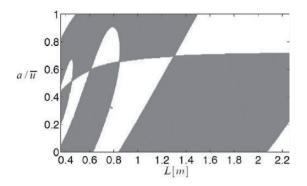
**Figure 22.** Stability map for the control parameter *L. Grey* areas are regions of instability; white areas are regions of stability (from Figure 3 in Bigongiari et al.<sup>30</sup>).
