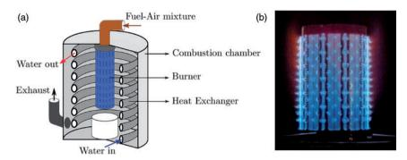
**Figure 37.** (a) Schematic of a domestic boiler with heat exchanger [Surendran<sup>74</sup>] and (b) Photograph of the burner with flames [Teerling<sup>75</sup>].
