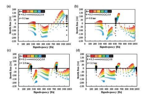
**Figure 25.** Eigenfrequencies and growth rates for all modes in the frequency window  $[0, ... 1000 \, \text{Hz}]$ . The temperature jump, expressed in terms of  $T_{21}$  (denoted by  $\theta$  in the figures) is scaled by marker size; the reflection coefficient R is scaled by colour. (a)  $\tau = 0.5 \, \text{ms}$ . (b)  $\tau = 0.8 \, \text{ms}$ . (c)  $\tau = 2.0 \, \text{ms}$  and (d)  $\tau = 2.5 \, \text{ms}$  (from Figures 5(b, c), 8(a, b) in Hosseini et al.<sup>47</sup>).
