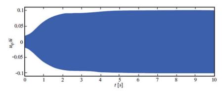
**Figure 19.** Time history of  $u_q(t)/\bar{u}$  in a Rijke tube with L=1.2m (after Figure 5 in Bigongiari and Heckl<sup>41</sup>).
