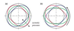
**Figure 8.** Waves in annular geometry. The pressure p' of mode 2 is shown at three successive time intervals  $t_1$ ,  $t_2$ ,  $t_3$ . (a) Standing wave and (b) Travelling wave (from slide 19 in Rouwenhorst et al.<sup>19</sup>).
