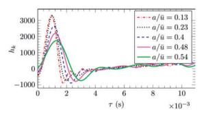
**Figure 12.** Impulse response corresponding to the measured FTFs shown in Figure 11 (after Figure 4 in Gopinathan et al.<sup>27</sup>).
