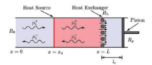
**Figure 56.** Schematic of the modelled combustion system (from Figure 1 in Surendran et al. <sup>90</sup>).
