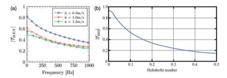
**Figure 46.** Numerical results for the gain of the HEX transfer function. (a) Results for the circular geometry in Figure 45(a) with d = 3 mm and  $h_g = 0.3$  mm (from Figure 4(a) in Surendran et al.<sup>90</sup>) and (b) Results for the rectangular geometry in Figure 45(b) with d = 12.8 mm and  $h_g = 0.8$  mm (after Figure 3(a) in Strobio Chen et al.<sup>91</sup>).
