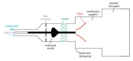
Figure 4. Schematic illustration of the turbulent swirl combustor (not to scale; after Figure 1(a,b) in George et al. 14).
