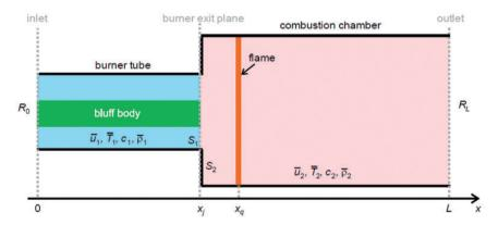
Figure 21. Idealised version of the BRS test rig shown in Figure 4.4 (from Figure 2 in Bigongiari et al.<sup>30</sup>).
