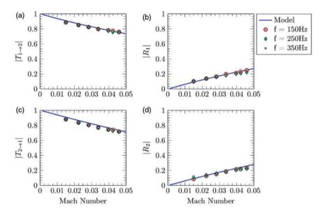
**Figure 44.** Magnitude of transmission and reflection coefficients as a function of upstream Mach number. Solid curve: predicted results for d = 16 mm,  $h_p = 20$  mm. Markers: measured results for an equivalent cylinder row (from Figure 11 in Surendran et al.<sup>86</sup>).
