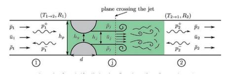
Figure 43. Schematic of two half-cylinders in a flow duct (from Figure 4 in Surendran et al. 86).
