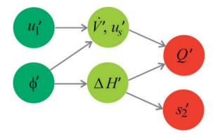
**Figure 36.** Causal links between upstream perturbations  $(u'_1, \phi')$ , flame front kinematics  $(u'_s, \dot{V}')$ , thermochemical properties  $(\Delta H')$ , and source terms for acoustic and entropy waves  $(Q', s'_2;$  after Figure 5.1 in Strobio Chen<sup>63</sup>).
