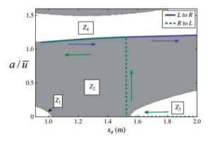
**Figure 18.** Hysteresis in the stability map of the Rijke tube with the heater position  $x_q$  as control parameter. Stable regions (white) are labelled  $Z_1$ ,  $Z_3$ ,  $Z_4$ ; the unstable region (grey) is  $Z_2$  (from Figure 11 in Bigongiari and Heckl<sup>39</sup>).
