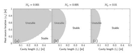
**Figure 40.** Stability maps in the  $l_c - x_q$  plane for a combustion system with three different Mach numbers (from Figure 8 in Surendran and Heckl<sup>78</sup>).
