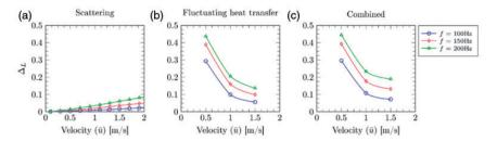
**Figure 48.** Absorption coefficient  $\Delta_L$  of a cavity-backed row of HEX tubes for three different HEX models: (a) acoustic scattering only. (b) fluctuating heat transfer only and (c) acoustic scattering and fluctuating heat transfer combined (from Figure 10 in Surendran et al. <sup>93</sup>).
