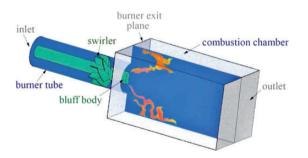
Figure 13. The BRS test rig (from Bigongiari et al.<sup>31</sup>).
