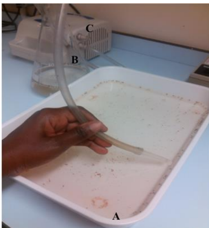
Figure 2.2.4: Picking of pupae in the insectary. A= Tray containing pupae and larvae, B=Conical flask with a tube attached to the pump C= Aspirator vacuum pump.
