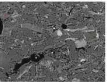
Pore Type: Shrinkage Crack Pores (SCP) 200µm Total Porosity 0.04% Microporosity 0.02% Micropore Frequency(100%); 16.8% Nanoporosity 0.02% Nanopore Frequency (100%); 83.3%
