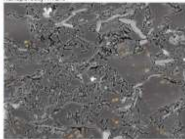
Pore Type: Moldic Pores (MP) 200µm Total Porosity: 0.99% Microporosity: 0.58% Nanoporosity: 0.41% Micropore Frequency (100%): 21.23% Nanopore Frequency (100%): 78.77%
