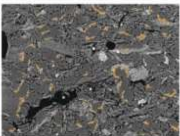
Pore Type: Grain Edge Pores (GEP) 200µm Total Porosity 2.13% Microporosity 2.11% Micropore Frequency(100%);76.19% Nanoporosity 0.02% Nanopore Frequency (100%); 23.81%
