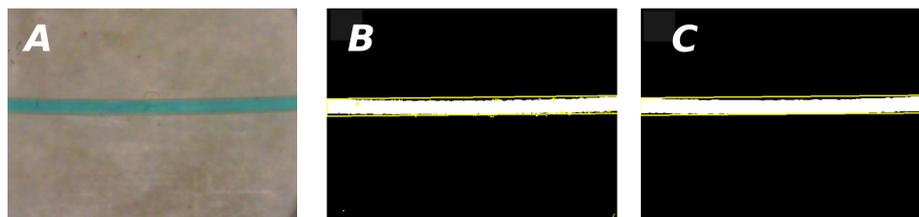
**Figure 2** A) A screenshot of an unprocessed frame from the webcam. B) Pixels filtered according to RGB value ('matching' pixels shown in white). A yellow bounding rectangle is shown around all clusters of matching pixels. A small number of 'noise' pixels can be seen on close inspection C) Image 'cleaned up' by performing opening/closing operations with an elliptical kernel to remove noise.
