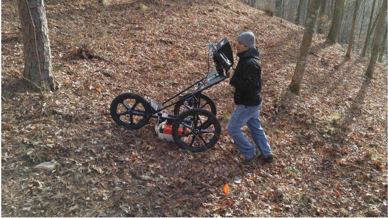
Figure 5. Site photograph facing east showing a SIR-4000 GPR with 400 MHz antenna being pushed up slope on the southside of War Hill (see Fig. 2 for location). Note colored flag indicates location of an HRD dog alert that is being tested with GPR.
