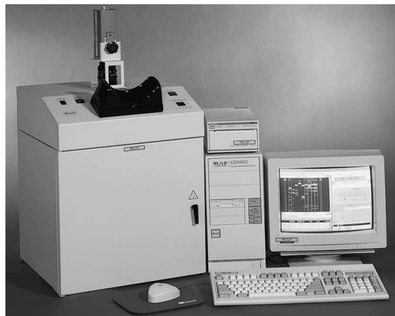
Figure 28: System for visualizing, analyzing and documenting ethidium bromide stained agarose and acrylamide gels
