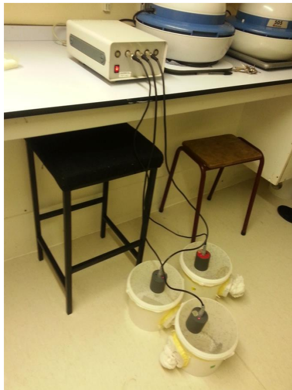
Figure 2.2. The feeder system (Hemotek membrane feeding system) – Used to feed the mosquitoes twice a week using horse blood, which was warmed to 37°C and presented to mosquitoes for 30min..
