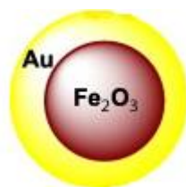
Figure 32: Diagram of a gold coated iron oxide nanoparticle (Wagstaff et al. 2012).
