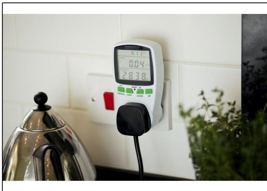
Figure 4.4. ENERGENIE power meter displaying Power (W), Energy (kWh), Volts, Amps, Hertz, Power Factor, Date and Time
