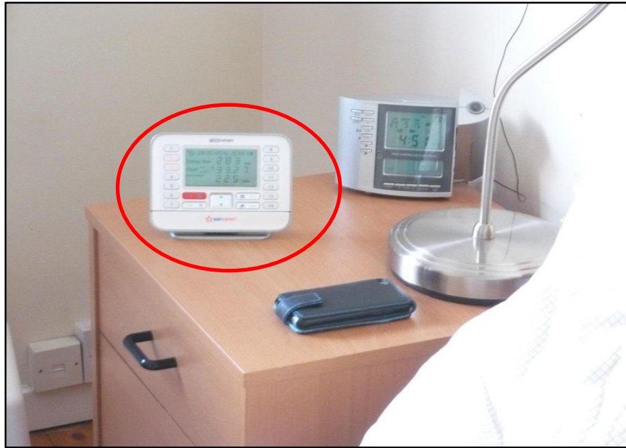
Figure 4.6. EDF ENERGY ECO-MANAGER display that allows wireless control over individual or group of appliances.
