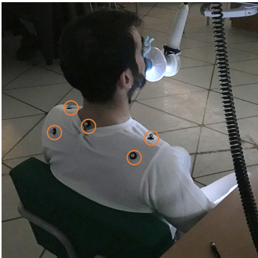
Figure 8-8. Markers placement on the subject's shoulder and C7
