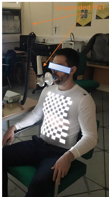
Figure 8-9. Study setup. The subject is sitting as far back in a high-backed chair as possible with his arms on the chair arms. The PNT suspended from the ceiling to avoid blocking SLP-grid.
