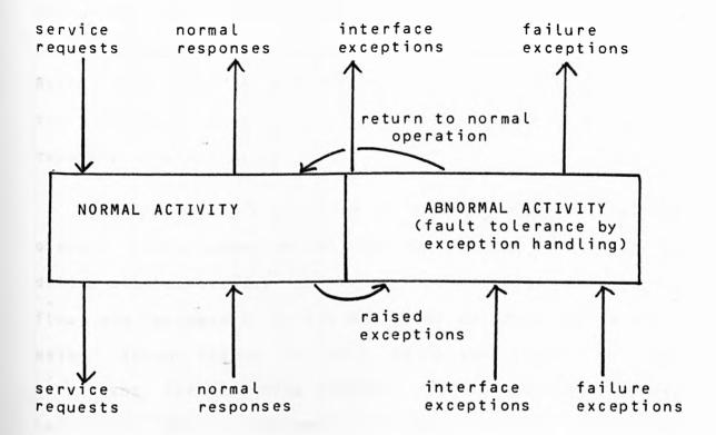
Masking of errors is achieved by raised exceptions (detected errors) invoking redundant code which takes corrective action and returns to normal processing. Detected errors which cannot be recovered within the component are indicated in the outputs as interface exceptions (illegal requests for service) or failure exceptions (errors due to the component), and must be dealt with outside the component. The component interfaces to other components and may have to deal with their errors.
