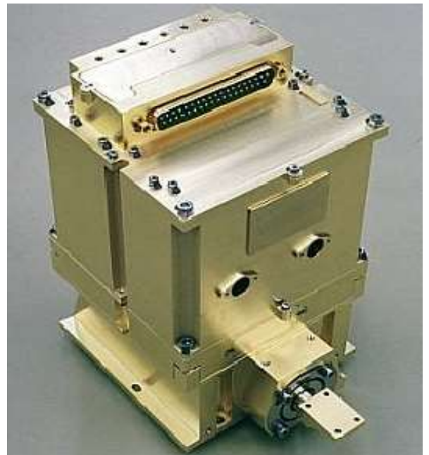
Figure 6.1- SCIAMACHY detector module, eight of which constitute part of the instrument on board the Envisat satellite (289).
