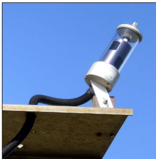
Figure 2.2- Sunshine duration meter used by many automated Met Office weather stations (162)
