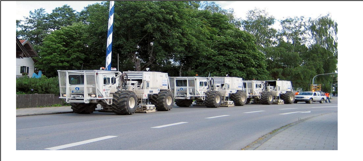
Figure 32: Truck train with mounted seismic survey 'Vibroseis' technology (SWM, 2015)
