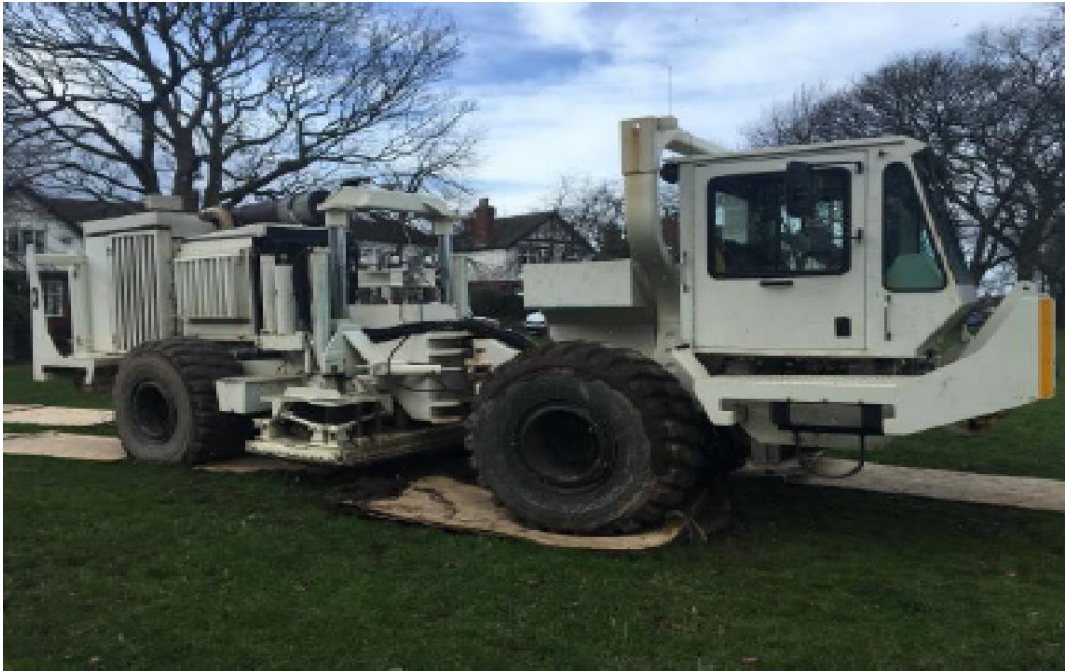
Figure 43: SoT "Vibroseis" Deep geo-sensing truck
