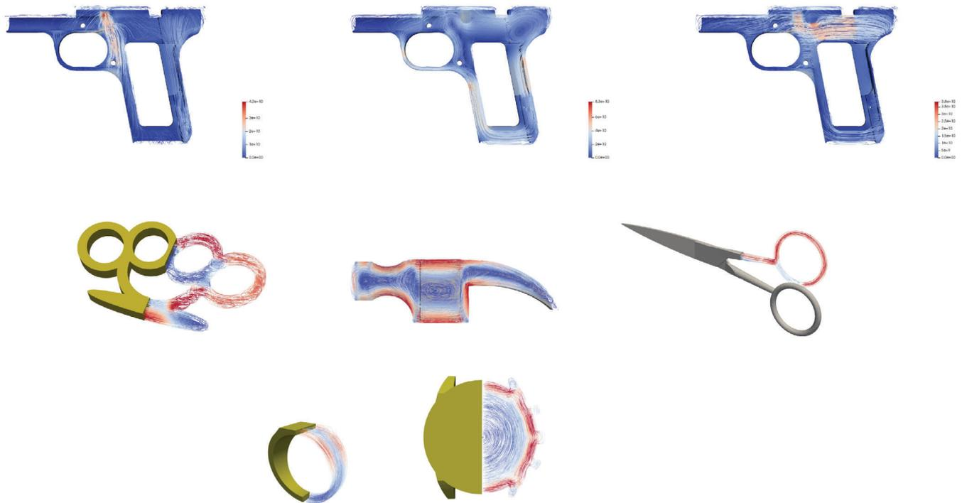
**FIGURE 12** Set of multiple threat and non-threat objects: Illustrative contours of  $\mathbf{J}_i^e = i\omega\sigma_*\boldsymbol{\theta}_i$  at  $\omega = 1 \times 10^4$  rad/s for a sample of the threat and non-threat objects
