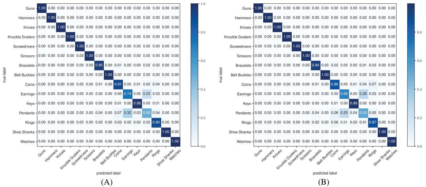
FIGURE 20 Set of multiple threat and non-threat objects: Comparison of confusion matrices for  $P^{(k)} = 5000$  when  $K = 15$  showing (A) MLP SNR = 40 dB and (B) MLP SNR = 20 dB
