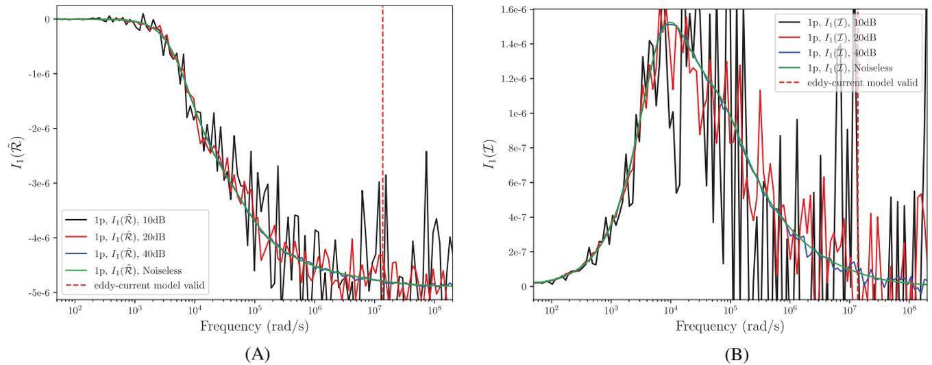
**FIGURE 2** Set of British coins: 1 p coin  $\alpha B$ ,  $\alpha = 0.001$  m,  $\mu_r = 1$ , and  $\sigma^* = 4.03 \times 10^7$  S/m showing the spectral signatures for noiseless and realizations of noise with SNRs of 40, 20, and 10 dB. (A)  $I_1(\tilde{\mathcal{R}}[\alpha B, \omega, \sigma_*, \mu_r])$  and (B)  $I_1(\mathcal{I}[\alpha B, \omega, \sigma_*, \mu_r])$
