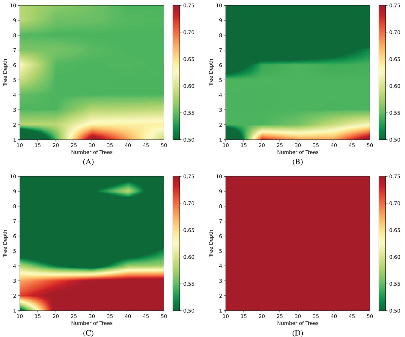
**FIGURE 22** Set of multiple threat and non-threat objects: Overall performance of the gradient boost classifier for different values in the hyperparameter space, for  $P^{(k)} = 2000$  with  $K = 8$  and  $\text{SNR} = 40$  dB, showing average  $\kappa$  score for different values  $n\_estimators$  and  $max\_depth$ , for different scaling regimes (A) Control, (B) A, (C) B, and (D) C
