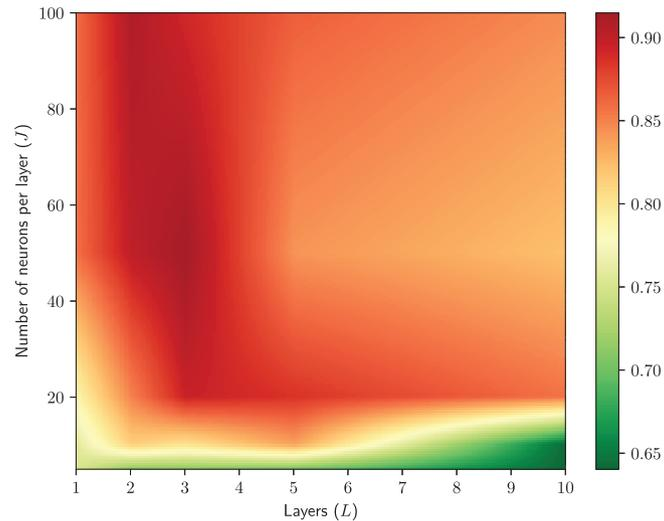
**FIGURE 14** Set of multiple threat and non-threat objects: Overall performance of MLP for different uniform network architectures, for  $P^{(k)} = 5000$  when  $K = 8$  and  $\text{SNR} = 40$  dB, showing  $\kappa$  score for different numbers of hidden layers  $L$  and numbers of neurons per layer  $J$
