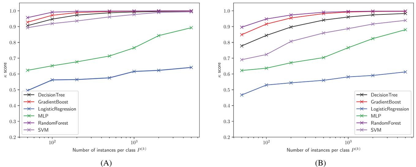
**FIGURE 15** Set of multiple threat and non-threat objects: Overall performance of different classifiers as a function of  $P^{(k)}$  when  $K = 8$  using the  $\kappa$  score (18) showing (A) SNR = 40 dB and (B) SNR = 20 dB
