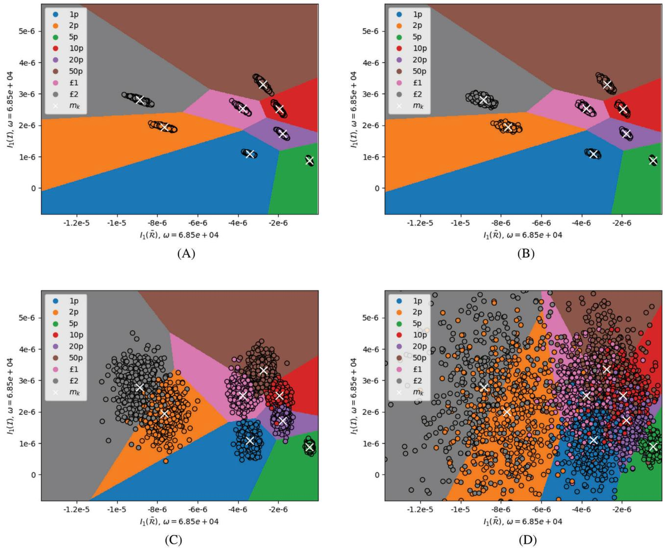
**FIGURE 5** Set of British coins: linear feature space splitting for the classes  $C_k, k = 1, \dots, K$ , for a simplified case of  $F = 2$  features based on  $\max_k \gamma_k(\mathbf{x})$  for logistic regression and  $P^{(k)} = P/K = 2000$  for (A) noiseless and SNR of (B) 40 dB, (C) 20 dB, (D) 10 dB
