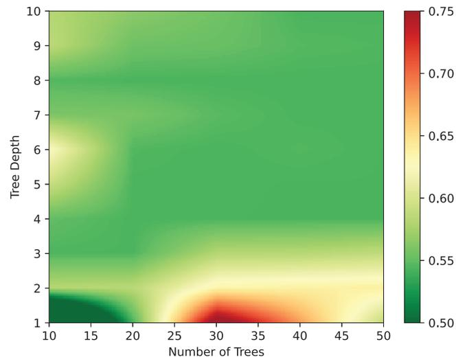
**FIGURE 21** Set of multiple threat and non-threat objects: Overall performance of the gradient boost classifier for different values in the hyperparameter space, for  $P^{(k)} = 2000$  when  $K = 8$  and  $\text{SNR} = 40$  dB, showing average  $\kappa$  score for different values of numbers of trees (`n_estimators`) and tree depth (`max_depth`)
