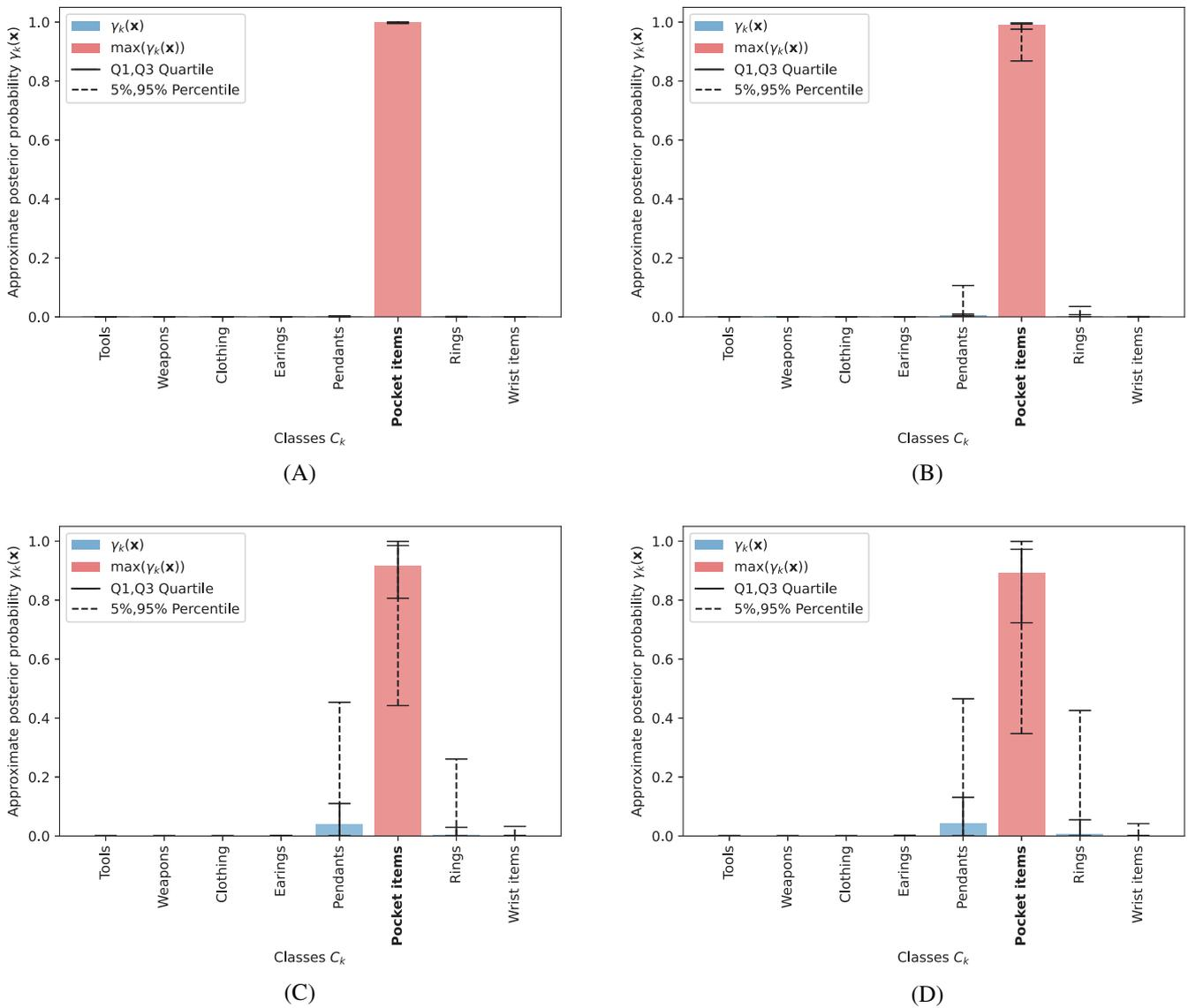
**FIGURE 16** Set of multiple threat and non-threat objects: Approximations  $p(C_k|\mathbf{x}) \approx \gamma_k(\mathbf{x})$  to posterior probabilities  $p(C_k|\mathbf{x})$ ,  $k = 1, \dots, K$ , where  $(\mathbf{x}, \mathbf{t}) \in D_8^{(\text{test},(2))}$  for  $P^{(k)} = 5000$  when  $K = 8$  showing the classifiers (A) gradient boost SNR = 40 dB, (B) gradient boost SNR = 20 dB, (C) MLP SNR = 40 dB, and (D) MLP SNR = 20 dB
