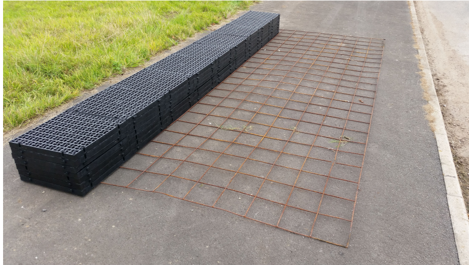
Figure 3. The data fusion testing mesh in-situ, with a simulated cover depth of 289 mm set up.
