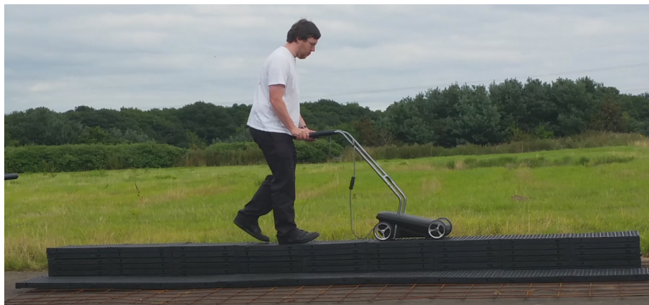
Figure 4. An EMAD scan being carried out with a simulated cover depth of 251 mm.
