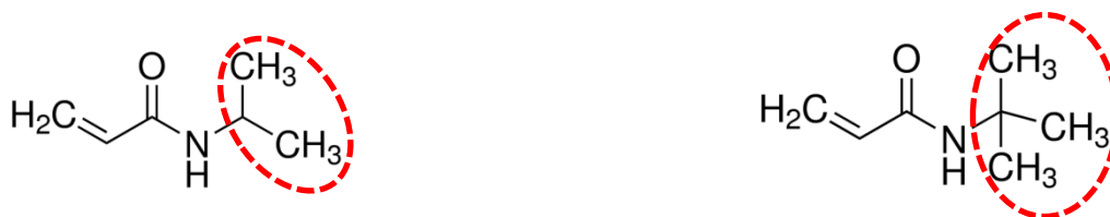
Figure 2-5. Monomeric structure of NIPAM and NTBAM. The main difference between the two materials in the basic chemical structure is illustrated by the red dotted circles.
