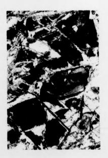
FIGURE 3.5.1. Twinned albitised plagioclase containing abundant white mica flakes, sample 167F (Moel Siabod).
