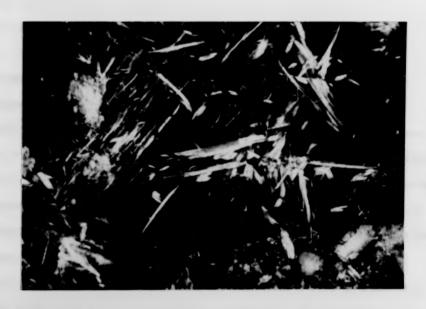
FIGURE 4.18.1. Epitaxial overgrowth of actinolite on a relict clinopyroxene crystal, sample 168J (Moel Siabod). XP. X14.
