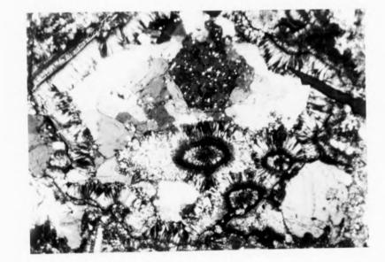
FIGURE 4.23. Chlorite, quartz and (minor) ferristilpnomelane infilling vesicles, sample 179C (Moel Siabod).
