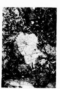
pseudomorphs the original ore phase and occasionally there is evidence that the ores had exsolved into Ti-rich (ilmenite) and Fe-rich (magnetite) phases, the former now being pseudomorphed by sphene whilst the latter remains relatively unaltered (Figure 3.1.2.).
