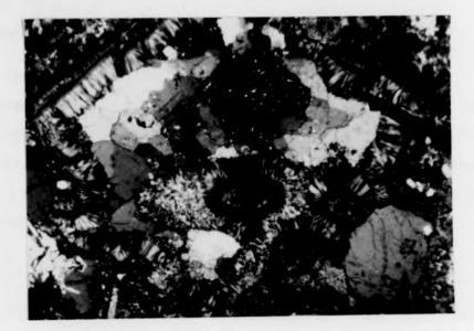
FIGURE 4.23. Chlorite, quartz and (minor) ferristilpnomelane infilling vesicles, sample 179C (Moel Siabod).
