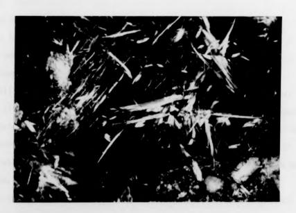
FIGURE 4.18.1. Epitaxial overgrowth of actinolite on a relict clinopyroxene crystal, sample 168J (Moel Siabod).
