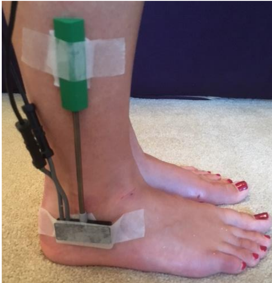
Figure 6.5 Set up for placement of the goniometer
