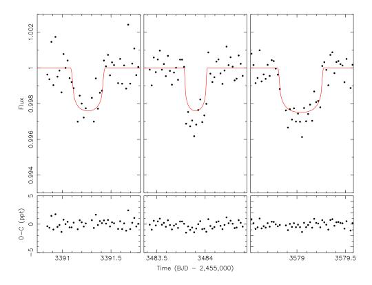
**Figure 8.** The transits of the CBP across the primary in Sector 3 (left), Sector 6 (middle), and Sector 10 (right) and the best-fitting model. The Sector 6 and 10 events were fit using 2-min cadence data, but for clarity we show the data binned to the 30-min cadence.
