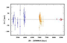
Figure 5. Left: radial velocities for TOI-1338, phase-folded on the binary orbital period of 14.61 days, taken with the CORALIE instrument (blue and orange) and HARPS (red). Right: residuals to the single-Keplerian radial velocity fit over time. The change in CORALIE residuals between blue and orange measurements coincide with a fibre change (see text for details).
