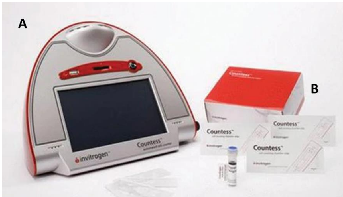
Figure 2.1: Countess automated cell counter. A: automated cell counter, B: single use Countess cell counting chamber slides (Image from Invitrogen).
