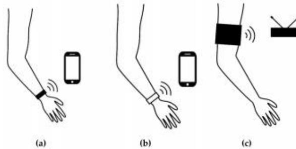
**Figure 1.** Wearables and apps for epilepsy seizure detection: (a) dedicated wrist-worn sensing device and companion app (e.g., Embrace and Epi-Care free); (b) app using sensed data from a compatible consumer wrist-worn tracker (e.g., the SmartWatch Inspyre app with an Apple or Samsung device); (c) a non-wrist wearable with a base station (NightWatch).
