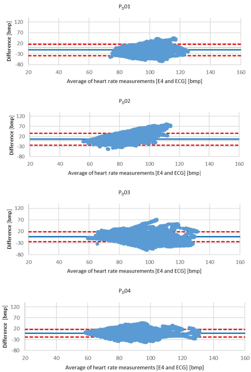
**Figure 4.4:** Bland-Altman plots for the E4 compared with the ECG chest strap for 12-hours free living.
