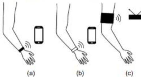
**Figure 1.** Wearables and apps for epilepsy seizure detection: (a) dedicated wrist-worn sensing device and companion app (e.g., Embrace (Empatica) and Epi-Care free (Danish Care Technology) devices); (b) app using sensed data from a compatible consumer wrist-worn tracker (e.g., the SmartWatch Inspyre app (Smart Monitor) with an Apple or Samsung device); (c) a nonwrist wearable with a base station (NightWatch (LivAssured, B.V) device).
