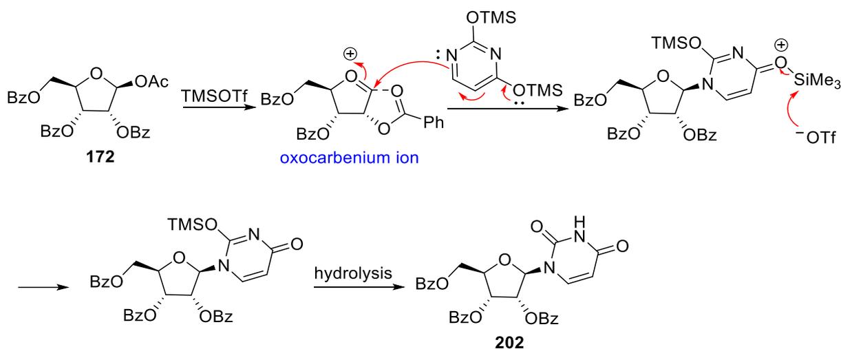
Scheme 36. Mechanism of Vorbrüggen reaction.
