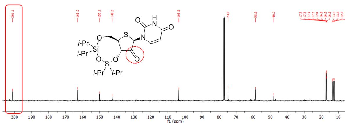
Figure 28. <sup>13</sup>C NMR (CDCl<sub>3</sub>, 101 MHz) spectrum of **246**.
