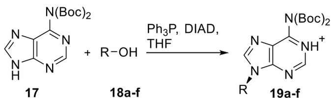
Scheme 5. Synthesis of carbocyclic adenosine analogues *via* modified Mitsunobu reaction.
