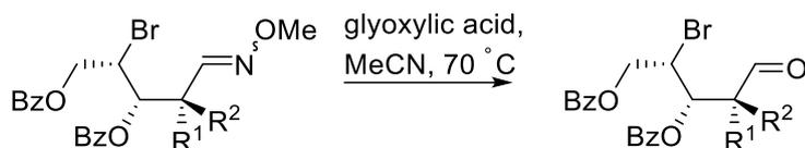
Oxime (1.0 equiv.) was dissolved in MeCN (0.5 M), glyoxylic acid (7.0 equiv.) added, and the solution heated to 70 °C overnight. The reaction was cooled to rt, poured onto H<sub>2</sub>O and extracted with EtOAc (2 ×). The combined organic phases were washed with H<sub>2</sub>O (5 ×) and brine (1 ×), dried over anhydrous Na<sub>2</sub>SO<sub>4</sub>, filtered and dried *in vacuo* to obtain a mixture of the crude product aldehyde and the hydrate of the aldehyde.
