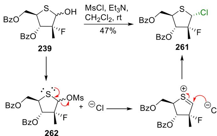
Scheme 77. Alternative proposed mechanism for the formation of **261**.
