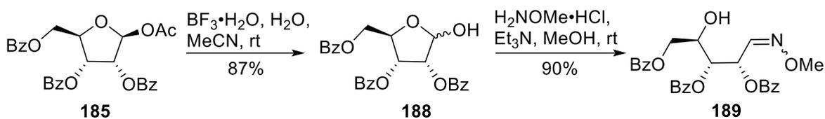
Scheme 29. Hydrolysis of **185** anomeric acetate to obtain **188** and conversion to the corresponding oxime **189**.
