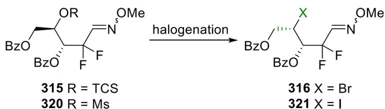
Scheme 106. S<sub>N</sub>2 C4 halogenation reaction.
