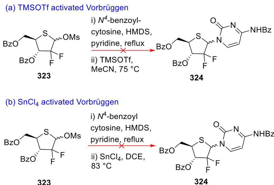
Scheme 109. Attempted synthesis of **324** from **323** via a) TMSOTf or b) SnCl<sub>4</sub> activated Vorbrüggen.
