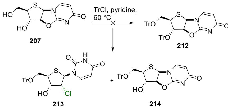
Scheme 47. Products **213** and **214** prepared from reaction of **207** with trityl chloride.
