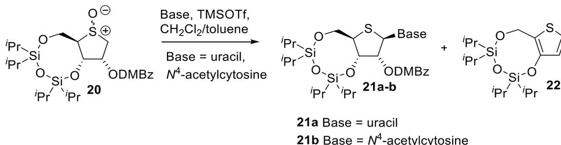
Scheme 6. Synthesis of **21a – b** and **22** *via* a Pummerer-type glycosylation.
