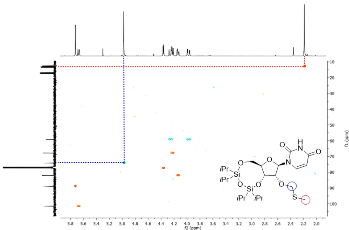
Figure 30. HSQC-DEPT correlation spectrum of **249**. Pale blue contours indicate CH<sub>2</sub>, red contours indicate CH or CH<sub>3</sub>.
