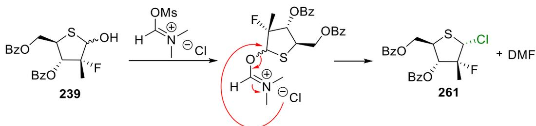
Scheme 76. A) Formation of iminium salt from reaction of MsCl with DMF; b) Formation of chloroglycoside **261** by reaction of **239** with the iminium salt.
