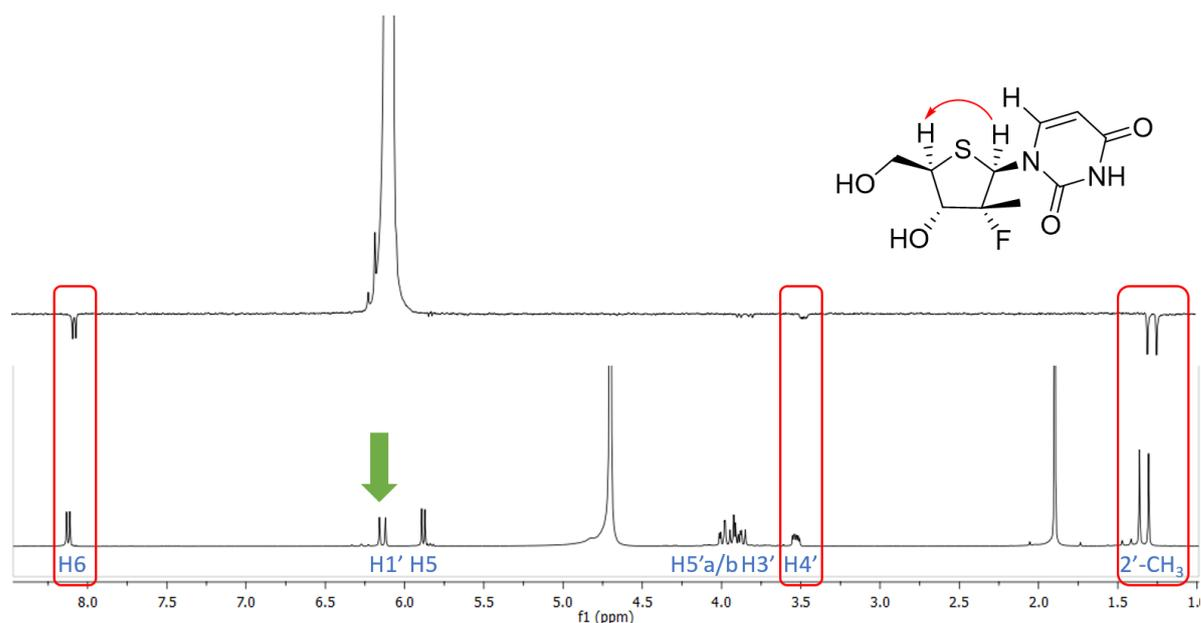
Figure 35. NOE of **240β** where H1' is irradiated and corresponding  $^1\text{H}$  NMR spectrum ( $\text{D}_2\text{O}$ , 400 MHz).
