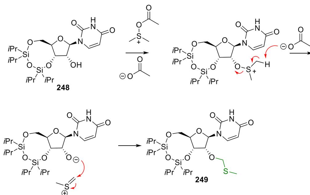
Scheme 64. Proposed mechanism for the formation of **249** via rearrangement under Albright Goldman conditions.
