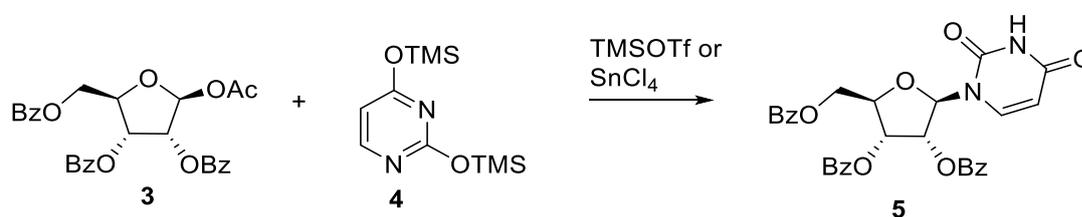
Scheme 1. Vorbrüggen synthesis of nucleoside **5** via Lewis acid catalysis by TMSOTf.
