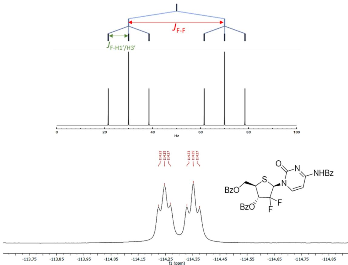
Figure 44. Tree diagram showing splitting of the 2-fluorine peaks for **324β** and  $^{19}\text{F}$  NMR ( $\text{CDCl}_3$ , 376 Hz) of **324β**.
