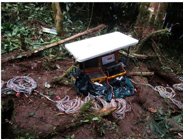
Fig. 7. Using electrical resistivity tomography (ERT) in tropical terrain near Casanare to locate clandestine graves of disappeared, difficult to access and irregular ground to collect datasets from.
