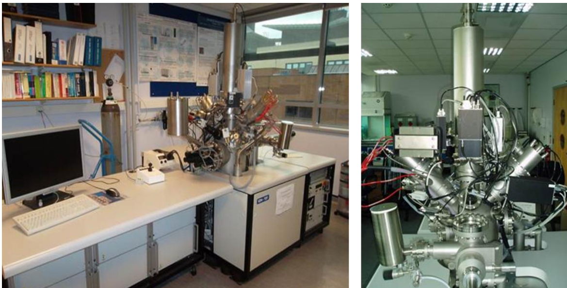
Figure 2.4 Photograph illustrating the ToF-SIMS instrument set-up. Courtesy of Dr David Scurr, Nottingham University.
