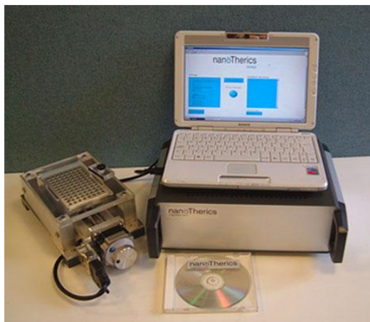
Figure 2: The magnefect-nano system (nanoTherics Ltd., Stoke-on-Trent, UK). A laptop with software is pictured above the computerised motor that drives an oscillating magnetic array, situated to the left of this image and configured for a 96-well plate. Image courtesy of nanoTherics Ltd.
