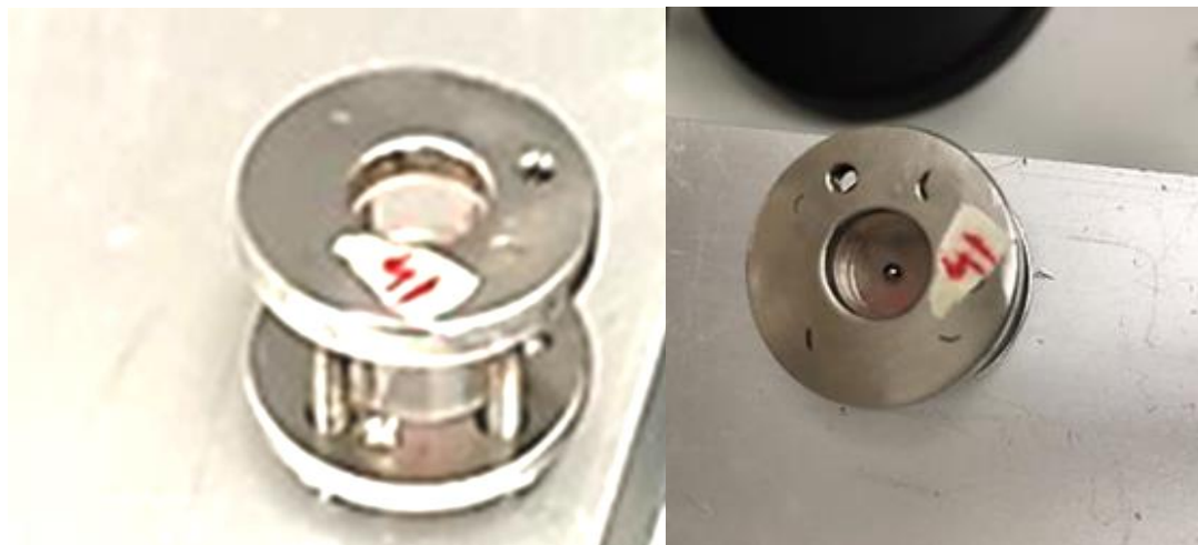
Figure 3.6: Mounted vaginal tissue segments within plastic O-rings secured within a metal screw and plate system.
