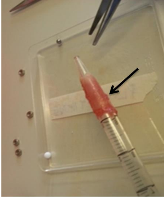
Figure 3.9: Insertion of tubular vaginal wall over a cylindrical object to enable precise incising in the process of creating a rectangular flat sheet for mounting on mechanical test device. The arrow indicates the tissue's location.
