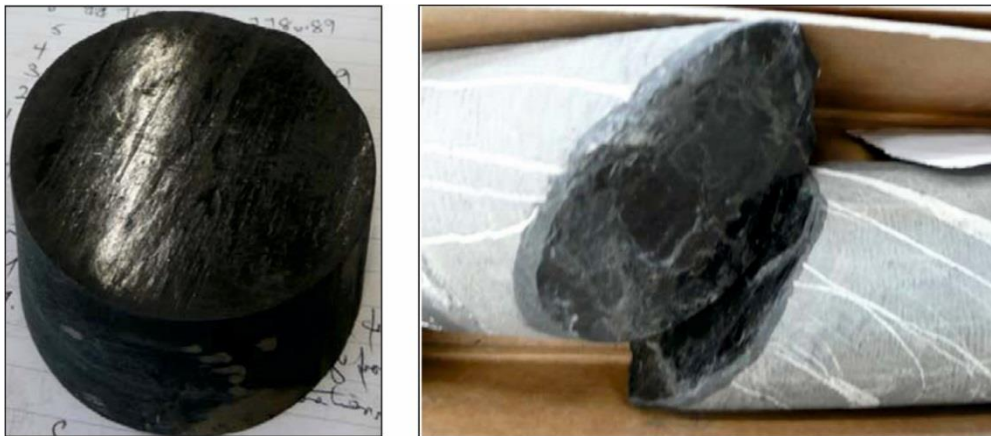
Figure 6.6: Polished slickenside bedding surfaces from the well Preese Hall 1 in the United Kingdom. From de Pater and Baisch (2011).
