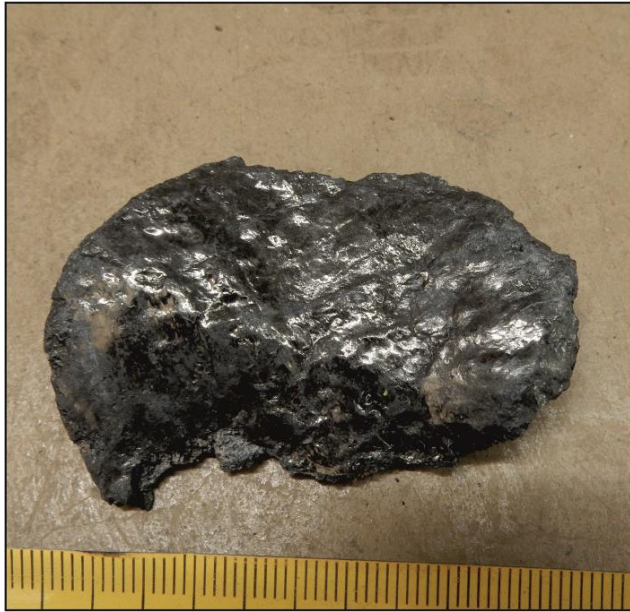
Figure 6.5: A section of core displaying a polished slickenside surface from the Whitehill Formation in borehole KZF-1 at a depth of 443.3 m
