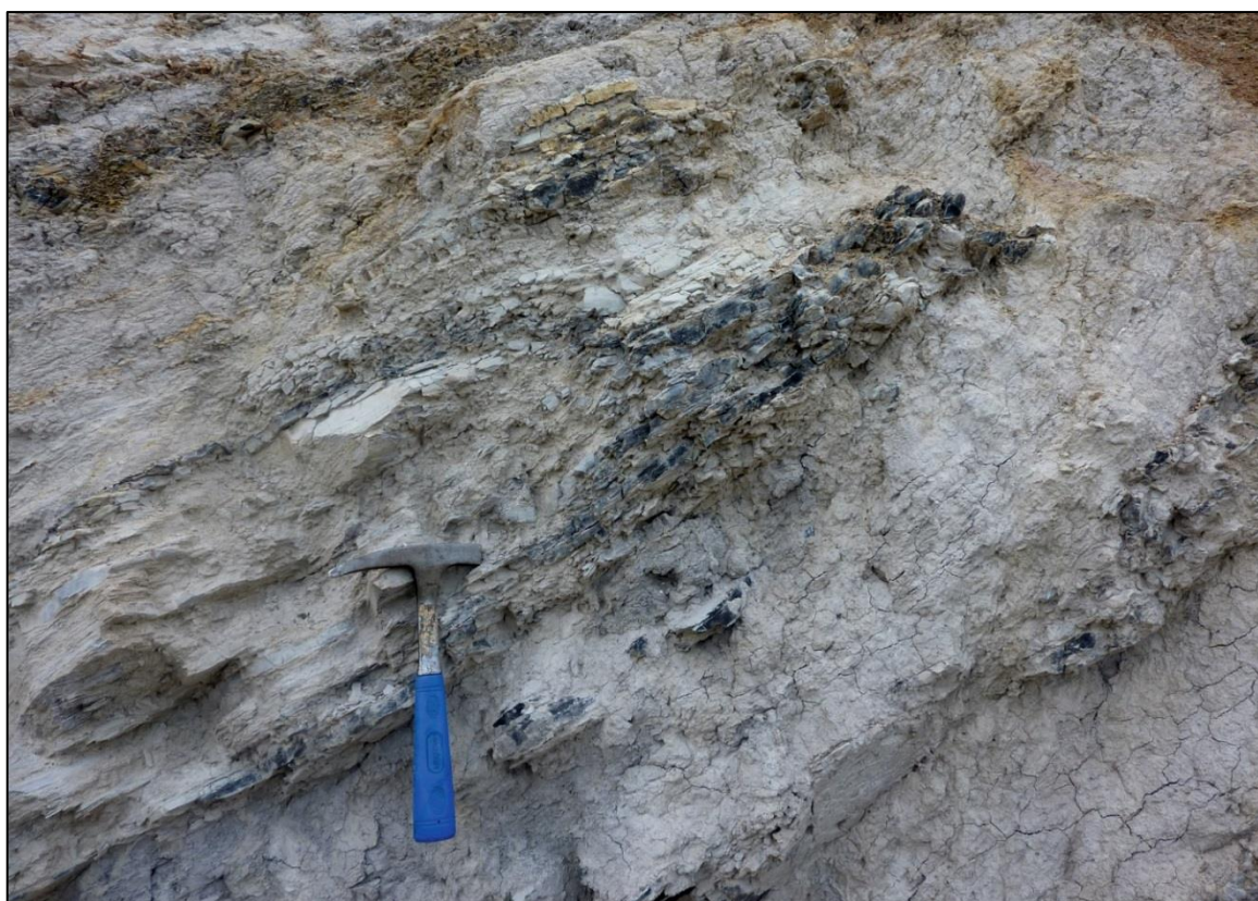
Figure 2.13: Weathered Whitehill Formation (see Figure 2.11) with characteristic white gypsum, from the breakdown of sulphides, exposed along the Ecca Pass (Eastern Cape, South Africa).
