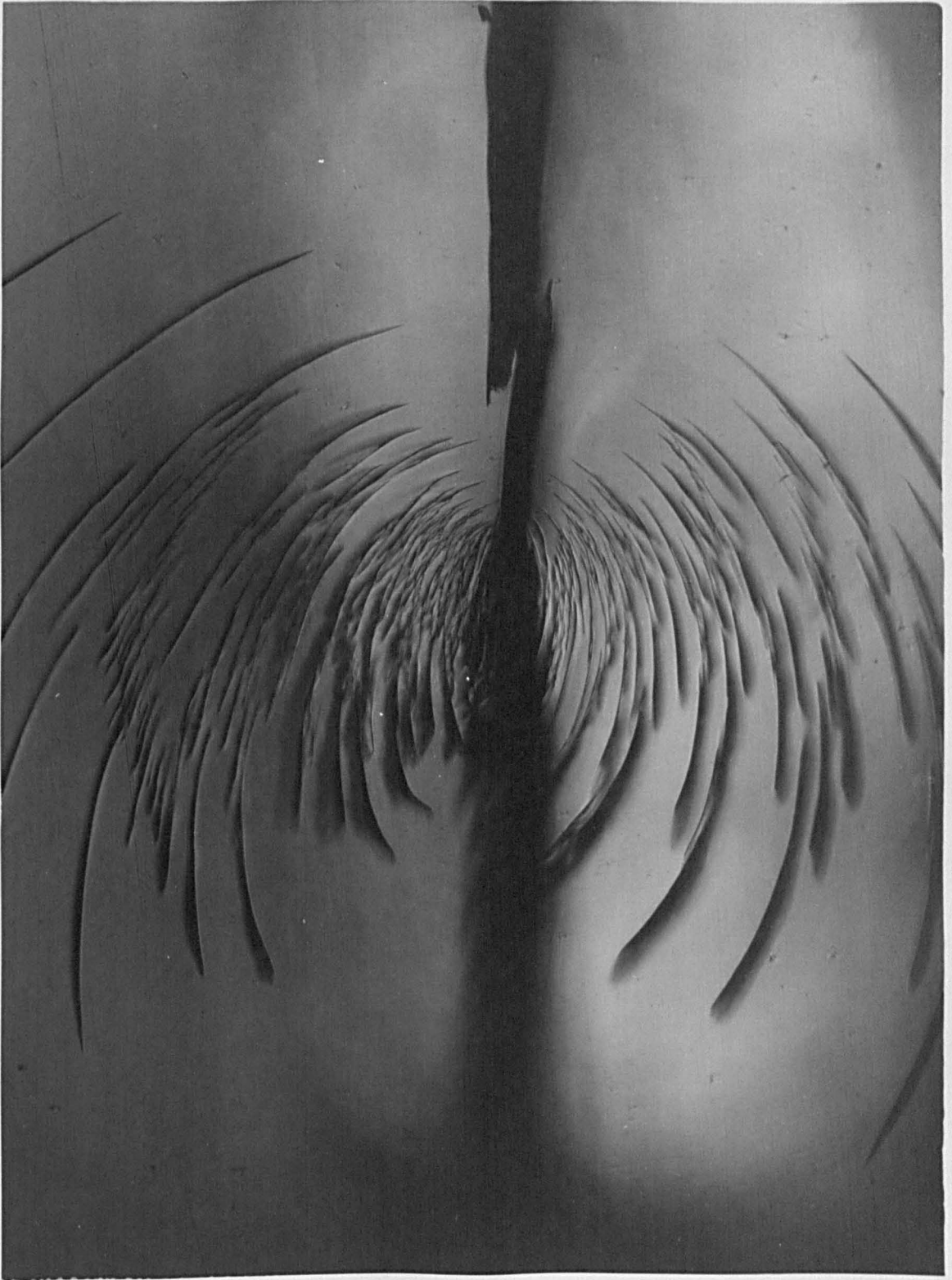
Fig. (3.7) Crazes around a crack tip in polystyrene (magnification x 100)
