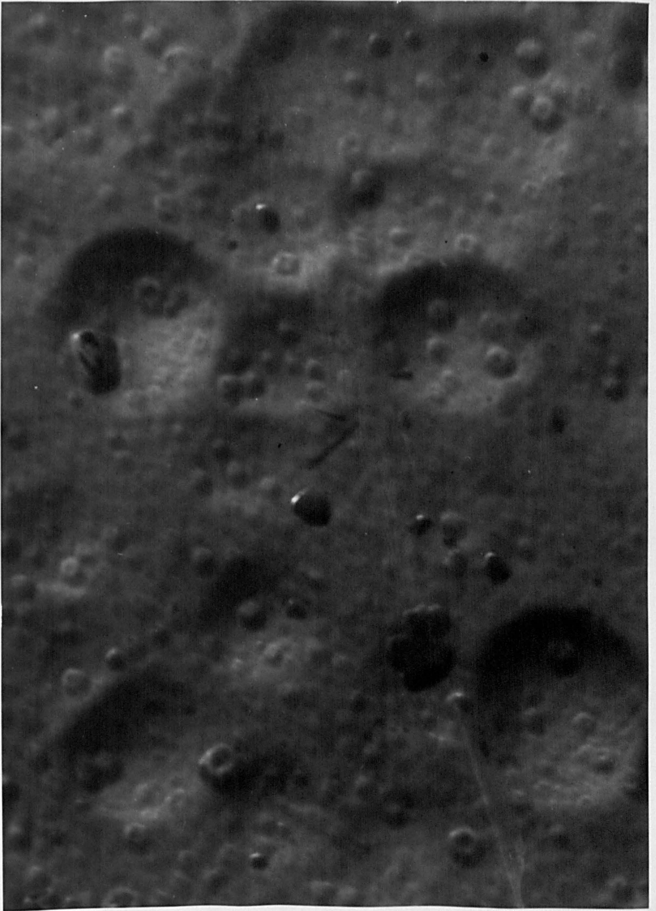
Fig. (3.13) The fracture surface of CT200/HT901 having been etched in chromic acid (magnification \times 40,000 )
