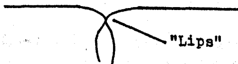
Figure 8.4 Schematic representation of the contact between two opposite crack faces possessing hypothetical surface irregularities (a) and shear "lips" (b). Plastic deformation at the points of intimate contact would result in increasing the real area of contact.
