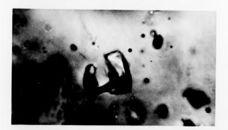
of negative crystal faces. In several samples they show some evidence of deformation such as stretching and flattening (Figure 7.1.2.). Many of these features are typical of 'secondary' inclusions formed after the host mineral crystallised (Roedder, 1979).
