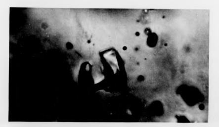
FIGURE 7.3. "Necking down" phenomena in fluid inclusions, sample 318. X800.
