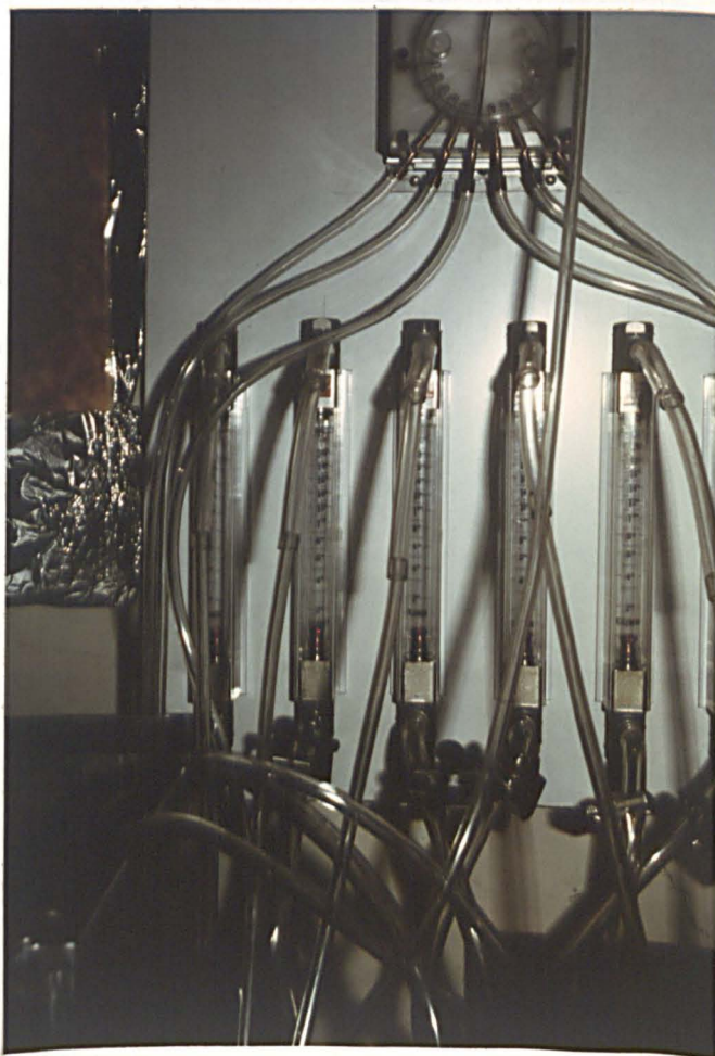
Plate 7 Equipment used to measure CO 2 flux: flow meters and 6-way switch.
