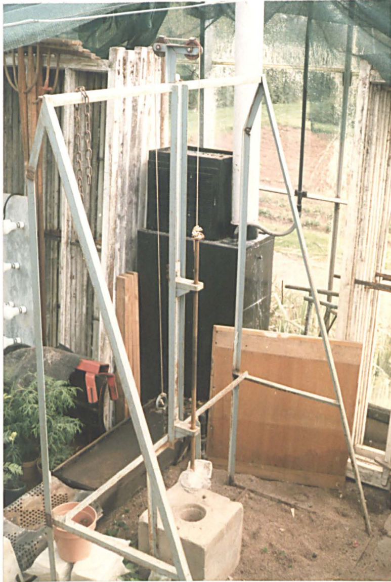
Plate 4 Falling tamp apparatus used to apply simulated trampling treatments to pots of grass.
