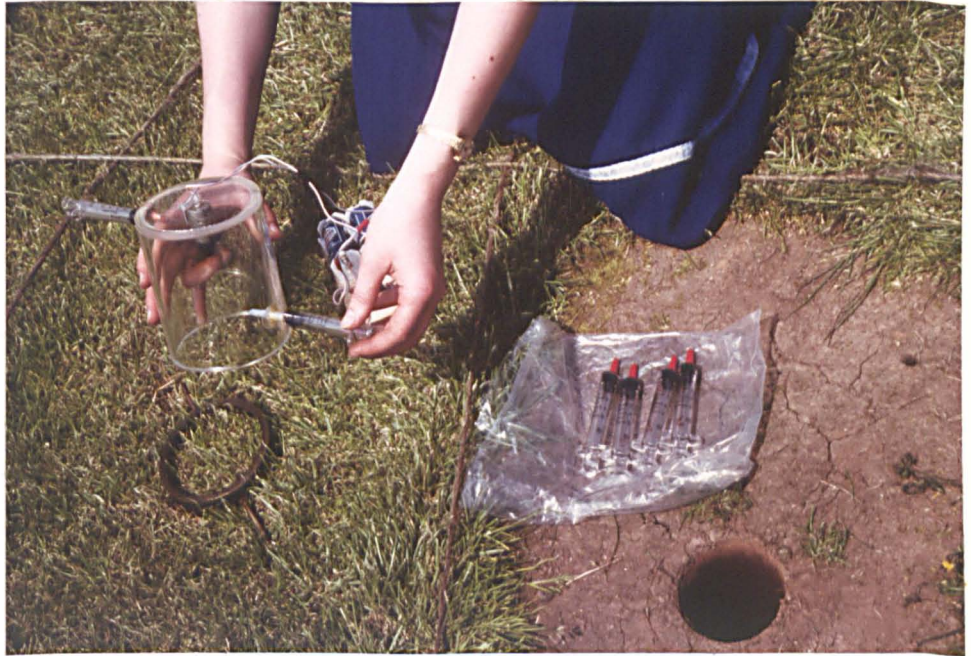
Plate 41 Field plots: Apparatus used to measure sward \text{CO}_2 flux.
