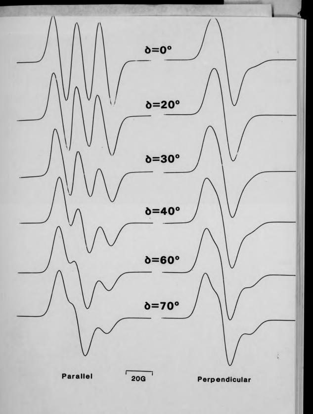
$\frac{\text{Fig. 5.13}}{\text{of misalignment (Tilt = 0°)}} \ \, \text{Computer simulations for a fibre for several angles}$
