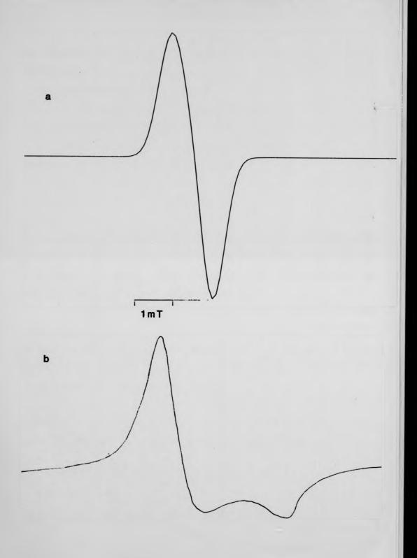
Fig. 6.7 (a) 9.5-GHz Fibre simulation of the A-form spectrum given that the hyperfine term is zero and  $\delta$  = 90°. (b) The Q-band simulation demonstrating the line broadening due to the g-value anisotropy.
