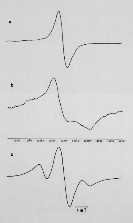
The 9.5-GHz Fibre spectrum corresponding to A-form  $\phi W{=}14$  DNA. The 35-GHz Fibre spectrum corresponding to A-form  $\phi W{=}14$  DNA. Fig. 6.6 (a)
