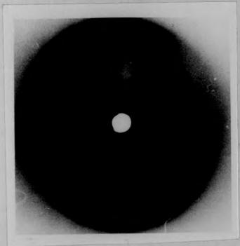
Fig. 5.10 A- and B-form X-ray diffraction patterns for a FPRZ+-DNA fibre recorded at 33% and 98% relative humidities.
