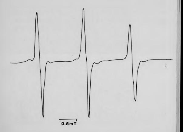
Fig. 6.3 The 9.5-GHz ESR spectrum of spin-labelled  $\phi W$ -14 DNA in aqueous solution.
