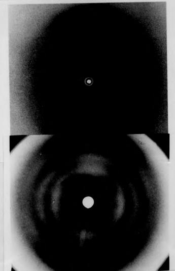
Fig. 6.4 Spin Labelled  $\phi$ W-14 Fibre Diffraction Patterns recorded at (a) 33% (b) 66% (c) 98% relative humidities.
