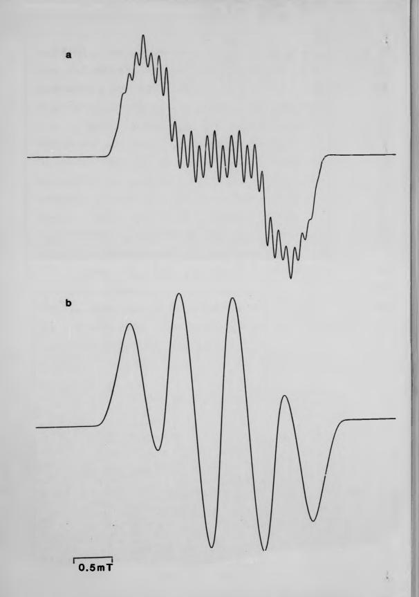
Fig. 5.9 (a) Computer simulation of the FPRZ+ spectrum. (b) Computer simulation of the PRTZ+ spectrum.
