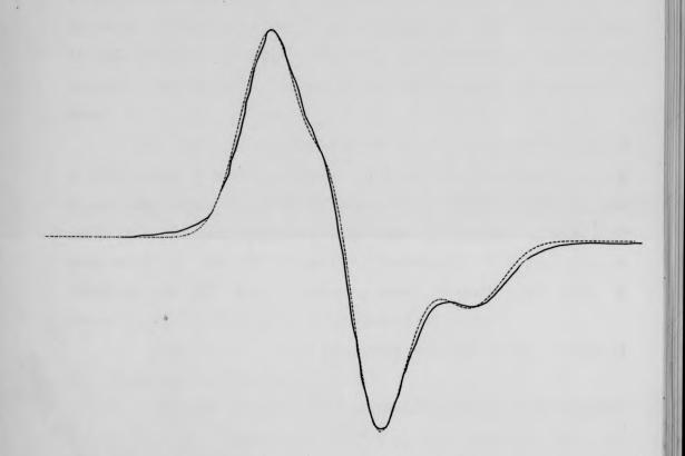
$\underline{\text{Fig. 5.12}}$  Computer simulation of the FPRZ+-DNA gel ESR spectrum.
