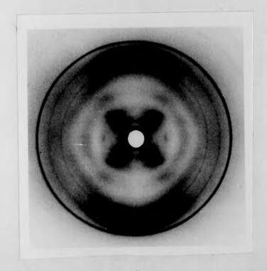
Fig. 4.28 A- and B-form X-ray fibre diffraction patterns for P/D = 70.
