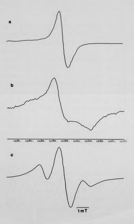
The 9.5-GHz Fibre spectrum corresponding to A-form  $\phi N\text{-}14$  DNA. The 35-GHz Fibre spectrum corresponding to A-form Fig. 6.6 (a)
