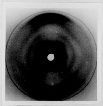
Fig. 4.30 C-form and B-form fibre diffraction patterns (P/D = 6).
