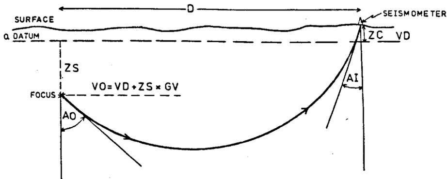
Fig. A-1: Seismic structure model with linear increase of seismic velocity with depth.
