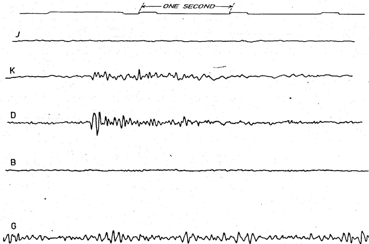
Fig. 4.10.1. Seismogram of first type of tremor recorded at 1977 6-6 06-23. Low amplitude and short duration of seismic waves probably indicate tremors which originate near the detection site. Letters designate seismometer names.
