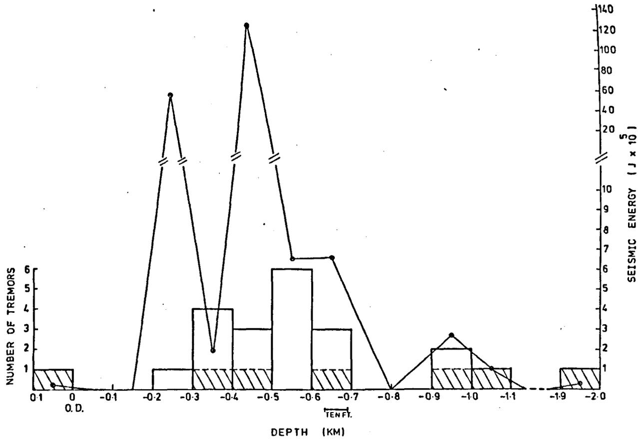
Fig. 9.6.4. A plot showing the number of tremors and the corresponding seismic energy release occurring within each 100 m depth interval in area D. The depth ranges of the active mine workings in the Ten Feet (TEN FT.) seam is also shown. The shaded area represents tremors with a shear source origin.
