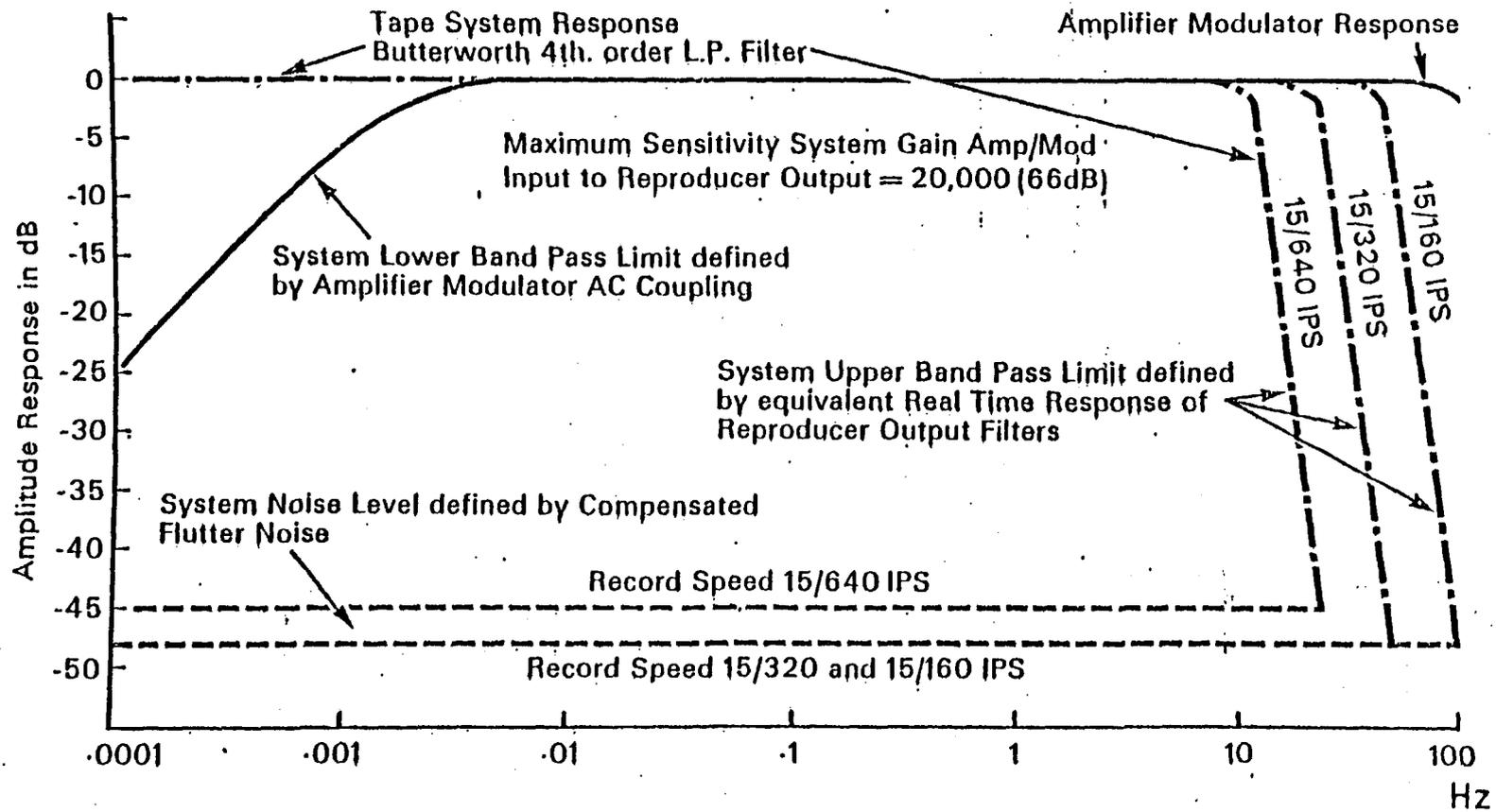
Fig. 4.4.1. Overall Geostore system frequency response (excluding seismometer).
