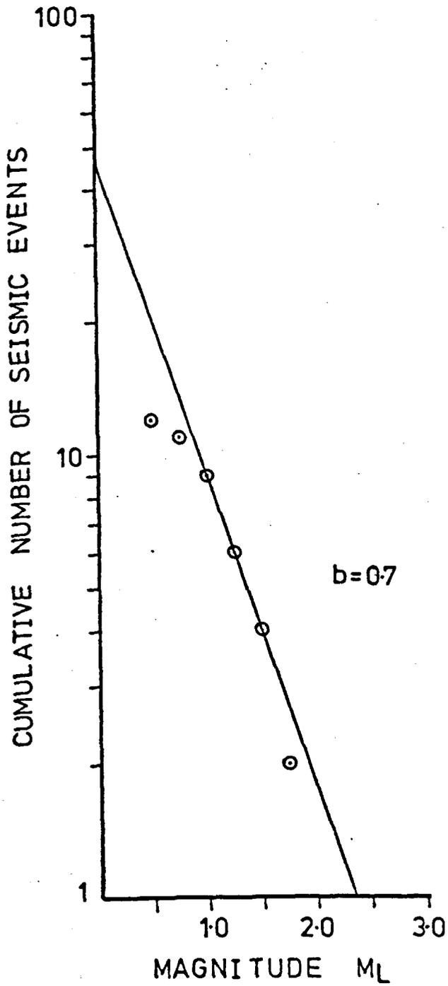
Fig. 9.7.8. A plot showing the frequency-magnitude distribution for tremors occurring in area E.
