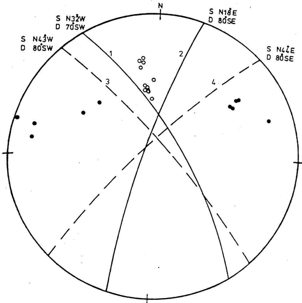
Fig. 9.4.7. A composite focal mechanism for tremors which occurred in area B.
