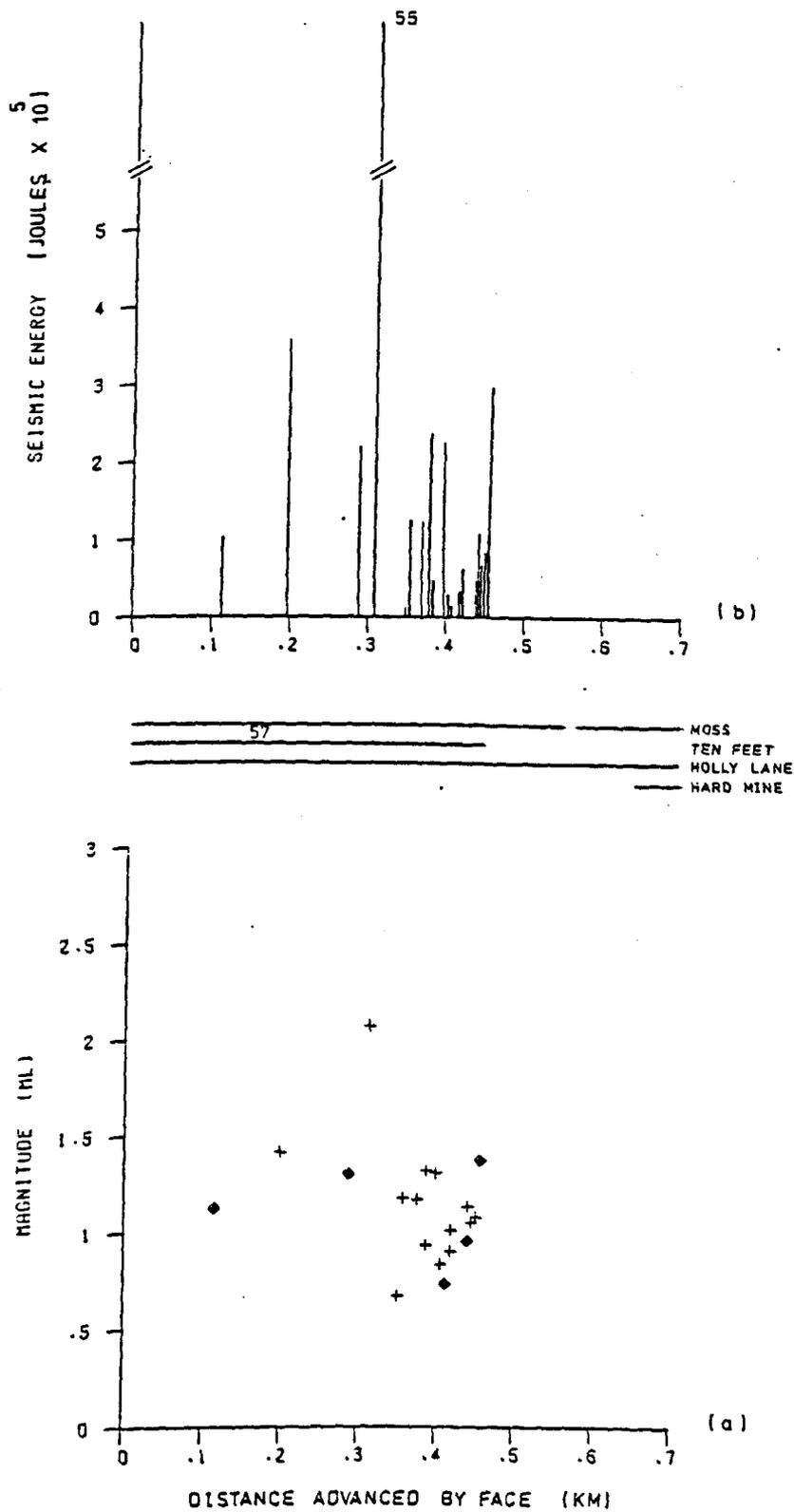
Fig. 9.6.9. Plots of (a) tremor magnitude,  $M_L$ , and (b) seismic energy release, against the distance advanced by the face for tremors occurring during the mining of panel 57 in area D. The regions where the panel face lies below or above previous workings in the Moss, Holly Lane and Hard Mine seams are also shown.
