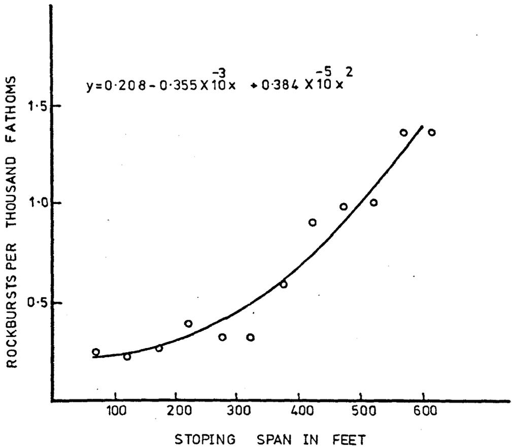
Fig. 3.4.2. The influence of stoping span, in a typical longwall face, on the rock burst incidence. (After Pretorius, 1964).
