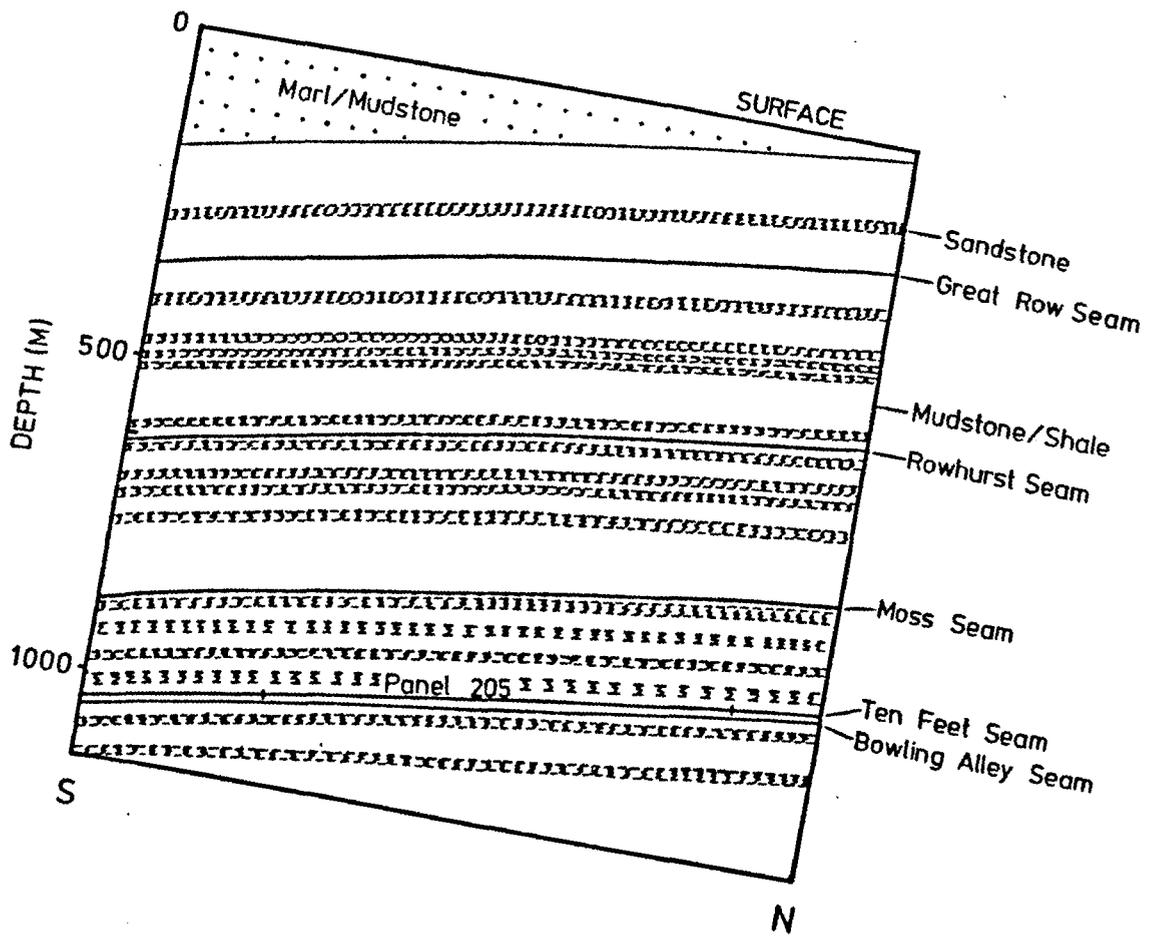
Fig. 7.1.1. General geological section along panel 205 showing major sandstone units and some important coal seams. (Taken from Kuszniir et al., 1980b).
