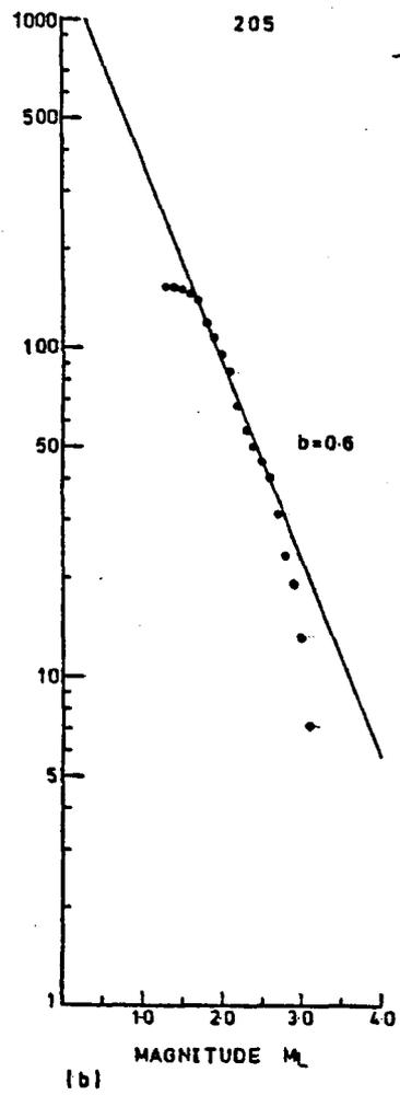
Fig. 7.4.1. Frequency-magnitude distribution for tremors occurring during the mining of panels 205 and 206.
