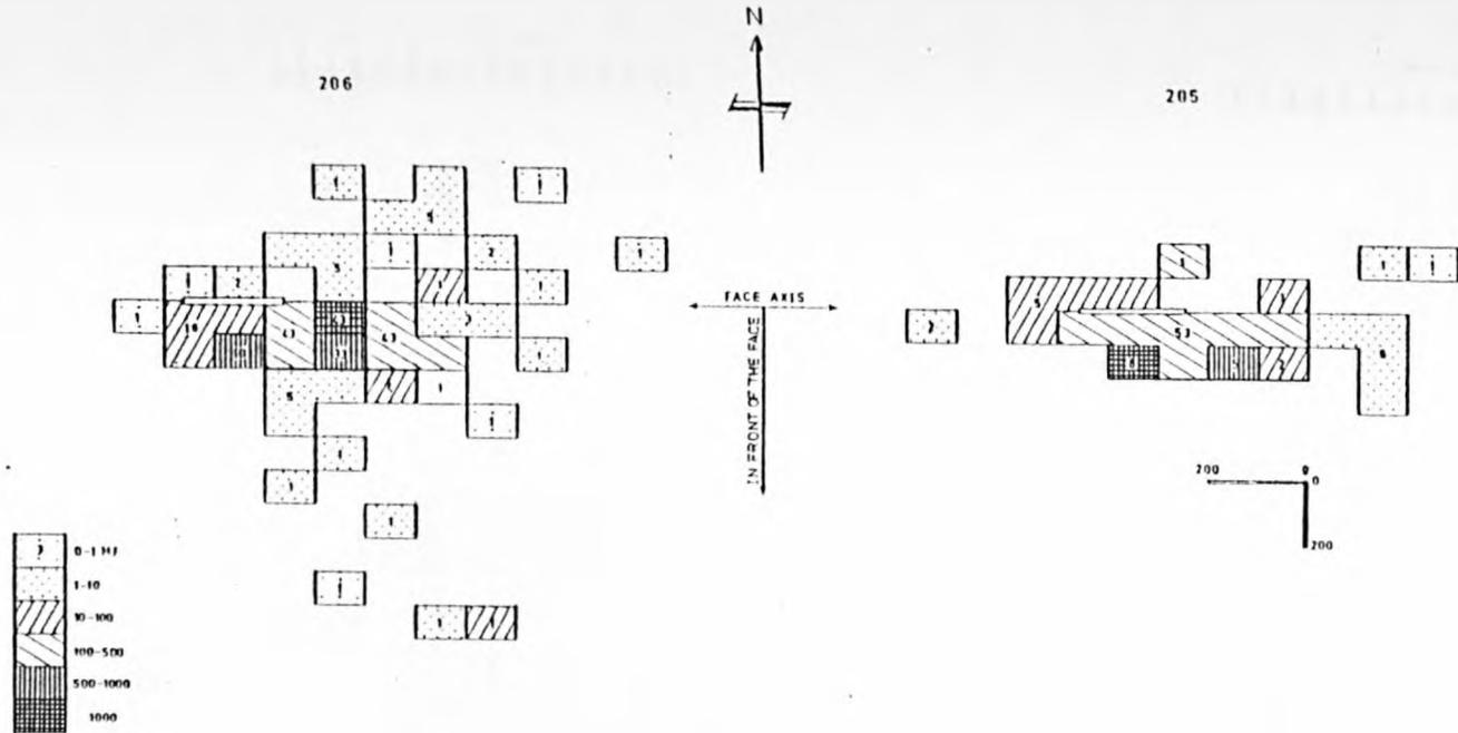
Fig. 7.4.4. Plan view showing the total amount of seismic energy released per 100 m x 100 m area (represented by a rectangle) relative to the position of the working face, at the time of occurrence, for tremors occurring during the mining of panels 205 and 206. Integers indicate the total number of tremors which occurred within the specific area.
