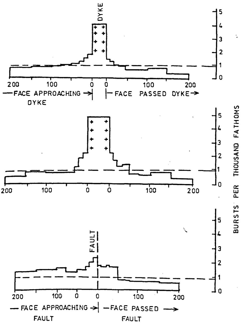
Fig. 3.4.4. The effect of dykes and faults on rock burst incidence in the Witwatersrand gold field. (After Hill and Denkhaus, 1961).
