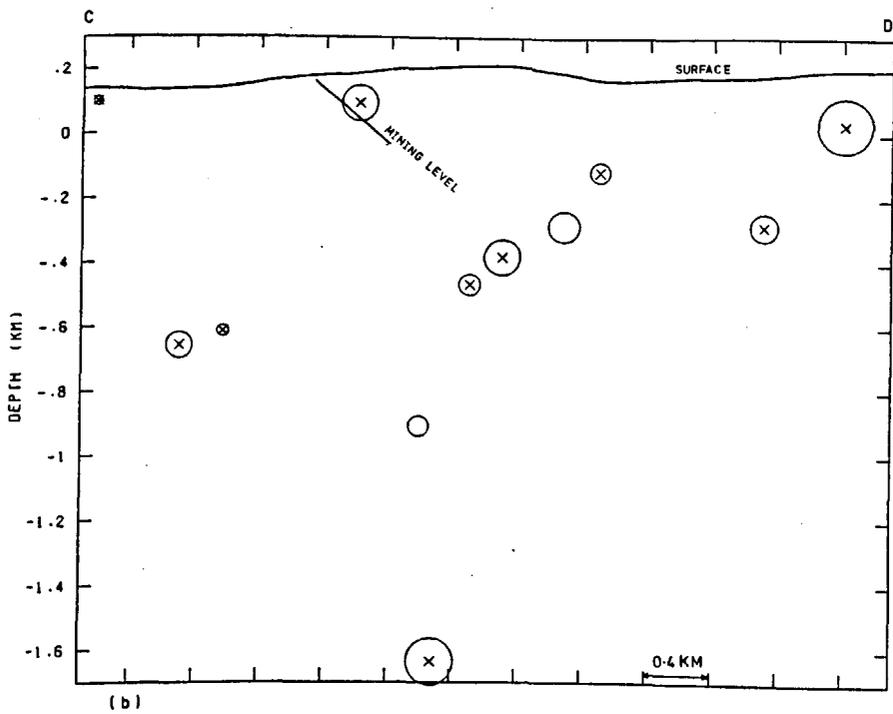
Fig. 9.7.3. Hypocentre sections (A-B, C-D, Figure 9.7.2) of tremors located in area E, showing the position of tremor hypocentres with respect to the active and old mine workings and to the major faults in the area.
