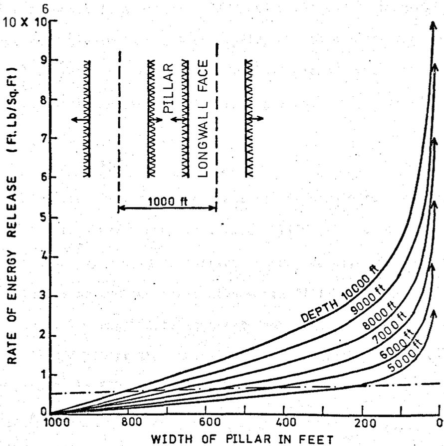
Fig. 2.8.3. The relationship between pillar size (formed by the approaching of two longwall faces) at different depths and the rate of energy release. The broken line represents the rate of non-violent energy dissipation. (After Cook et al., 1966).
