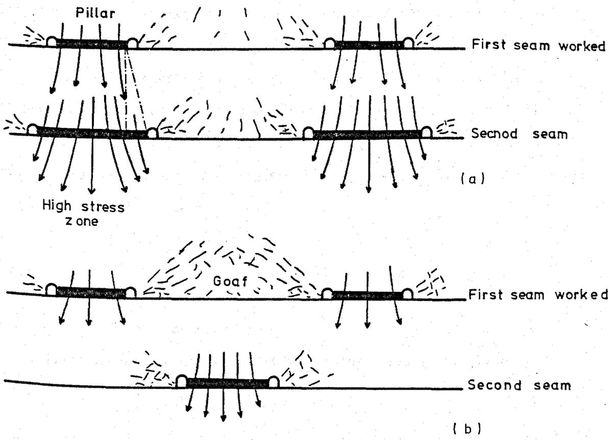
Fig. 2.5.1. Composite layout of longwall workings showing the best position of the current mine workings (2nd seam) with respect to old mine workings in an adjacent seam.
