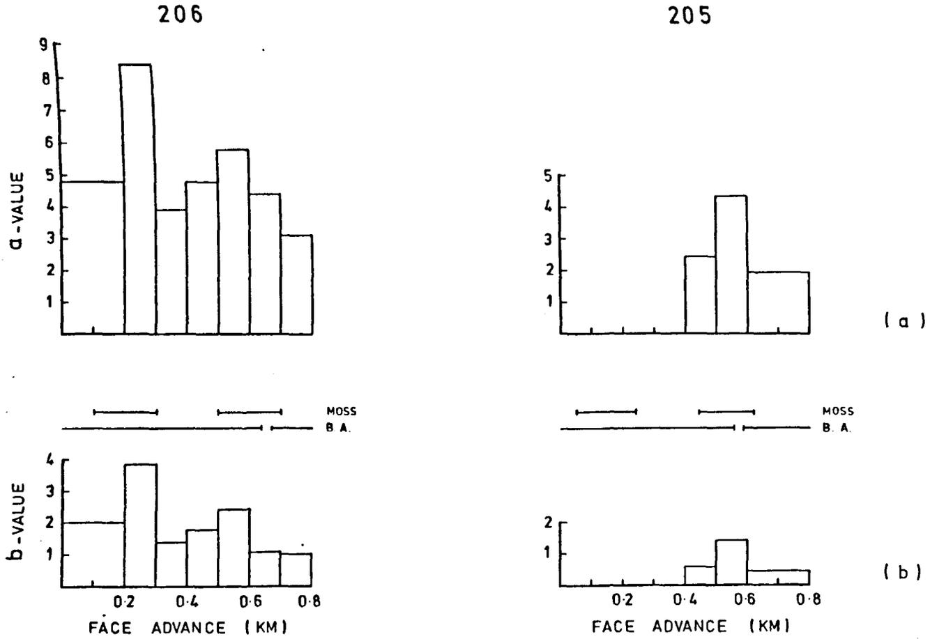
Figure 7.4.2. Histograms of (a) a-value and (b) b-value for each 100 m or 200 m of face advance, for tremors occurring during the mining of panels 205 and 206. The regions where the Ten Feet face lies above or below the Moss and Bowling Alley (B.A.) seams are also shown.
