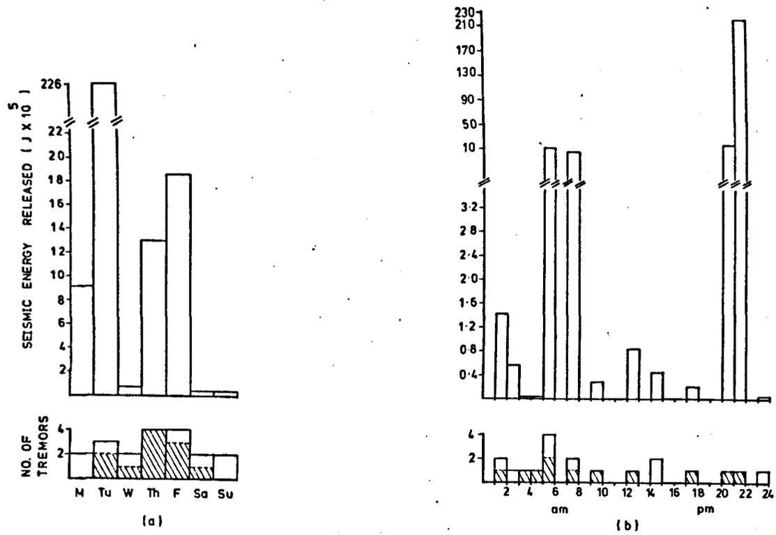
Fig. 9.3.11. Histograms showing (a) the weekly and (b) the daily distribution of tremors and the corresponding seismic energy release for tremors which occurred in area A. The shaded area represents tremors having a shear source mechanism.
