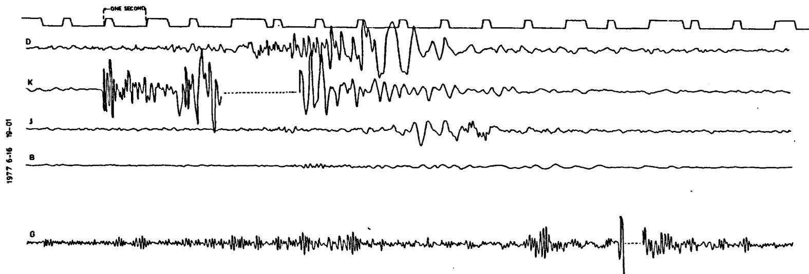
Fig. 4.10.4. Seismogram of fourth type of tremor recorded at 1977 6-16 19-01. Two prominent downward peaks can be seen in seismometer K and probably in seismometer G also, while in the other seismometers the highest amplitude seismic waves preceded by low amplitude waves. These most probably represent seismic waves produced by sonic booms from jet aircraft.
