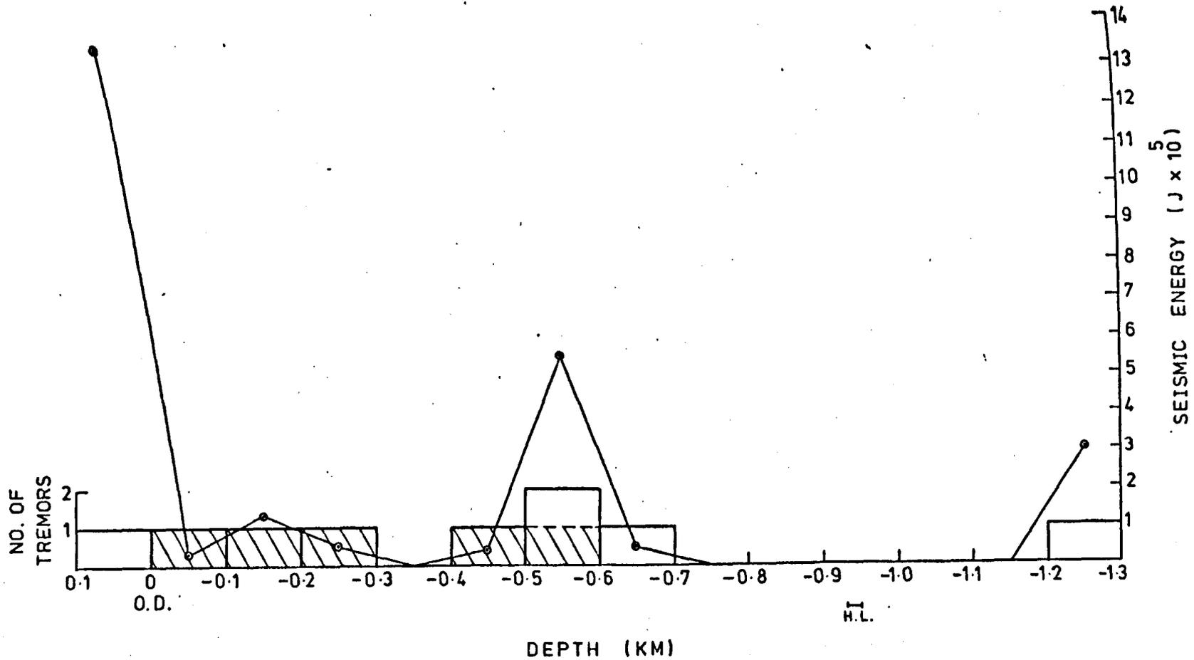
Fig. 9.4.4. A plot showing the number of tremors and the corresponding seismic energy release, occurring within each 100 m depth interval in area B. The depth ranges of the active mine workings in the Holly Lane (H.L.) seam is also shown. The shaded area represents tremors with a shear source origin.
