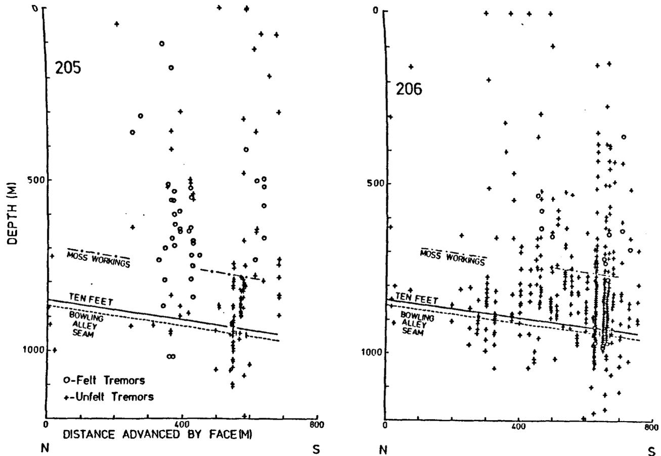
Fig. 7.2.4. Plot of the vertical position of tremor foci against distance advanced by the face for tremors occurring during the mining of panels 205 and 206. The position of the Ten Feet seam workings and previous workings in the Moss and Bowling Alley seams are also shown. (Taken from Kuszniir et al., 1980a).
