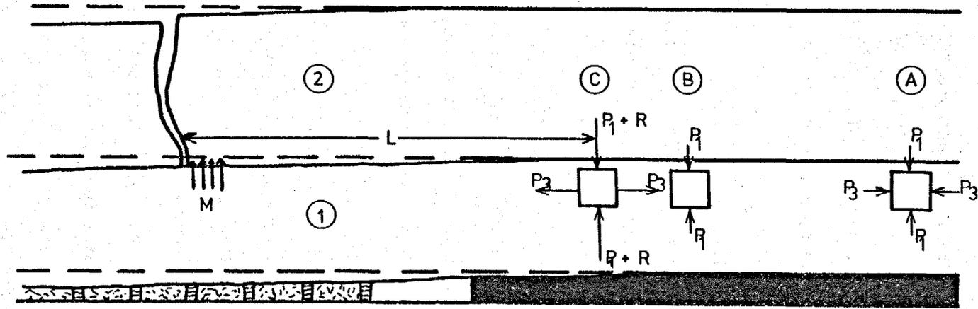
Fig. 2.6.1. Vertical section through coal face and goaf, illustrating the action of strata pressure in three different places (A, B and C) in front of the coal face. (After Hudspeth and Phillips, 1932-33).
