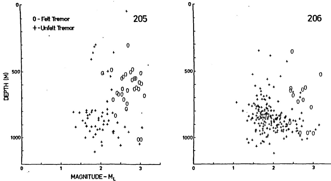
Fig. 7.2.5. The tremor depth plotted against local magnitude,  $M_L$ , for tremors occurring during the mining of panels 205 and 206. (Taken from Kusznir et al., 1980a).
