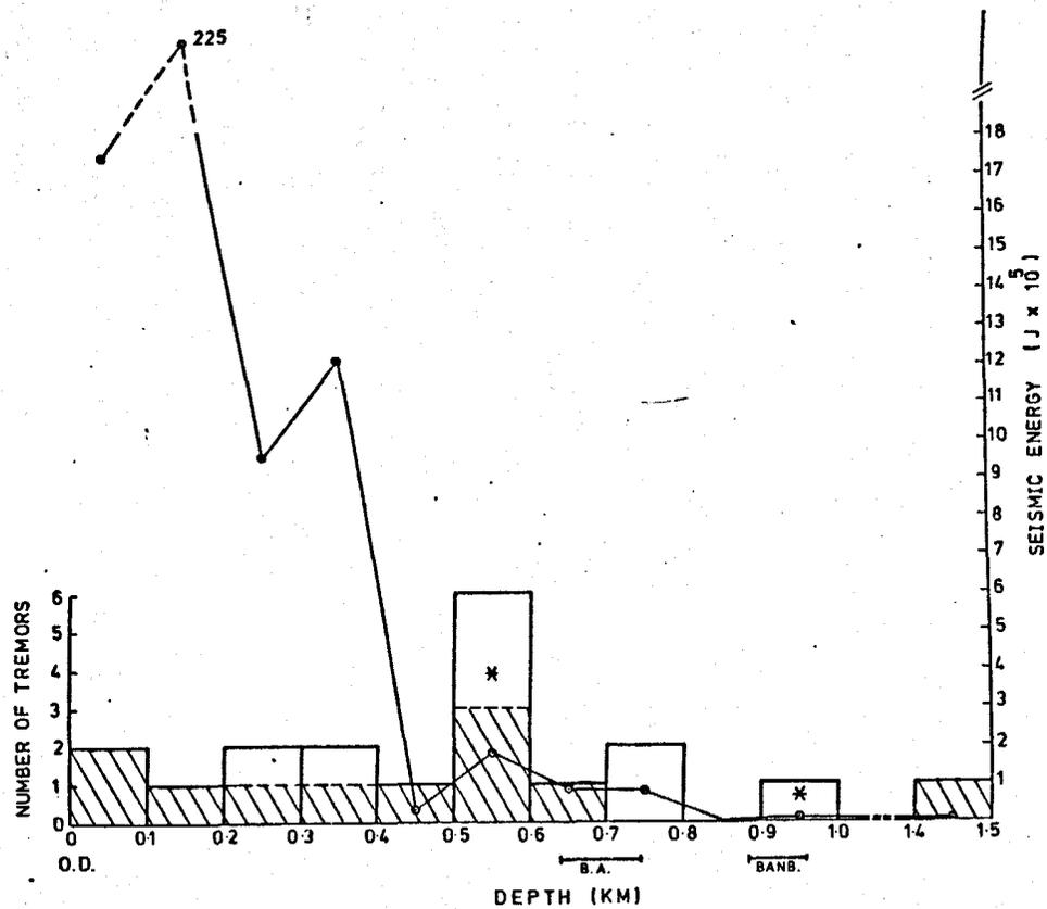
Fig. 9.3.4. A plot showing the number of earth tremors and the corresponding seismic energy release, occurring within each 100 m depth interval in area A. The depth ranges of the active mine workings in the Bowling Alley (BA) and Banbury (BANB) seams are also shown. The shaded area represents tremors having a shear source mechanism.
