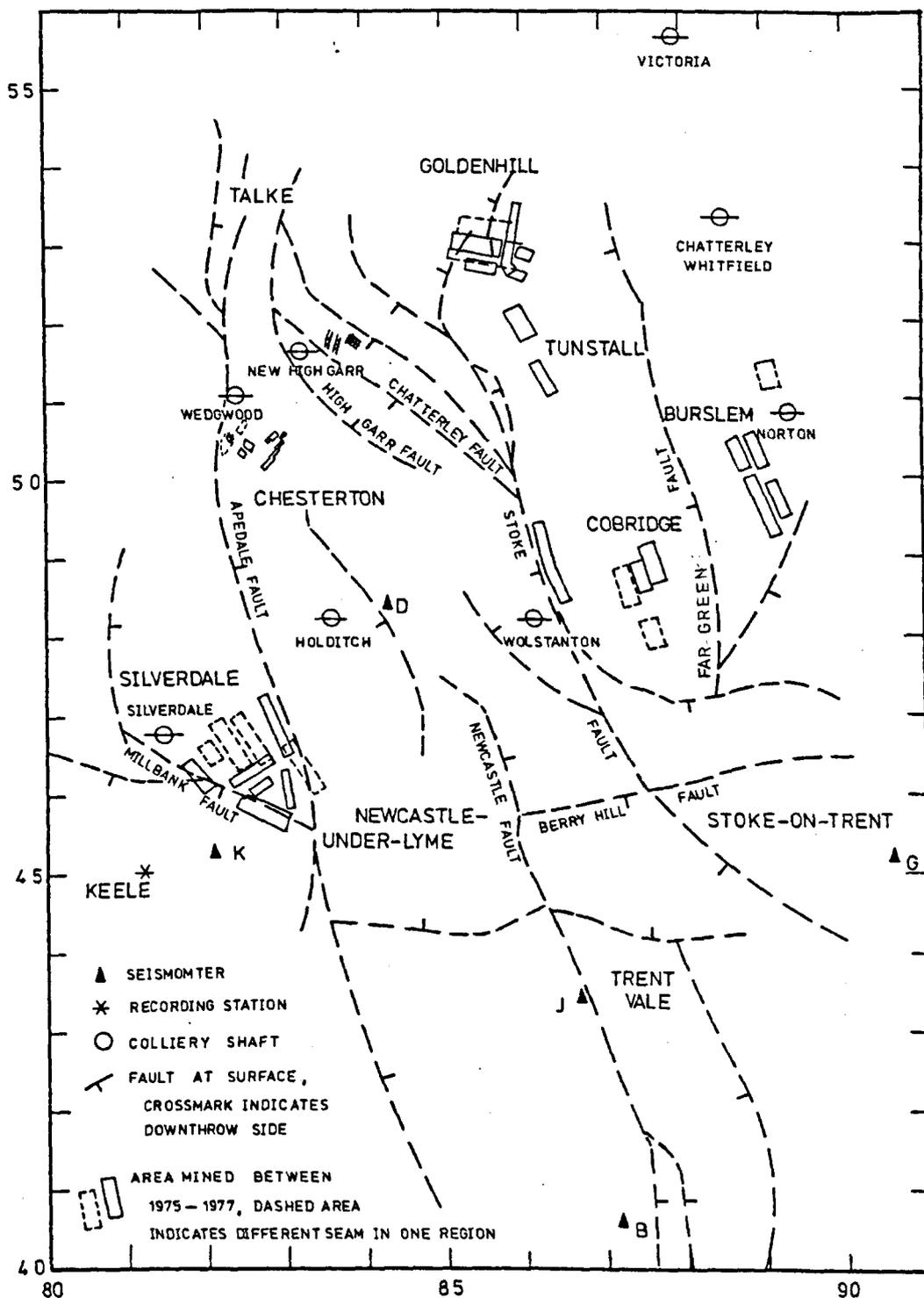
Fig. 4.2.1. Map showing the positions of the active mine workings, major surface faults, seismometer sites, seismic recording station and the colliery shafts in the northern part of the North Staffordshire Coalfield.
