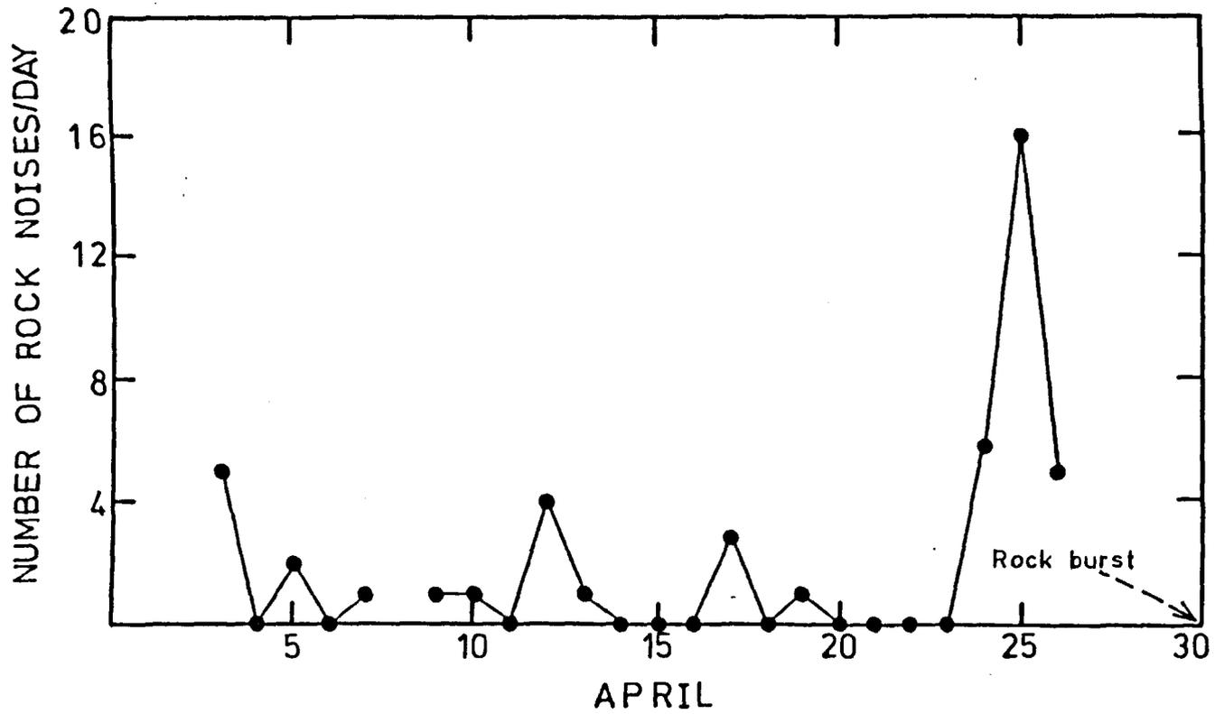
Fig. 3.5.2. Development of rock noise rate associated with the rock burst shown in Fig. 3.5.1. (After Leighton and Steblay, 1977).
