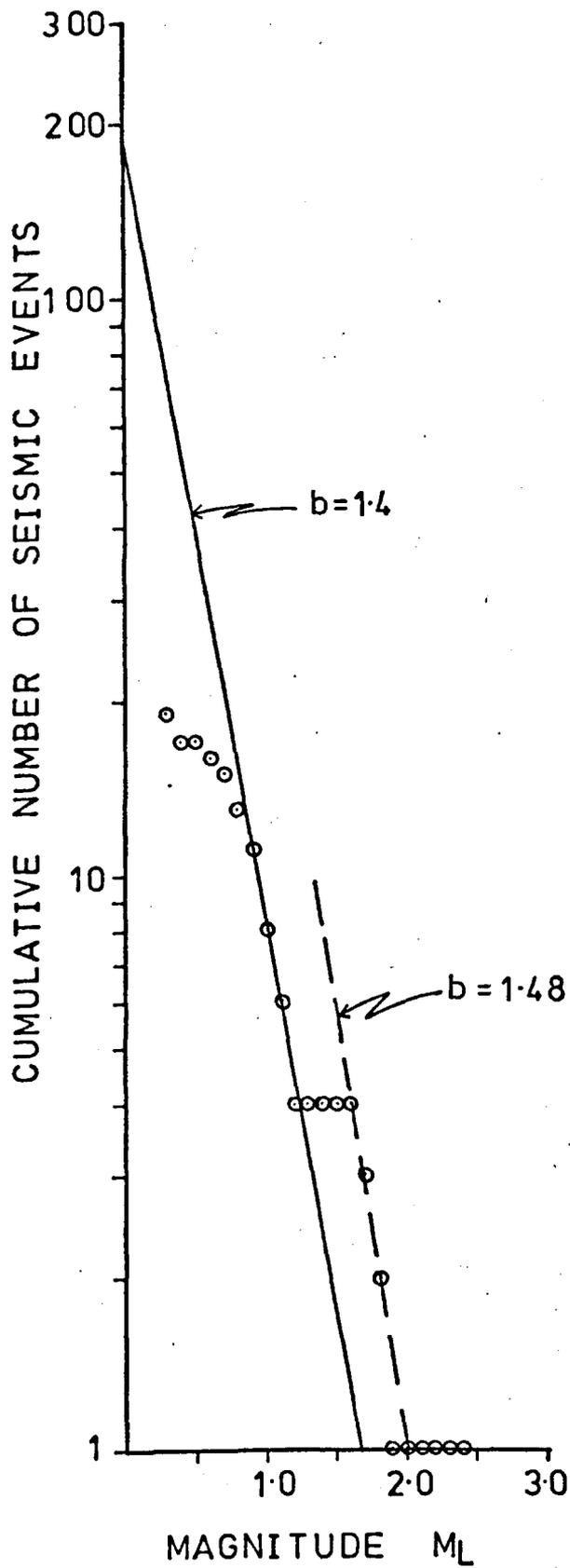
Fig. 9.3.13. A plot showing the frequency-magnitude distribution for tremors occurring in area A.
