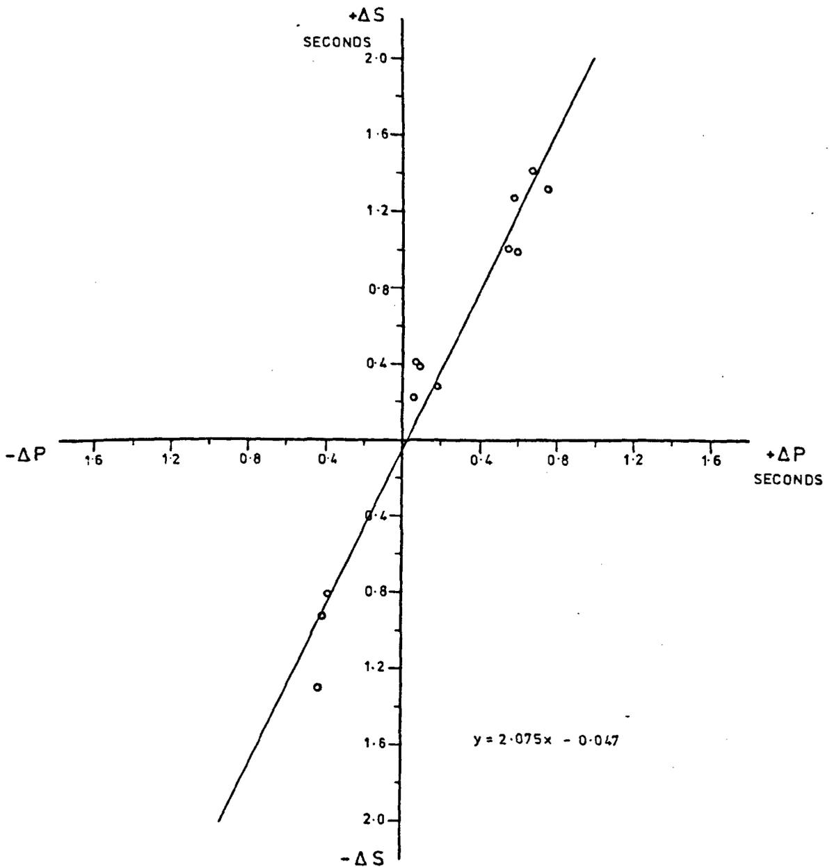
Fig. 4.6.1. Plot of S-arrival time difference ( $\Delta S$ ) against P-arrival time difference ( $\Delta P$ ). The straight line indicates that the ratio between P and S velocities is 2.075.
