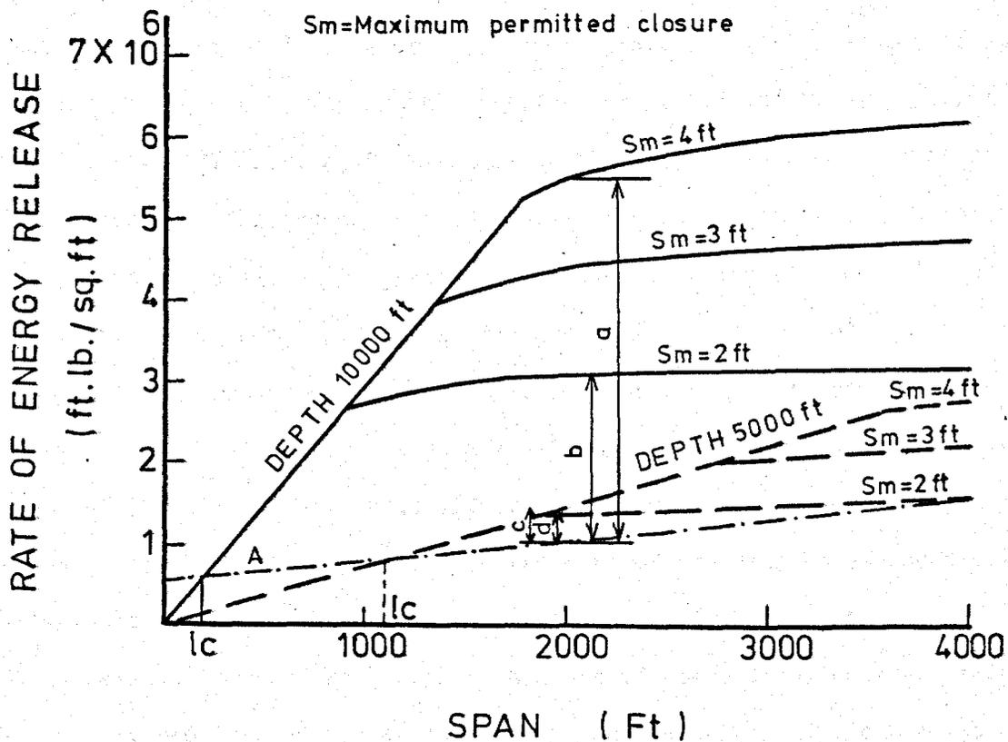
Fig. 2.8.2. The relationship between the rate of energy release and the span of a longwall stope, in which maximum closure is limited to 2, 3 and 4 ft., at two different depths. Line A represents the rate at which energy is dissipated non-violently. The difference in length between lines a and b, and c and d represents the difference in the energy release due to the effects of 2 ft. waste filling in a 4 ft. high stope. (After Cook et al., 1966).
