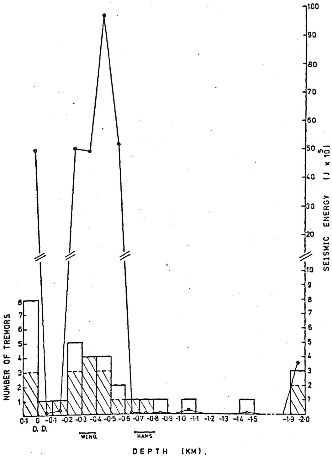
Fig. 9.5.4. A plot showing the number of tremors and the corresponding seismic energy release, occurring within each 100 m depth interval in area C. The depth ranges of the active mine workings in the Winghay (WING) and Hams seams are also marked. The shaded area represents tremors with a shear source origin.
