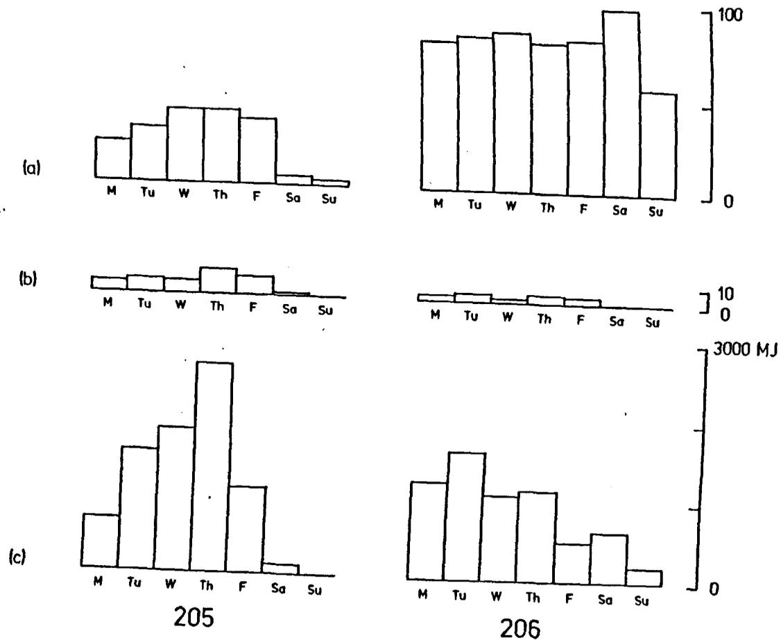
Fig. 7.2.6. The distribution throughout the week of (a) the total number of tremors, (b) the number of felt tremors, and (c) the total seismic energy released for panels 205 and 206. (Taken from Kuznir et al., 1980a).
