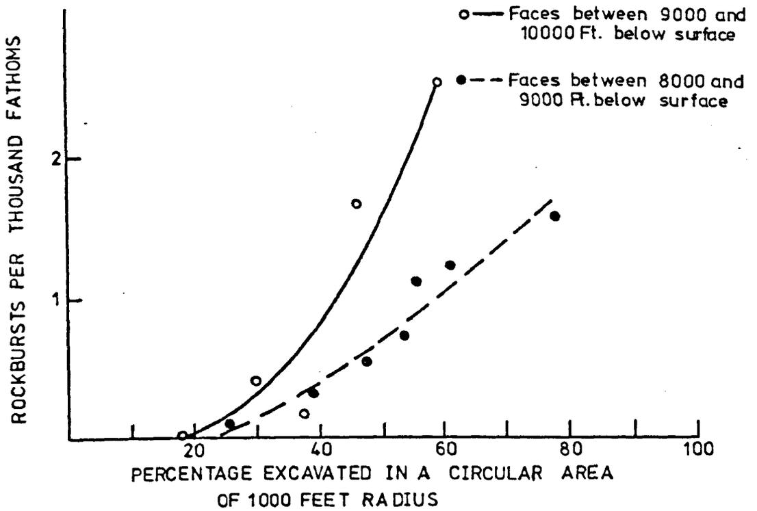
Fig. 3.4.3. The relationship between rock burst incidence and the relative excavation size at different depths in the Witwatersrand gold mines. (After Cook et al., 1966).
