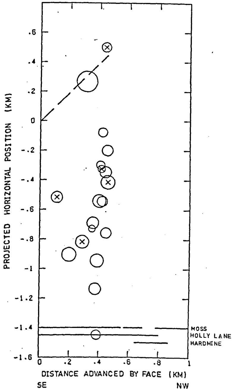
Fig. 9.6.8. Plot of the horizontal position of tremor epicentres projected onto the line of face advance and measured from the start of the panel, against distance advanced by the face for tremors occurring during the mining of panel 57 in area D. The diagonal dashed line corresponds to the line on which tremors would plot if they occurred on the face 57. The regions where the face 57 lies below previous Moss or above Holly Lane and Hardmine seam workings are also shown.
