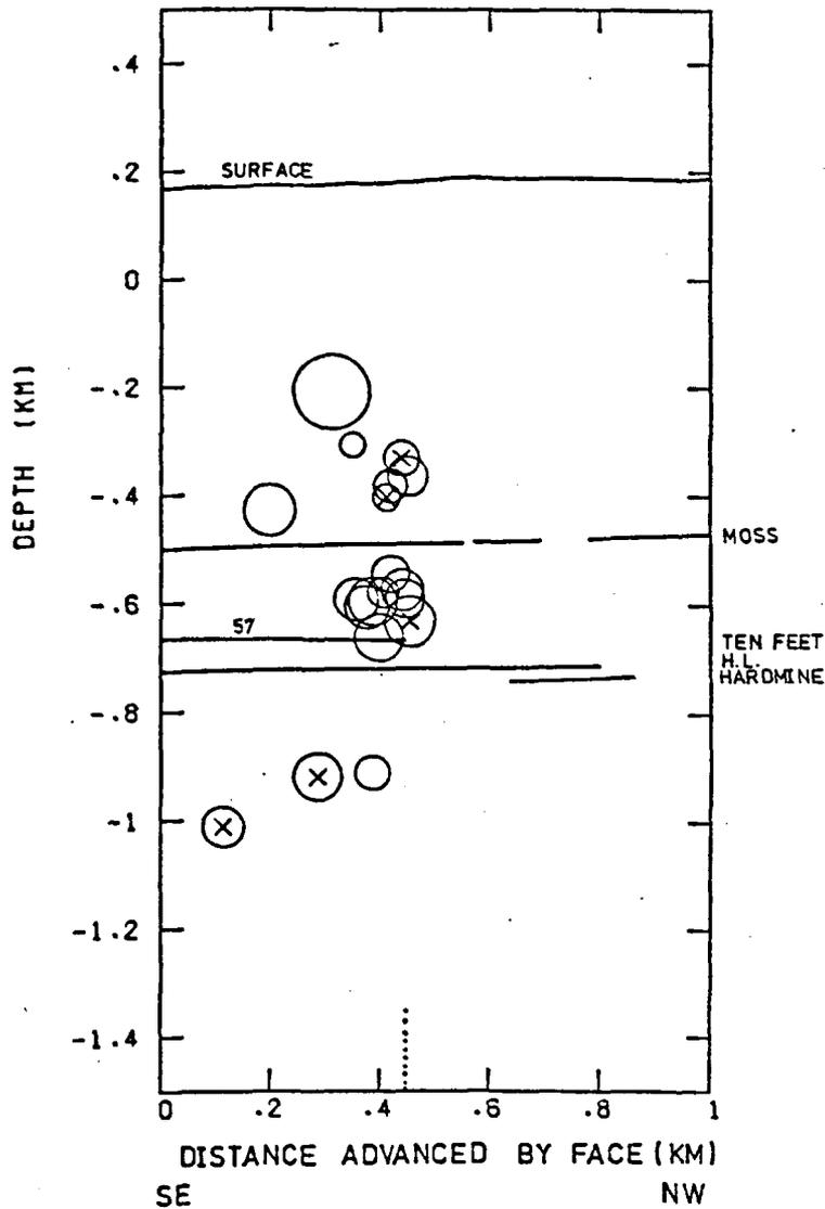
Figure 9.6.10. Plot of tremor depth against the distance advanced by the face for tremors occurring during the mining of panel 57 in area D. The position of mine workings in panel 57 of the Ten Feet seam and previous workings in the Moss, Holly Lane (H.L.) and Hard mine seams are also shown.
