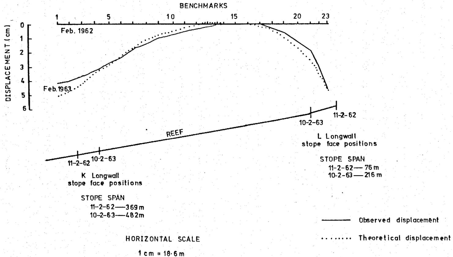
Fig. 2.7.3. Comparison between observed and calculated elastic theory displacements, along tunnel 58 in the vicinity of the K and L longwall stopes (Witwatersrand), relative to benchmark 15 from February 1962 to February 1963. (After Ryder and Officer, 1964).
