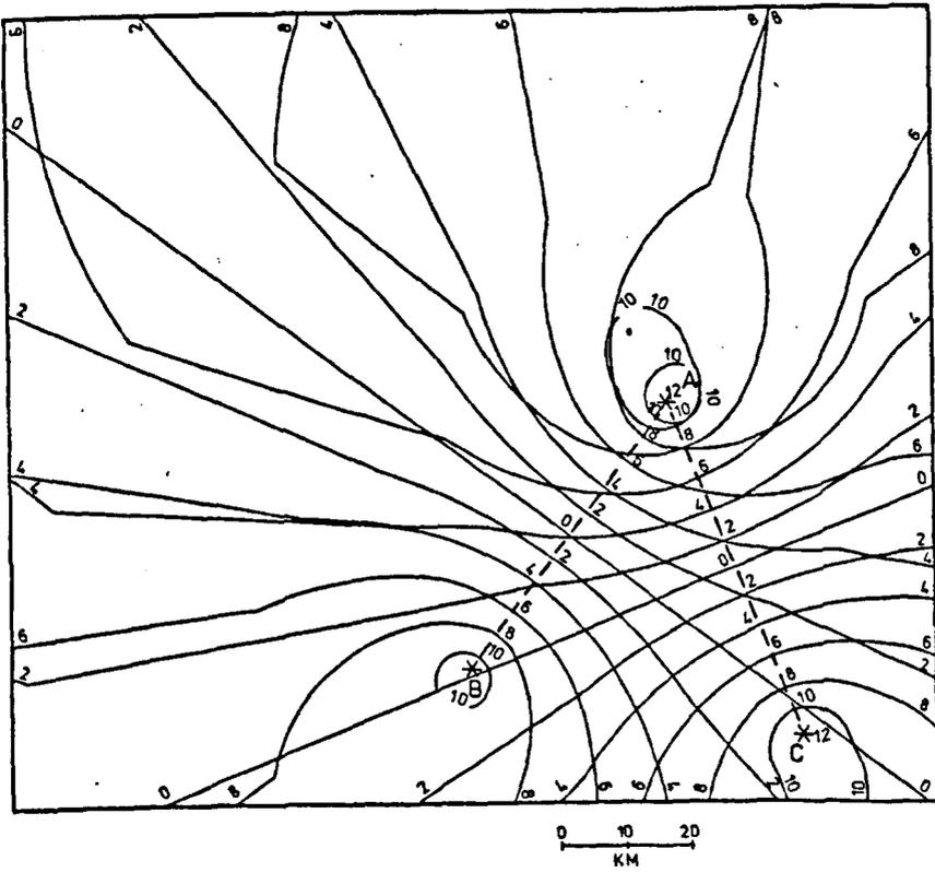
Fig. 4.7.1. Two time-difference charts obtained from two pairs of stations (stations A and B, and A and C) superimposed on each other illustrating epicentre location technique. (After Browitt, 1977).
