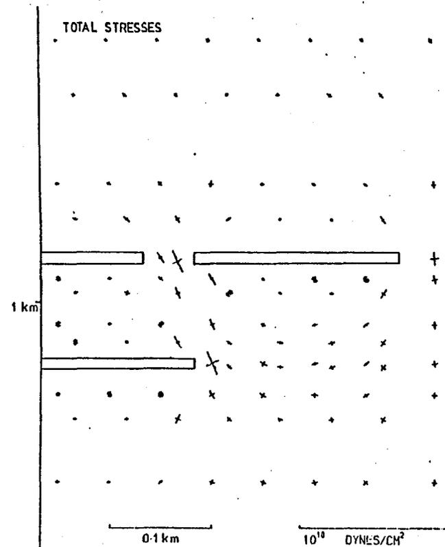
Fig. 7.4.9. Stresses induced by a 300 m length panel advancing beneath a 50 m wide pillar. (After Beale, 1981).
