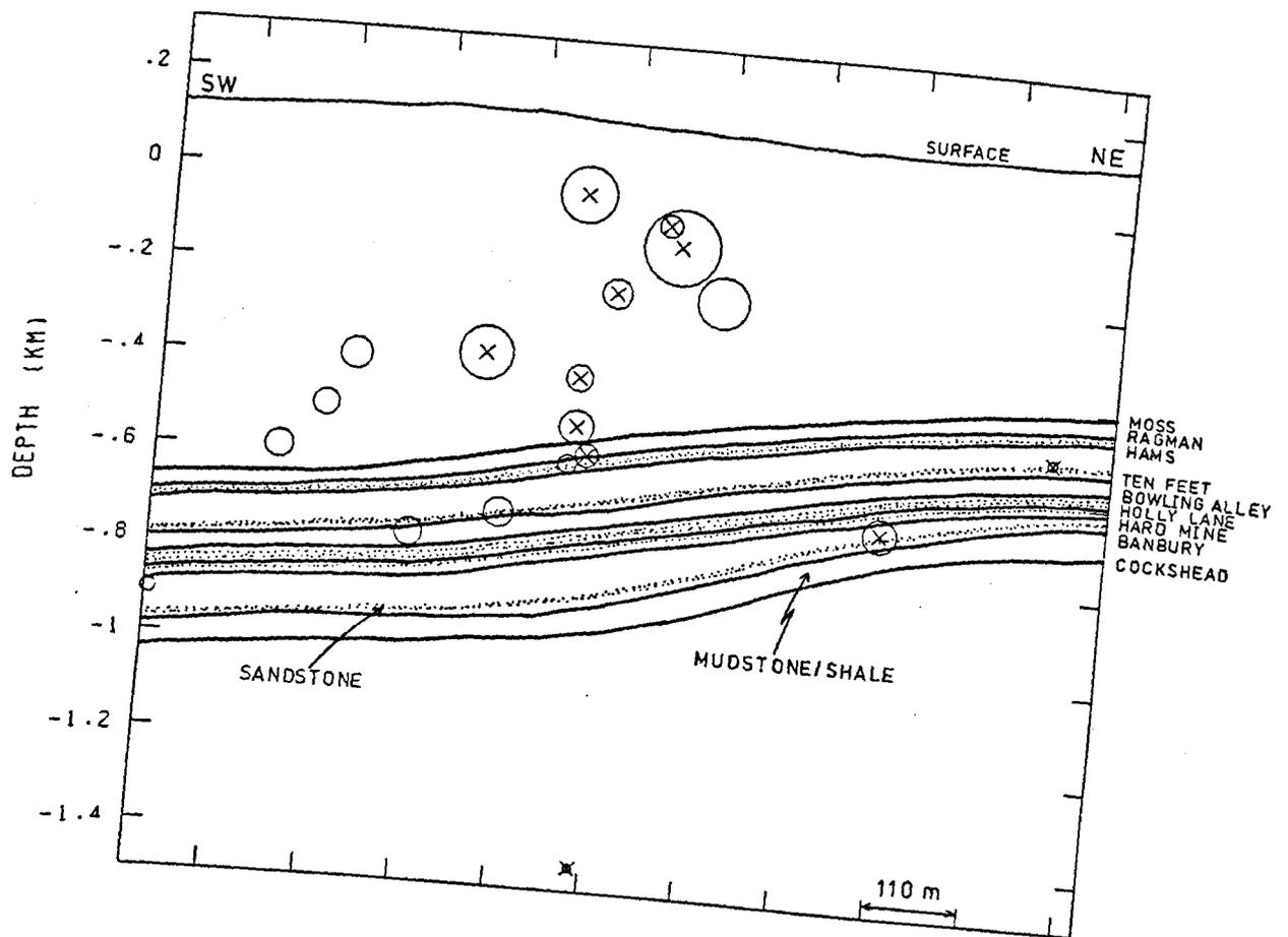
Fig. 9.3.6. Geological section drawn downdip showing the positions of tremor foci for tremors occurring in area A.
