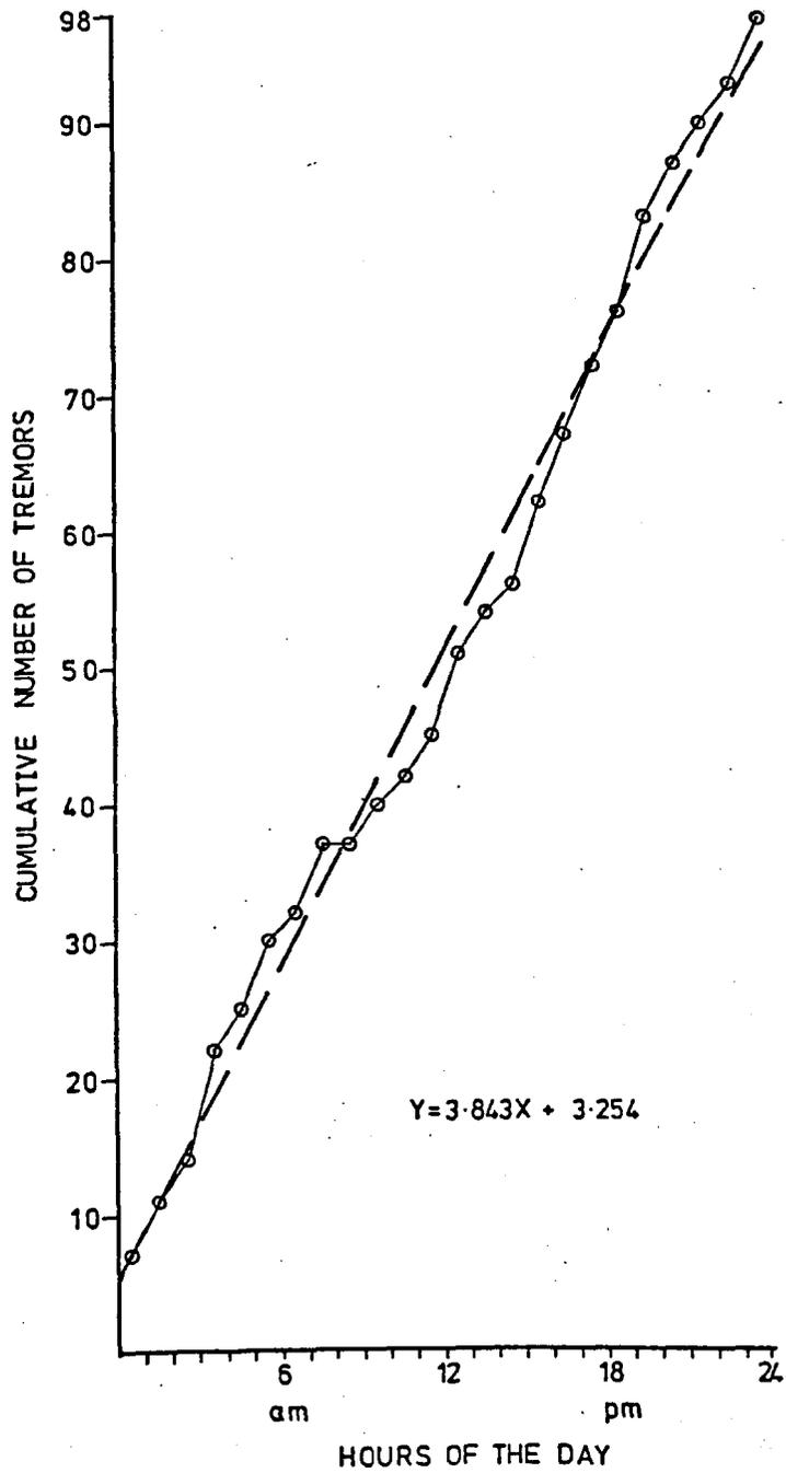
Fig. 8.3.9. Plot of the cumulative number of tremors against hours of the day for tremors which occurred in the northern part of the North Staffordshire Coalfield. The diagonal dashed line corresponds to the line on which the total number of tremors would plot if the tremor occurrence was uniform throughout the day.
