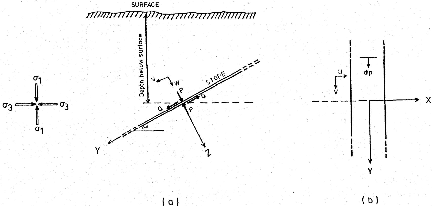
Fig. 2.7.2. Induced components of movements in the solid rocks as a result of the action of lithostatic stresses on a dipping stope.
