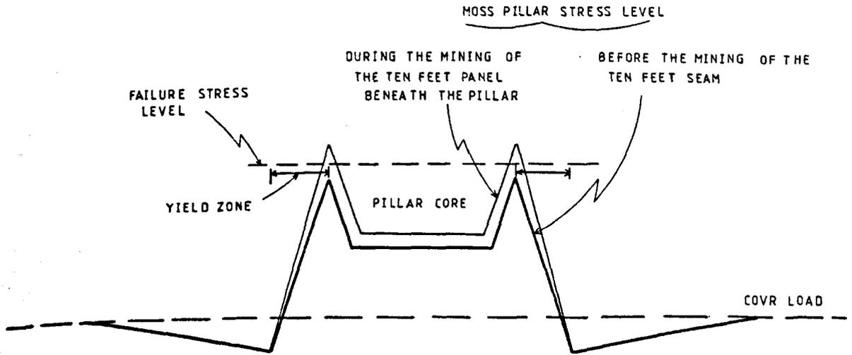
Fig. 7.4.10. Changing of the vertical stress level in the Moss pillar due to the mining of the Ten Feet panel beneath it.
