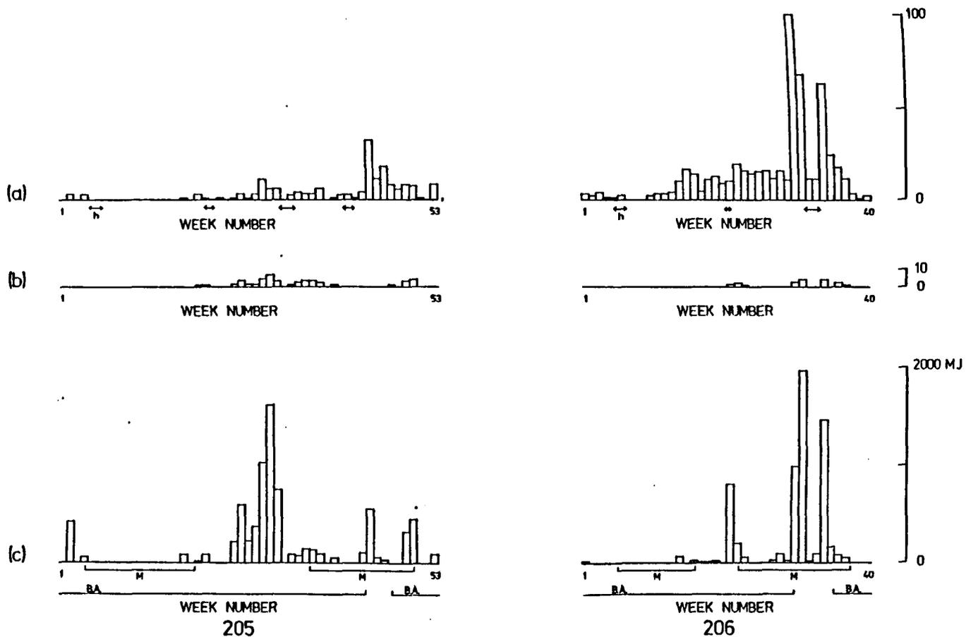
Fig. 7.2.7. Histograms of (a) the total number of tremors per week, (b) the number of felt tremors and (c) the total seismic energy release for panels 205 and 206. The periods during which the Ten Feet face was passing under or over previously extracted Moss seam (M) and Bowling Alley seam (BA) are shown. Miners' holidays are also indicated (h). (Taken from Kuszniir et al., 1980a).
