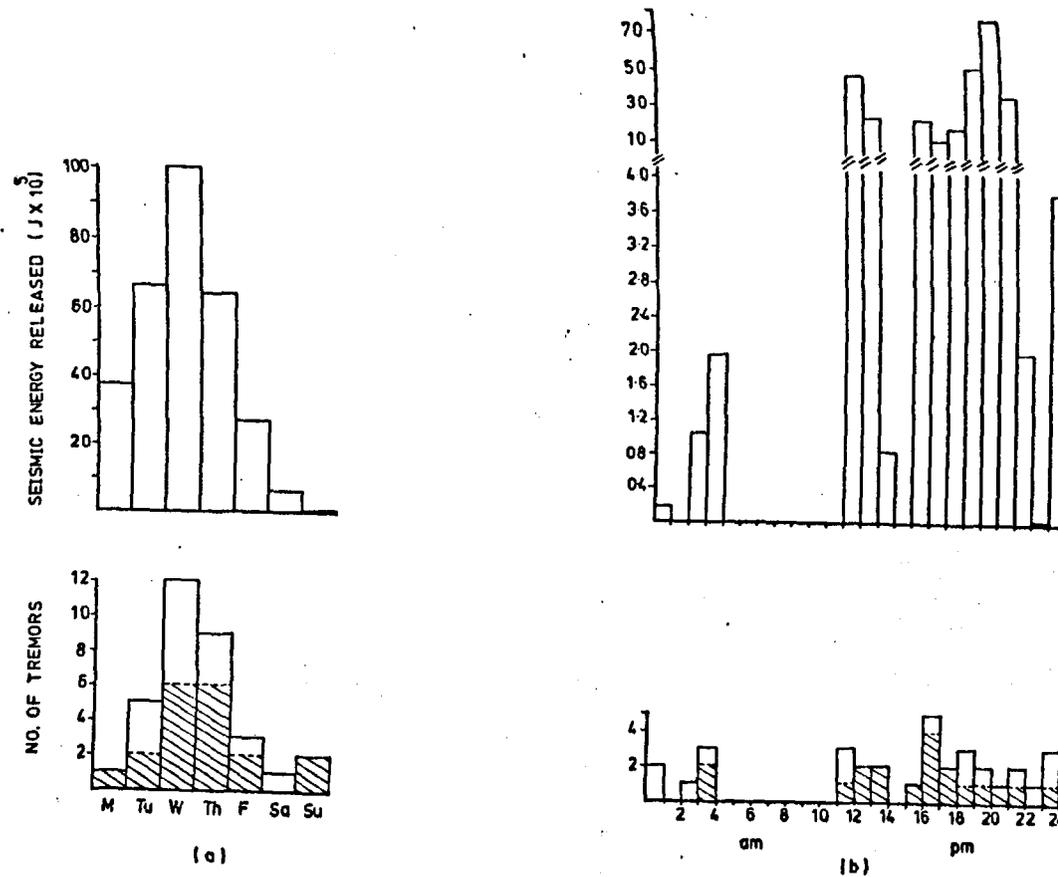
Fig. 9.5.7. Histograms showing (a) the weekly and (b) the daily distribution of tremors and the corresponding seismic energy release for tremors which occurred in area C. The shaded area represents tremors with a shear source mechanism.
