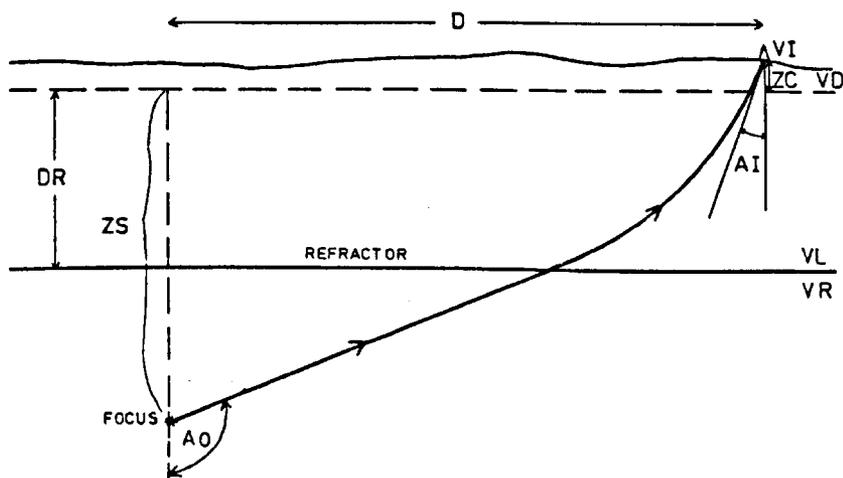
Fig. A-4: Seismic structure model with linear increase of seismic velocity with depth which is underlain by a constant higher velocity layer (refractor). The tremor focus lies below the refractor.
