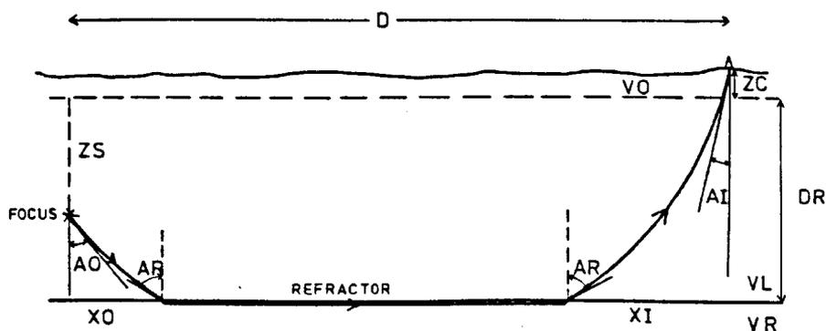
Fig. A-3: Seismic structure model with linear increase of seismic velocity with depth which is underlain by a constant higher velocity layer (refractor). The tremor focus lies above the refractor.
