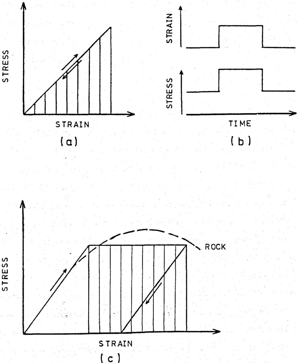
Fig. 2.8.1. (a) Stress-strain curve showing the strain energy resulting from the deformation of an elastic material.
