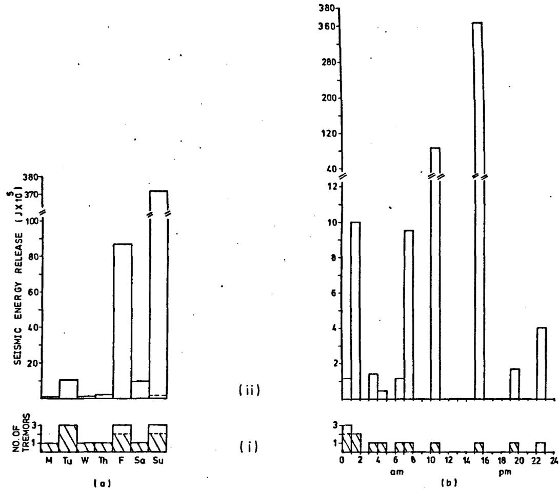
Fig. 9.7.6. Histograms showing (a) the weekly and (b) the daily distribution of tremors and the corresponding seismic energy release for tremors which occurred in area E. The shaded area represents tremors with a shear source mechanism. The dashed line in Fig.a (ii) represents the amount of energy release on Sundays if the seismic energy released by event 1976 10-31 15-47 is subtracted.
