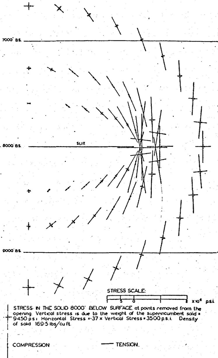
Fig. 2.7.1. The magnitudes and directions of the principal stresses along one half of a horizontal slit in an elastic body subject to gravity. (After Cook, 1962).
