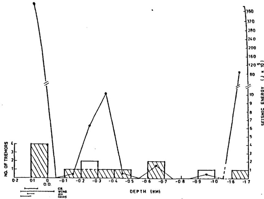
Fig. 9.7.4. A plot showing the number of tremors and the corresponding seismic energy release occurring within each 100 m depth interval in area E. The depth ranges of the active mine workings in the Cannel Row (CR), Winghay (WING), Rowhurst (RH) and Hams seams are also shown. The shaded area represents tremors with a shear source origin.
