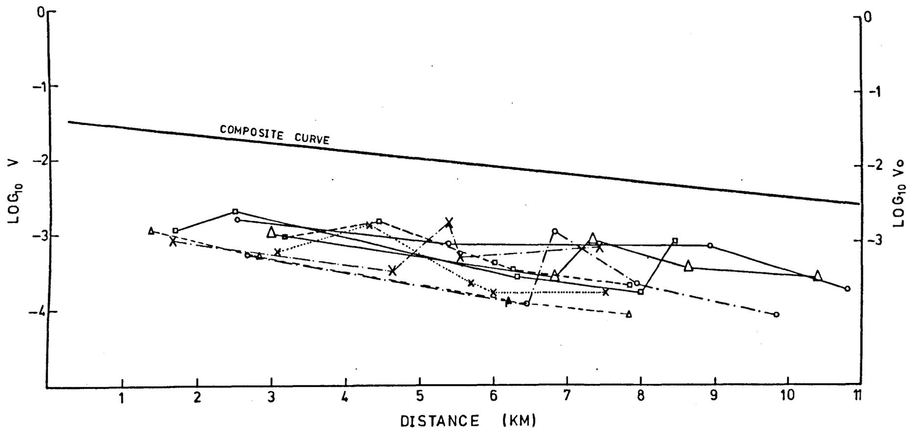
Fig. 4.9.1. Plot of logarithm amplitude ( $\log_{10} V_0$ ) of the standard earth tremors against distance, showing the attenuation of the ground velocity in the North Staffordshire Coalfield (labelled composite curve). The figure was obtained by plotting the logarithm of maximum trace amplitude of ground velocity against its epicentral distance, for a number of seismic events. The curves were then combined into a single composite curve passing through a point chosen as the standard shock.
