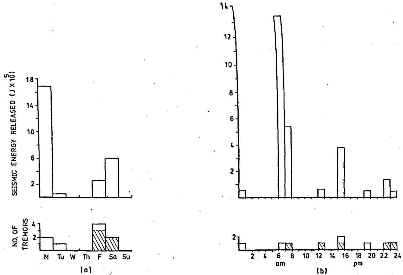
Fig. 9.4.6. Histograms showing (a) the weekly and (b) the daily distribution of tremors and the corresponding seismic energy release for tremors which occurred in area B. The shaded area represents tremors with a shear source mechanism.
