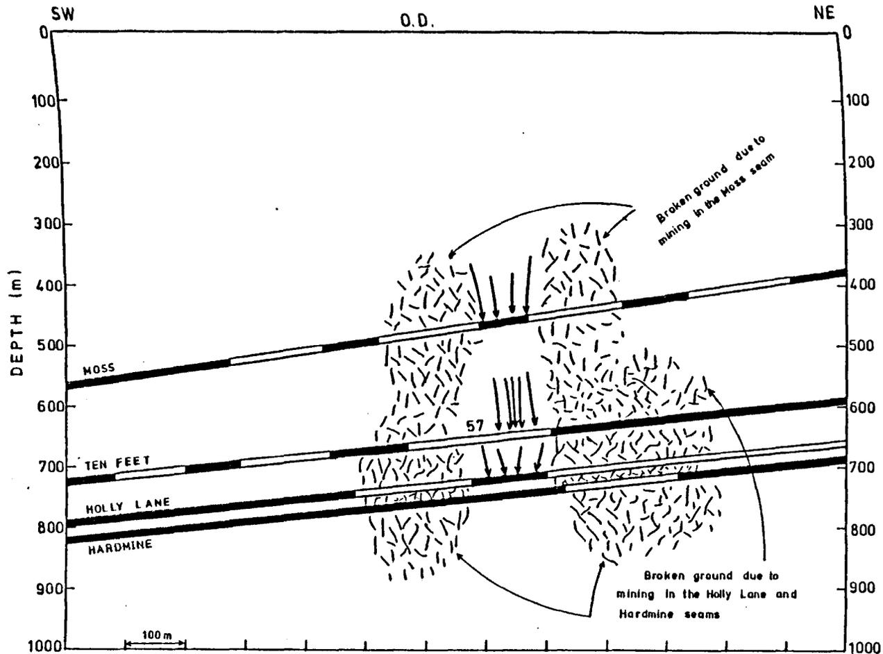
Fig. 9.6.14. Diagrammatic section parallel to face 57 of the Ten Feet seam in area D showing the distribution of stresses around the panel face due to the presence of pillars in previous mine workings above and below the panel, in the Moss, Holly Lane and Hard mine seams. The stress is concentrated on pillars while the broken ground above and below the extracted region is de-stressed.
