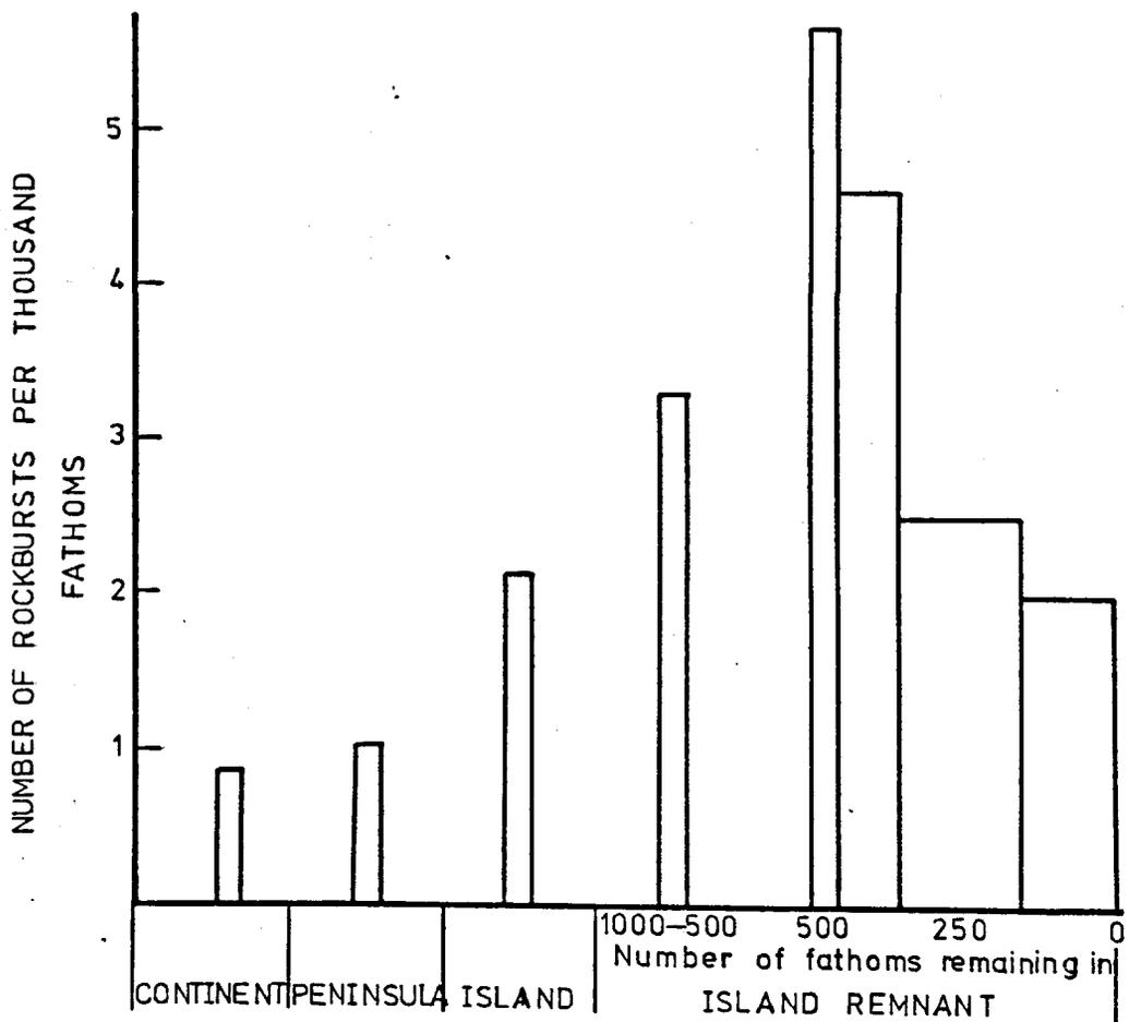
Fig. 3.4.1. The variation in rock burst incidence for various abutment types. Also shown is the influence of the size of abutment on rock burst incidence, in the case of island remnant. (After Pretorius, 1964).
