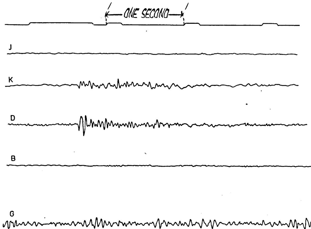
Fig. 4.10.1. Seismogram of first type of tremor recorded at 1977 6-6 06-23. Low amplitude and short duration of seismic waves probably indicate tremors which originate near the detection site. Letters designate seismometer names.
