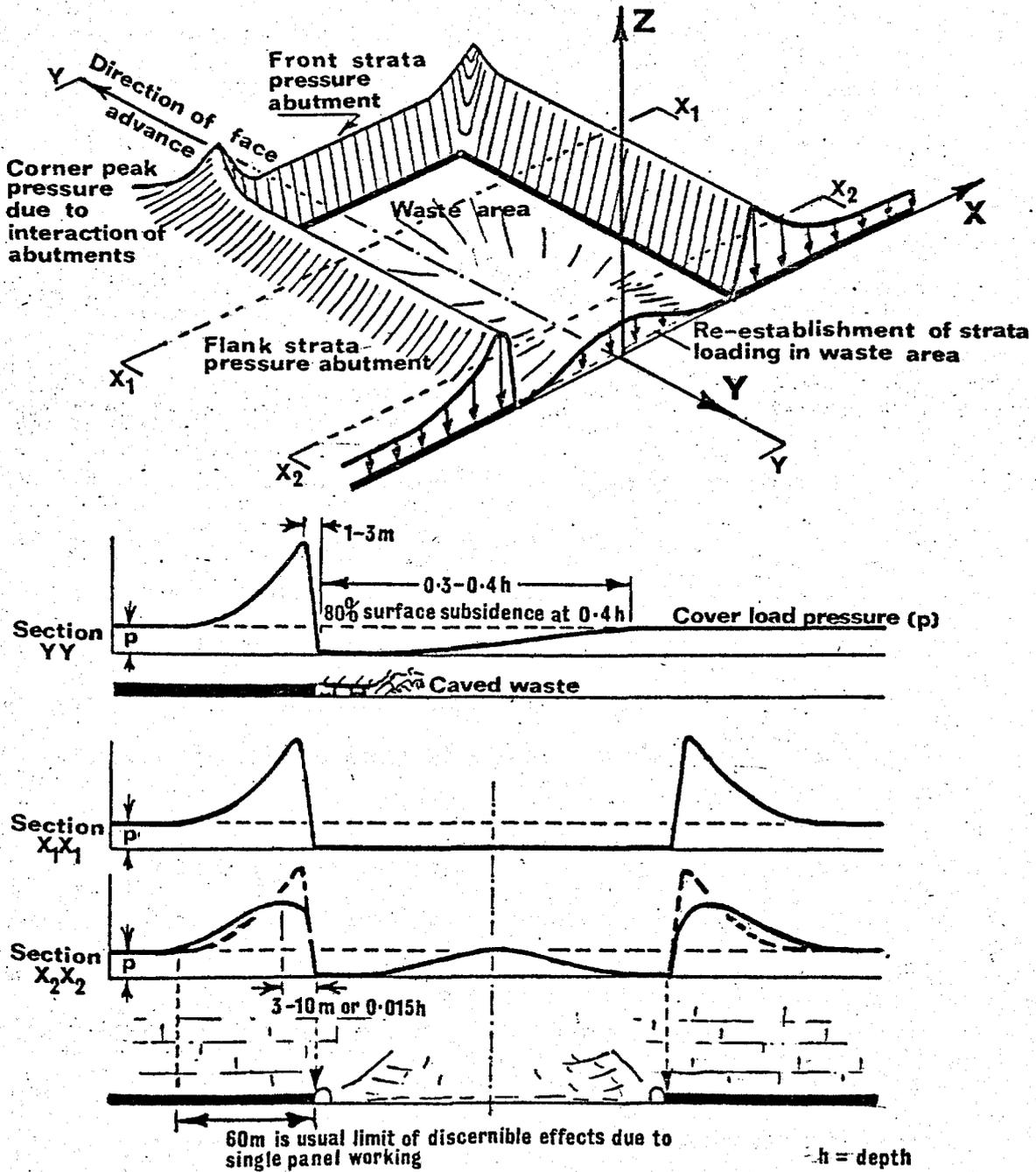
Fig. 2.3.3. Stress distribution around a longwall face. (After Whittaker, 1974).
