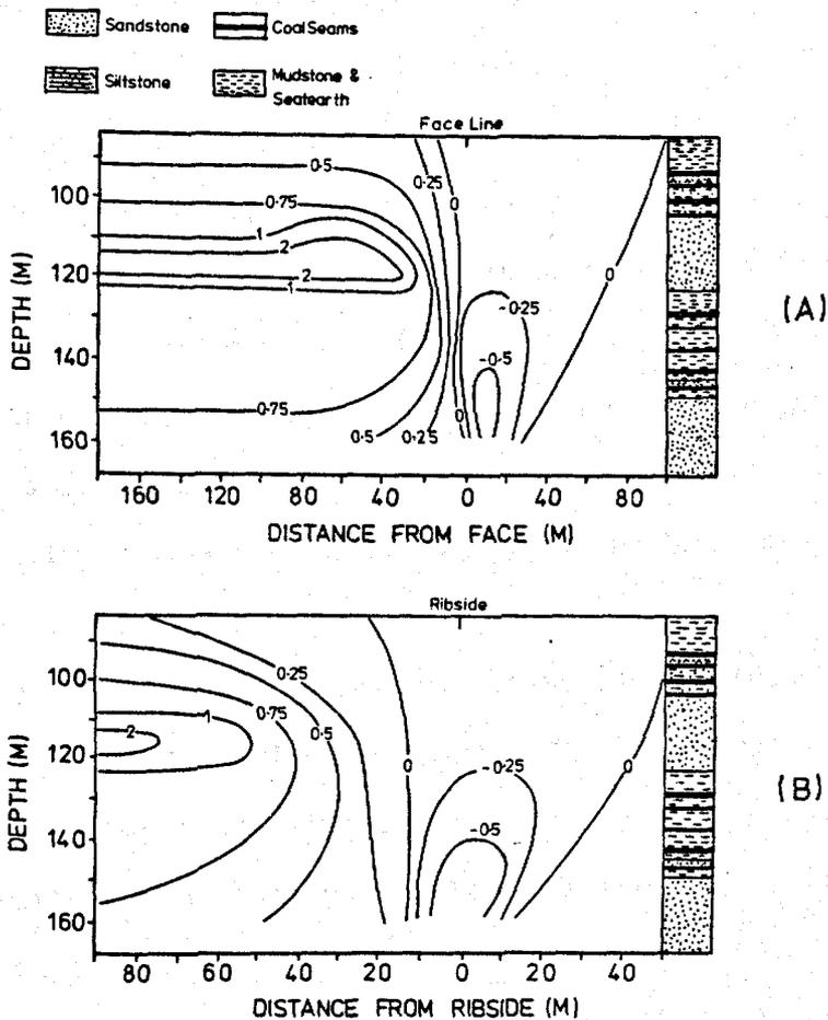
Fig. 2.4.1. Vertical strain contours above a longwall face.
