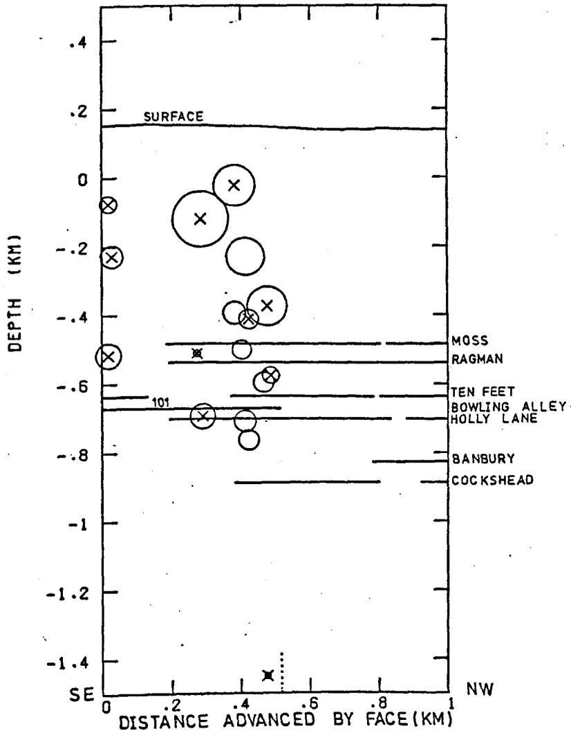
Fig. 9.3.9. Plot of tremor depth against the distance advanced by the face for tremors occurring during the mining of panel 101 in area A. The position of mine workings in panel 101 of the Bowling Alley seam and previous workings in different adjacent seams are also shown.
