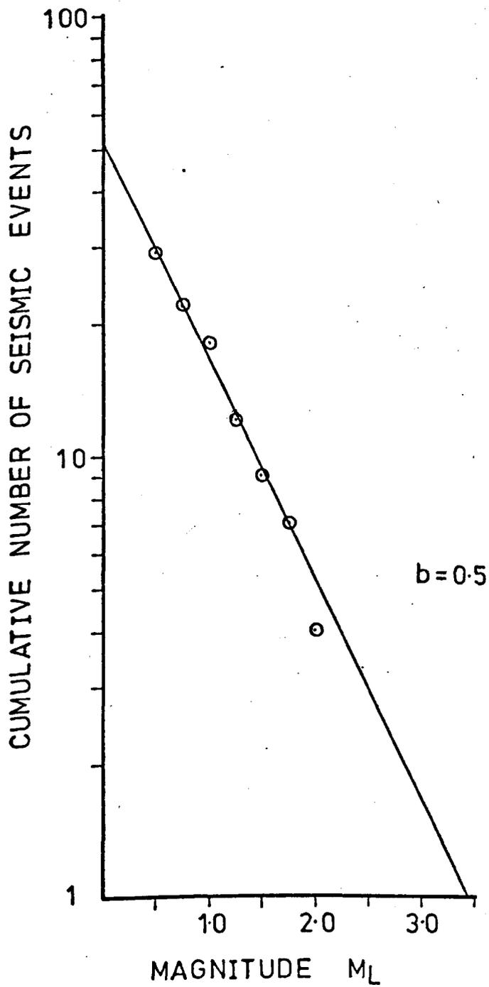
Fig. 9.5.9. A plot showing the frequency-magnitude distribution for tremors occurring in area C.
