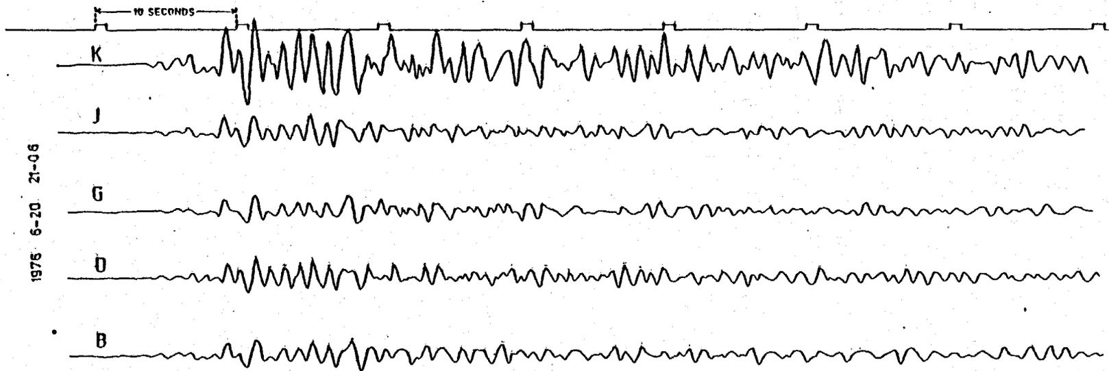
Fig. 4.10.3. Seismogram of third type of tremor recorded at 1976 6-20 21-06. Very low frequency, high amplitude and long duration of seismic waves represent regional or teleseismic events.
