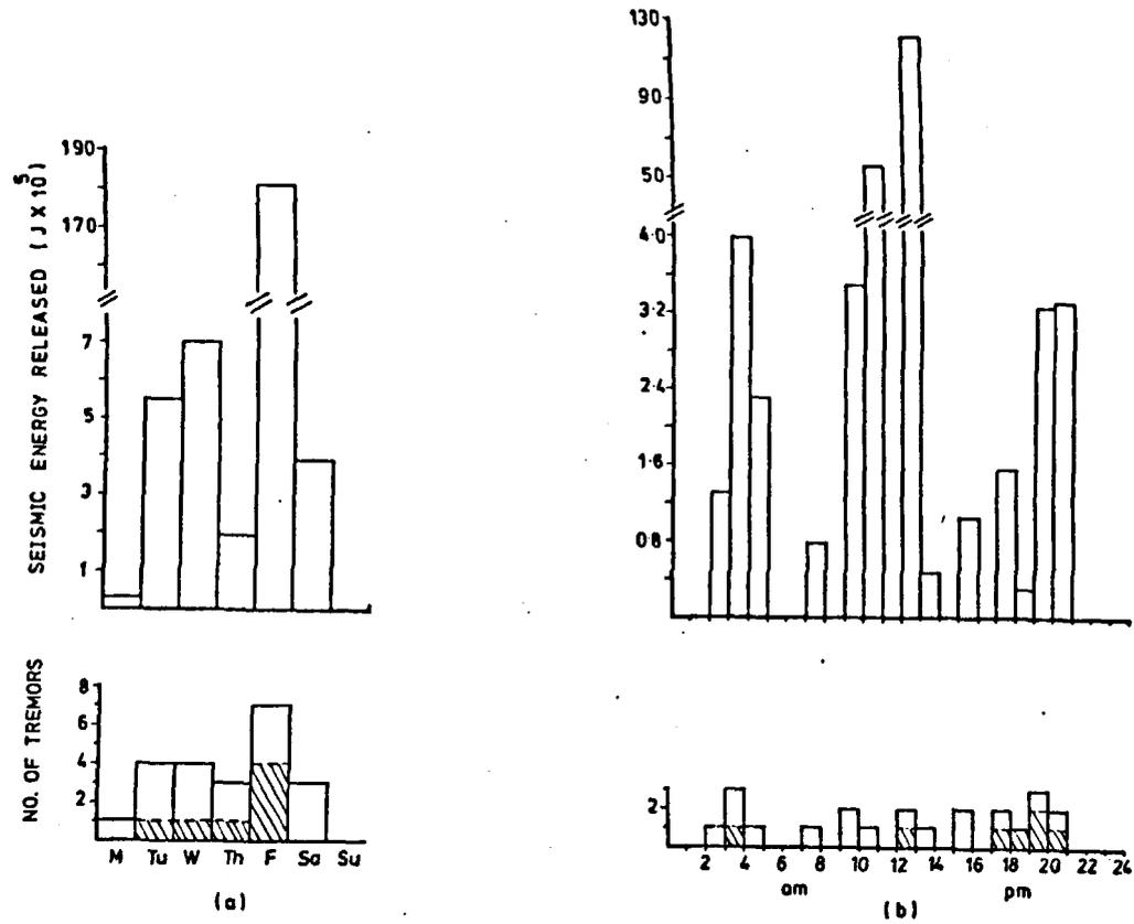
Fig. 9.6.11. Histograms showing (a) the weekly and (b) the daily distribution of tremors and the corresponding seismic energy release for tremors which occurred in area D. The shaded area represents tremors with a shear source mechanism.
