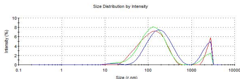
Figure 65: Photon correlation spectroscopy size correlation charts for unfiltered solutions of carrier 46f with concentrations 0.1 mg/mL (A), 1 mg/mL (B) and 5 mg/mL (C) in deionised water (n=3).
