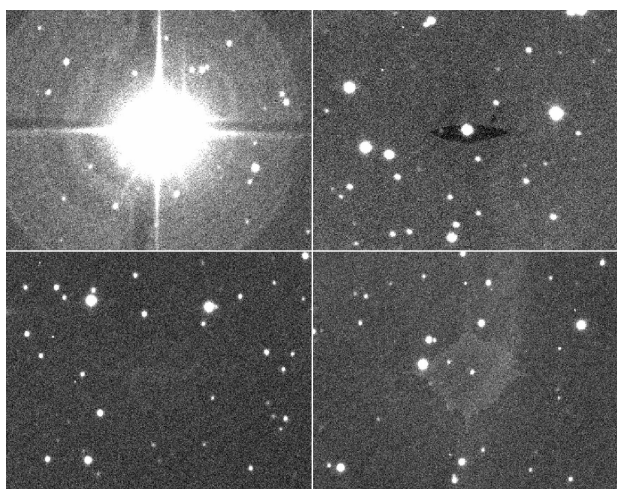
Fig. A.9. Cross talk on image r1023036. CCD#1 is shown top left, #2 top right, #3 bottom left and #4 bottom right. The same pixel section is shown for each CCD. The bright star on CCD#1 is seen as a negative imprint on #2 for pixels that are saturated, as a positive imprint on #4 and a faint positive imprint on #3.
